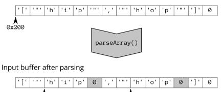
Adding null-terminators is not the only thing the parser modifies in the input buffer. It also replaces escaped character sequences, like \n by their corresponding ASCII characters.
