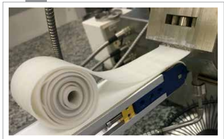
Scientists affiliated with the Food Research Center in Brazil are working to improve industrial feasibility of disruptive technologies such as the packaging that warns costumers when food starts spoiling (biofilm made from cassava starch (photo: Bianca Chieregato Maniglia / FoRC).
