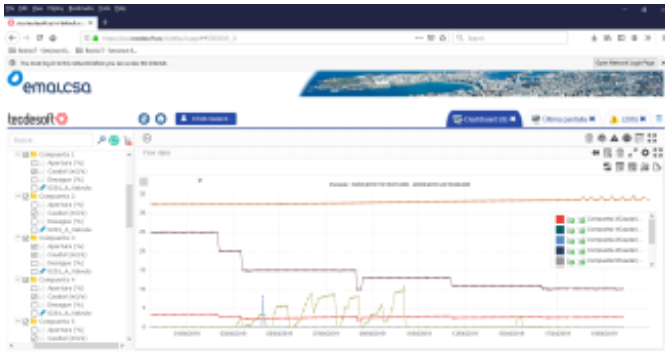
Fig. 9. Plot, in end user dashboard, of the data gathered by a water meter end device model
