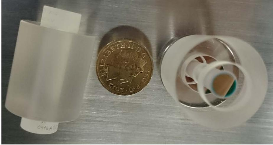
Figure 5.10: The cavities are multiband coated for stabilizing more than one laser in one cavity. The length of the ultra low expansion(ULE) cavity body is 30mm.
