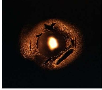
(b) MOT image without background by high power blue laser and repumping laser
