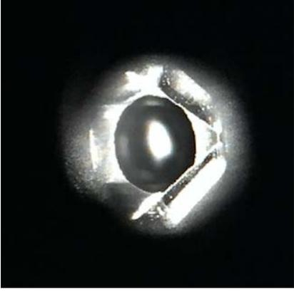
(a) Real MOT image by high power blue laser and repumping laser
