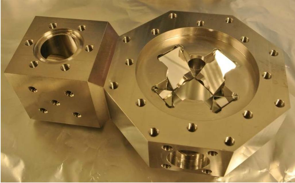
Figure 4.8: The octagonal chamber holds the prism mirrors for trapping the atoms. A valve, a dispenser and a ion pump with pumping speed of 2 L/s are connected to the vacuum setup through the cubic chamber. Some strontium oxide sample is held in the borehole which connects the octagonal chamber and the cubic chamber.
