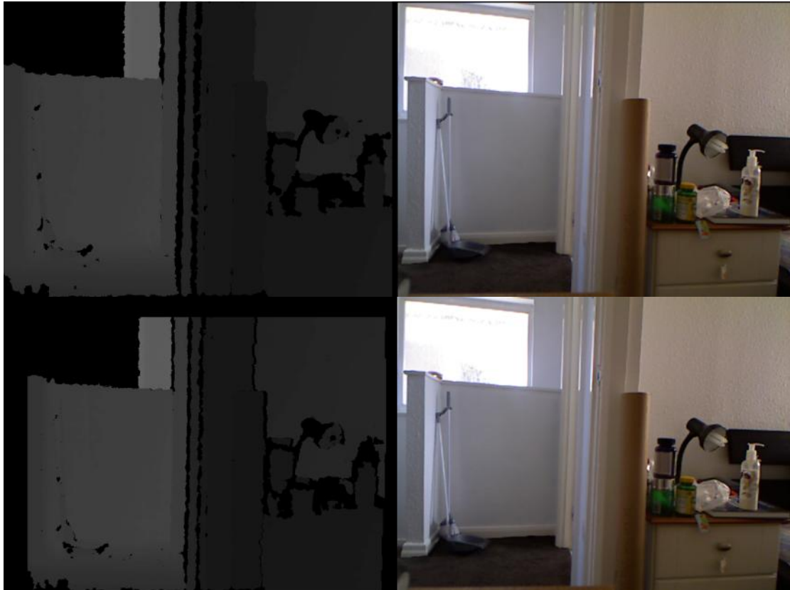
Figure 2-12: the unregistered depth image (upper) and the registered depth image (lower) with their corresponding colour image captured by Kinect.
