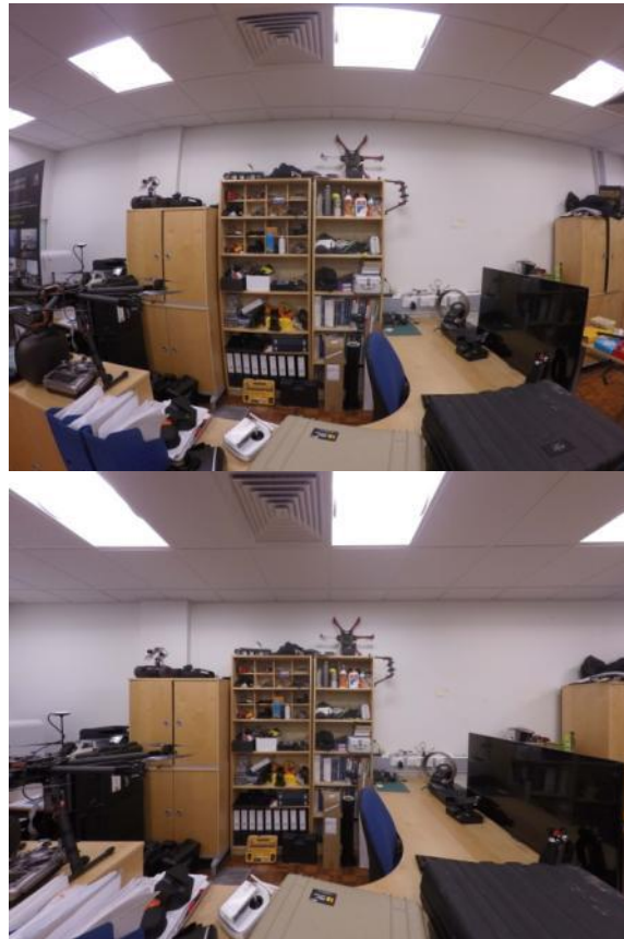
Figure 3-14: An image with fisheye lens distortion before distortion correction (left) and after correction (right).
