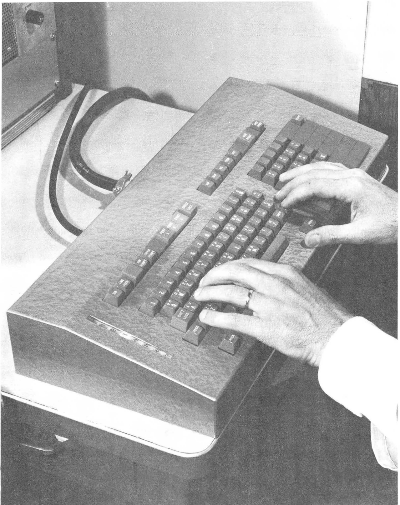
Fig. 1. The expanded character keyboard for inputting data into Table of Isotopes files.
