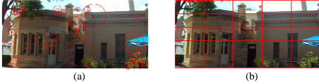
Fig. 5. Visual place description techniques fall into two broad categories. (a) Interesting or salient parts of the image are selected for extraction, description and storage. For example, SURF [73] extracts interest points in an image for description. The number of possible features may vary depending on the number of interest points detected in the image. The red circles are interest points selected by SURF within this image. (b) The image is described in a pre-defined way without first detecting interest points. Whole-image descriptors such as Gist [74], [75] divide an image into blocks as shown by the red lines and processes each block regardless of its content.
