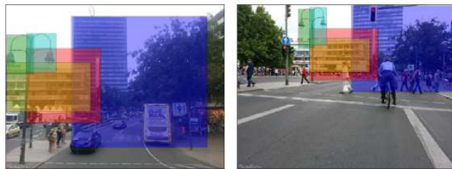
Fig. 7. Object proposal methods such as the Edge Boxes method [123] shown here were developed for object detection but can also be used to identify potential landmarks for place recognition. The colored boxes in the images above show landmarks that have been correctly matched between two viewpoints of a scene (from [122]).
