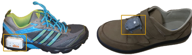
Fig. 2: Sensor setup for the lab data set (left) and validation data set (right), the sensors are highlighted with boxes.
