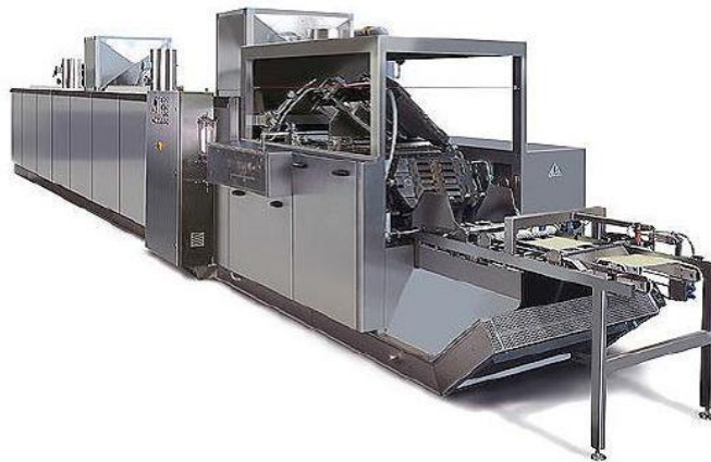
Figure 31 Typical baking oven from FHW
