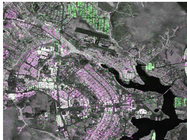
Fig. 14: Overlay of monostatic (magenta) and bistatic (green) SAR image.
