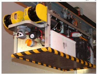
Batteries can be charged from the mains (380 V plug), and by monorail power feed rail in any position in the tunnel (when stopped) via an automatic power connector.
