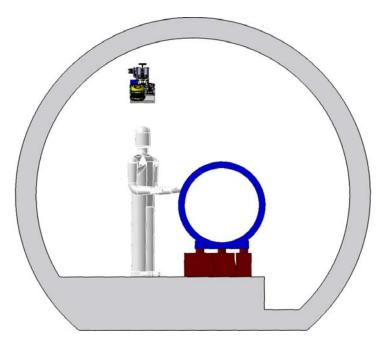
This TIM can travel faster than the standard TIM (up to 12 km/h) since it will probably be used to urgently reach zones in which a machine failure has happened and give an image/radiation feedback to guide the maintenance. It will be able to travel to the destination automatically once the operator enters the Dcum number.
