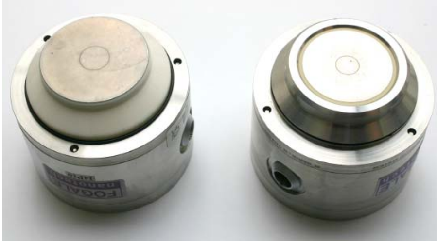
Figure 1. Two different types of HLS sensors (left: 1 st generation, right: 4 th generation)
