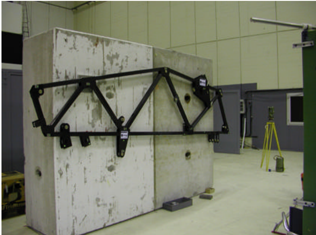
MAB Prototype in ISR during the deformation test
