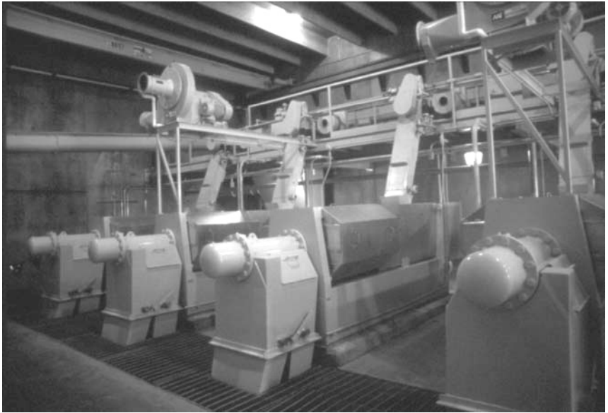
Figure 2. Photograph inside a modern soybean screw-press plant (courtesy of West Central Cooperative, Ralston, IA). (This figure is available in full color at http://www.mrw.interscience.wiley.com/biofp .)
