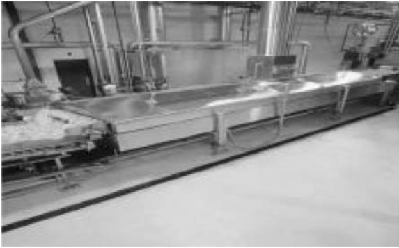
Figure 15. Corn chip fryer (Courtesy of Heat & Control Co.).
