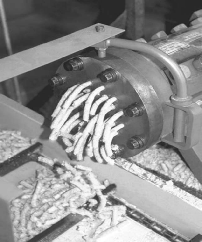
Figure 16. An expander making soybean collets for solvent extraction. Courtesy of Anderson International, Cleveland, Ohio. (This figure is available in full color at http://www.mrw.interscience.wiley.com/biofp .)
