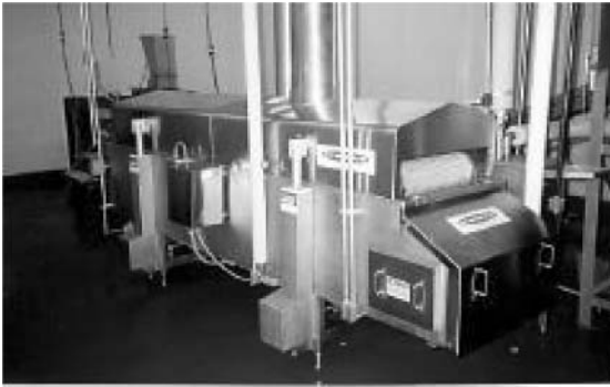
Figure 8. Direct fired fryer (Courtesy of Heat & Control Co.). (This figure is available in full color at http://www.mrw.interscience.wiley.com/biofp .)
