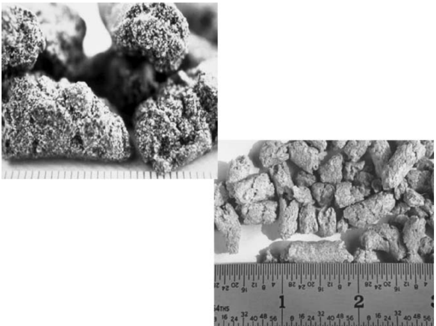
Figure 18. Collets made from pre-press canola and rice bran by expander for solvent extraction. Courtesy of Anderson International, Cleveland, Ohio. (This figure is available in full color at http://www.mrw.interscience.wiley.com/biofp .)
