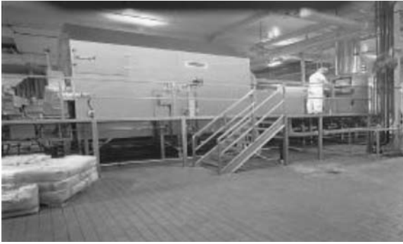
Figure 17. Low-oil potato chip-making system (Courtesy of Heat & Control Co.).
