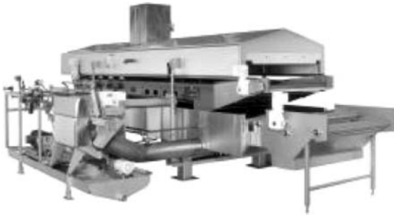
Figure 14. Tortilla chip fryer (Courtesy of Heat & Control Co.). (This figure is available in full color at http://www.mrw.interscience.wiley.com/biofp .)
