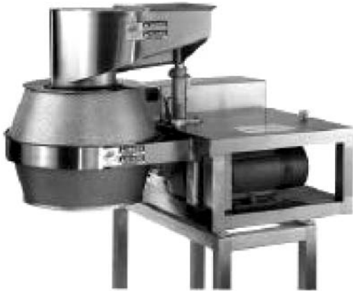
Figure 11. High-speed potato slicer (Courtesy of Urschel Co.).
