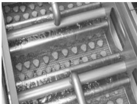
Figure 16. Heat wave fryer (Courtesy of Heat & Control Co.). (This figure is available in full color at http://www.mrw.interscience.wiley.com/biofp .)
