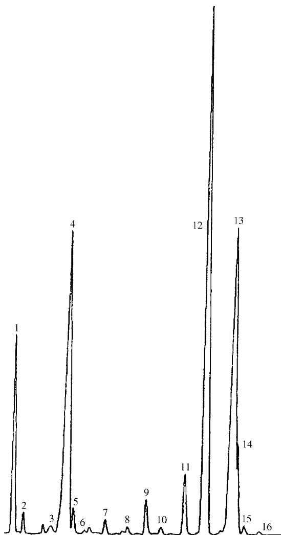
Figure 7. Part of gas-liquid chromatographic analysis of methyl esters of cod liver oil on an Omegawax-320 column, 0.32 \times 30 \times 0.25 . Temperature 160^{\circ}\text{C} for 8 min, 3^{\circ}\text{C}/\text{min} to 220^{\circ}\text{C} , hold. Peaks identified are as follows: 1 = 18:4n-3 ; 2 = 18:4n-1 , unmarked probably 18:5n-3 ; 3 = 20:0 ; 4 = 20:1n-9 with frontal shoulder of 20:1n-11 after peak 3; 5 = 20:1n-7 ; 6 = 20:1n-5 ; unknown; 7 = 20:2n-6 ; unknown; 8 = 20:3n-6 ; 9 = 20:4n-6 ; 10 = 20:3n-3 ; 11 = 20:4n-3 ; 12 = 20:5n-3 ; small peak for 22:0 ; 13 = 22:1n-13 + 22:1n-11 ; 14 = 22:1n-9 ; 15 = 22:1n-7 ; 16 = 22:1n-5 (Ackman, unpublished).
