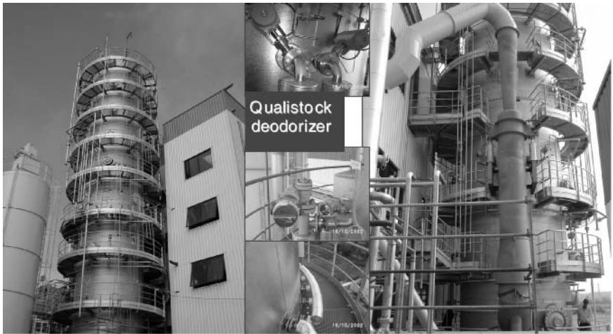
Figure 25. Modular single-vessel stand-alone deodorizer (Qualistock-De Smet).
