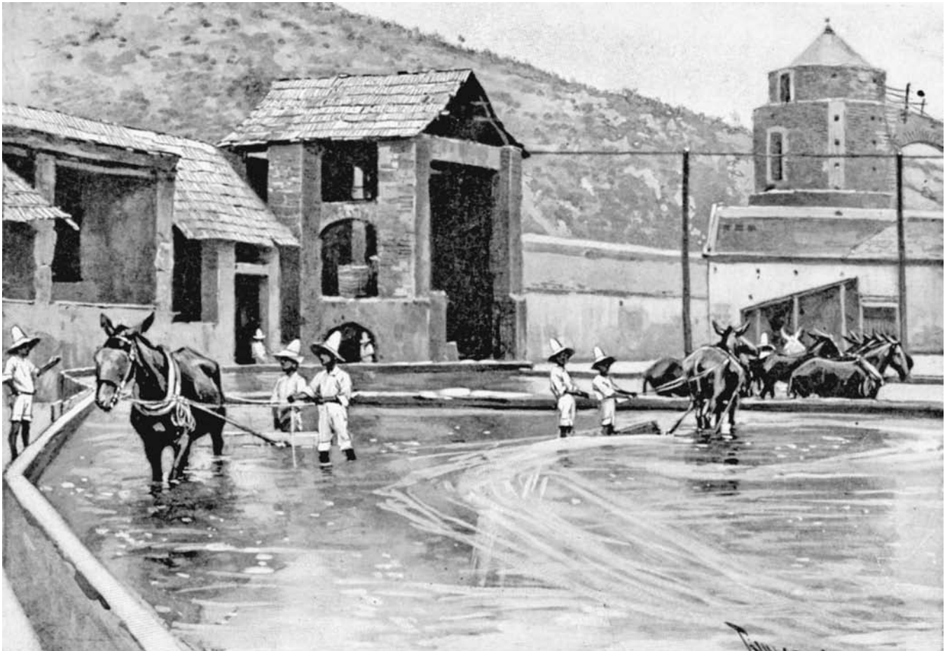
The patio process using mercury enabled using lower-quality silver ore than smelting did. (From the collections of the Mercantile Library at the University of Missouri–St. Louis)
