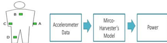
Figure 55. Placement of the accelerometer on the body: A: Wrist, B: Chest, C: Hip, D: Leg, and Block diagram of the measurement system.
