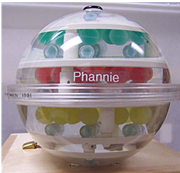
Figure 15. NIST-Developed MR system phantom. In addition to geometry, biomedical quantities such as proton density, T_1(\mathbf{r}) , and T_2(\mathbf{r}) are defined and characterized by independent means. How accurate are MR-based measurements of these quantities in research and clinical settings?
