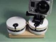
[Panner With Arduino](#) This project it's a new time-lapse tripod or panning with two axis that works with an arduino protoboard. Everyone will be able to create their own time-lapse trajectory without need to check it. With the arduino code we'll can change the value for the movement..... Listed under: [Motor Projects](#)
