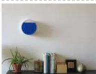
293. [Tidal Clock](#) This is a tutorial for making the Tidal Clock. The clock shows the ebb and flow between high and low tide by a rising and falling water level. It consists of an airtight acrylic container that has a front visible chamber and a back hidden..... Listed under: [Clock – Timer Projects](#)
