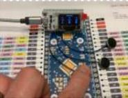
[ESP32 Capacitive Touch Input Using "Metallic Hole Plugs" for Buttons](#) <https://youtu.be/qQG8SdMgj8I> As I was finalizing design decisions for an upcoming ESP32 WiFi Kit 32 based project requiring three button input, one noticeable problem was that the WiFi Kit 32 does not possess a single mechanical pushbutton, yet alone three mechanical buttons, for input. However, the..... Listed under: [Wifi - WLAN Projects](#)
