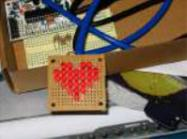
[Arduino Charliplexed Heart, Just in Time for Valentines Day](#). Here is an Arduino controlled Charliplexed LED heart just in time for Valentine's Day. It uses a total of 6 wires to controll the 27 LEDs. A PIC or AVR could easily be used for this, but I have Arduinos lying around and they are..... Listed under: [LED Projects](#)
