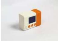
[Smart Thermostat](#) Connect your home heater to Internet and chat with it via Telegram! Things used in this project Hardware components Arduino MKR1000 × 1 DHT22 Temperature Sensor × 1 SparkFun Pushbutton switch 12mm × 3 Resistor 10k ohm × 4 LCD screen × 1 Software apps..... Listed under: [Projects](#), [Temperature Measurement Projects](#)
