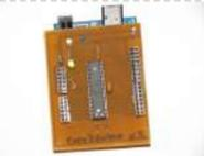
[Core2duino Updated with Arduino](#) This instructable will show you how to build an Arduino shield that adds another Atmega168/328 on top of your Arduino, giving you an extra complete set of I/O pins to use. That's 12 PWM pins, 12 Analog pins, 4 external interrupts, or 40 Digital pins..... Listed under: [Ideas](#), [Interfacing\(USB – RS232 – I2c -ISP\) Project Ideas](#)
