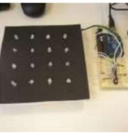
[RGB LED Grid](#) This project involved creating a red, blue, green (RGB) light emitting diode (LED) matrix that displayed the colors of the rainbow. The colors of the rainbow were chosen to show the full color spectrum that the LEDs are capable of, while still giving distinct variation..... Listed under: [LED Projects](#)
