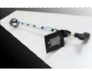
[Assistance for Visually Impaired featuring 4Duino-24](#) Blind Assistance is a project designed to help visually impaired people detecting obstacles in their way. It uses 4Duino, three ultrasonic sensors, one vibration motor and an LED. These components are attached to a walking stick. Blind Assistance alarms the user if there's an obstacle..... Listed under: [Wireless Projects](#)
