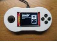
[Berry Racer – a Game Programmed in Arduino and Played on a Custom PCB](#) <https://youtu.be/C8IPaMl1wTk> Berry Racer is a game that I came up with and programmed using Arduino's Software. The game is run on a Teensy microcontroller which is connected through a custom PCB (Printed Circuit Board) to a Screen, a Joystick, four buttons, and a piezo speaker..... Listed under: [Game – Entertainment Projects](#)
