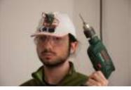
[Eye Guardian: Sound Triggered Eye Protection](#) Eye Guardian is an Arduino powered, High-Decibel continuous sound triggered eye protection wear. It detects heavy equipment sound and lowers protective eye goggles while the equipment is in use. Outline In the first step, I will explain the Inspiration&Idea behind this project. Next, I will..... Listed under: [Sound – Audio Project Ideas](#)
