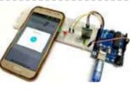
[Voice Controlled LEDs using Arduino and Bluetooth](#) Controlling LEDs with voice command seems to be a difficult task, but it's easy and you can quickly build it. We just need an Arduino UNO to serially communicate with HC-06 Bluetooth module and a smartphone to send voice command to Bluetooth module HC-06. For..... Listed under: [Bluetooth Projects](#)
