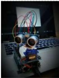
226. [Ultrasonic Mapmaker Using Arduino and MatLab](#) Vision is one of the most exciting senses you can endow on your robot. The ability to perceive obstacles allows a robot to make an educated decision regarding further movements. However, it is also not the easiest senses to implement for a few reasons. Firstly,..... Listed under: [Other Projects](#)
