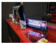
165. [Totally Lit – Programmable RGB LED Acrylic Sign](#) <https://youtu.be/AcvpgUQGpn4> Been playing around with the laser cutter/engraver, and really fell in love with engraving in to clear acrylic and shining a light source from the edge. The thickness of the acrylic being used is a .25" sheet, which cuts really cleanly by the laser..... Listed under: [LED Projects](#)
