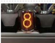
298. [How to Control a Nixie Tube With an Arduino](#) A Nixie Tube is a Neon gas-filled tube, that has a wiremesh anode with various cathodes shaped like numbers or symbols. Back in the 1950s they were used in computers, calculators, and laboratory equipment. Nixie tubes were replaced by LEDs and VFDs(vacuum fluorescent displays)in the..... Listed under: [Other Projects](#)
