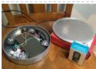
[Smart IOT Propane Monitoring Pedestal](#) Smart IOT Propane Pedestal capable of tracking propane level as well as detecting any propane leaks. Integration with Amazon Alexa. Things used in this project Hardware components Arduino MKR1000 × 1 SparkFun Load Sensor 50kg × 4 SparkFun Logic Level Converter - Bi-Directional × 1..... Listed under: [Projects](#), [Sensor – Transducer – Detector Projects](#)
