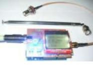
[ARDUINO UNO FM AM TRANSMITTER CIRCUIT SI4713](#) The most important part is the construction of a functional sample of a Arduino Uno software-defined one transmitter. After agreement with the supervisor and current options, she was elected concept with SI4713 digital circuit... Electronics Projects, Arduino Uno FM AM Transmitter Circuit SI4713 "arduino projects, microcontroller projects, " The..... Listed under: [Radio Projects](#)
