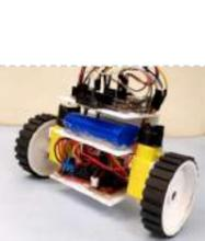
[DIY Self Balancing Robot using Arduino](#) After being inspired by RYNO motors and other self balancing scooters from Segway, I always wanted to build something similar. Thinking for while, I decided to build a Self Balancing Robot using Arduino. This way I would be able to grasp the underlying concept behind all..... Listed under: [Robotics – Automation Projects](#)
