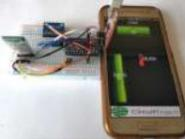
[DIY Arduino Inclinometer using MPU6050](#) The MPU6050 is an IC 3-axis accelerometer and a 3-axis gyroscope combined into one unit. It also houses a temperature sensor and a DCM to perform a complex task. The MPU6050 is commonly used in building Drone and other remote robots like a self-balancing robot..... Listed under: [Bluetooth Projects](#)
