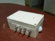
[Adaptable Sensor and Notification System](#) A easy to use adaptable sensor and notification system that is designed to be used as a temporary change of state notifier. Things used in this project Hardware components Arduino MKR1000 × 1 PIR Motion Sensor (generic) × 1 SW-420 Motion Sensor Module Vibration Switch..... Listed under: [Arduino Programmer Projects](#), [Internet – Ethernet – LAN Projects](#), [Projects](#)
