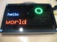
[Mirolo Networked LED Matrix Display for Digital Signage](#) Digital signage can be useful at events to inform visitors about upcoming panels, changes in the schedule or dynamically provide information. Using LED Matrix displays for that makes the messages readable even from far away and is an eye catching feature. Features include: 2 Lines..... Listed under: [Arduino Battery Project Ideas](#)
