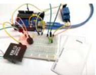
[Arduino RFID Door Lock](#) You have seen RFID Door Lock Mechanism in some Hotels and other places, where you don't need a key to unlock the room. You are given a card and you just need to put it in front of a RFID Reader box, and the lock gets unlocked..... Listed under: [Security – Safety Projects](#)
