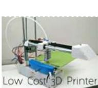
297. [Edge 3D Printer 1.0 – an Affordable Open Source 3D Printer!](#) Hello everyone! In this instructable I will show you how to make a low cost 3d printer that I designed! It should cost around \$150 US dollars or \$175 Canadian dollars, if you buy from the links provided in this project (parts are from Aliexpress)..... Listed under: [CNC Machines Projects](#)
