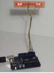
[Charlieplexed row of LED lights, for the Arduino](#) This is my instructable on charlieplexing a LED row/string with the arduino. I noticed that there weren't many instructables on charlieplexing using an arduino, so i made this. I tried to keep the project simple, but that didn't work very well. The soldering is complex,..... Listed under: [Arduino LED Project Ideas](#), [Ideas](#)
