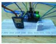
830. [Digital Thermometer using Arduino and DS18B20 Sensor](#) In this project, we are going to make a Digital Thermometer using Arduino Uno. We will use DS18B20 temperature sensor to sense the temperature and Nokia 5110 LCD to display it. DS18B20 is a 1-Wire digital temperature sensor manufactured by Maxim Integrated and is capable..... Listed under: [Calculator Projects](#), [LCD Projects](#)
