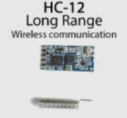
263. [Long Range, 1.8km, Arduino to Arduino Wireless Communication With the HC-12.](#) <https://youtu.be/DGRPqeaCJns> In this instructable you will learn how to communicate between Arduinos over a long distance up to 1.8km in open air. The HC-12 is a wireless serial port communication module that is very useful, extremely powerful and easy to use. First you will learn..... Listed under: [Wireless Projects](#)
