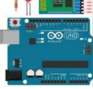
[Arduino Bluetooth Basic Tutorial](#) Ever thought of controlling any electronic devices with your smart phone ?Controlling your robot or any other devices with your smartphone will be really cool. Here is is a simple and basic tutorial for interfacing Bluetooth with arduino Step 1: Things You Need Hardware Bluetooth Module HC 05/06ArduinoLED220Ω ResistorAndroid device..... Listed under: [Bluetooth Projects](#)
