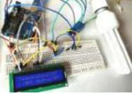
[Temperature Controlled AC Home Appliances using Arduino and Thermistor](#) Suppose you are sitting in a room and feeling cold and you want your heater to be automatically turned on, and then off after some time when room temperature is increased, then this project help you to control your home appliances automatically according to the..... Listed under: [Battery Projects](#), [LCD Projects](#)
