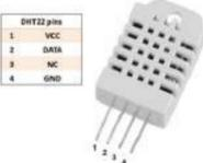
[Temperature and Humidity monitoring with DHT22 sensor Arduino Uno R3](#) The objective of this tutorial is to learn how to use the DHT22 sensor with Arduino uno. The room temperature and humidity will be printed to serial monitor and also will be displayed to the LCD 4×20 in Proteus ISIS. [caption id="attachment\_28379" align="aligncenter" width="300"] DHT22..... Listed under: [Temperature Measurement Projects](#)
