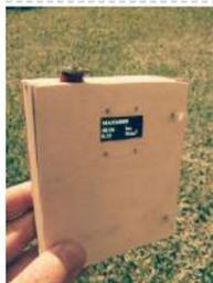
166. [Portable Luxmeter](#) This project is about making portable luxmeter. It can be used in schools, where children can measure different kinds of light sources.Functions: 1. measure intensity of light in lux. 2. calculate solar irradiation from lux to watts/m2 (factor 112) 3. charging battery using USB port..... Listed under: [Battery Projects](#)
