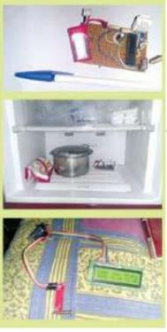
[Microcontroller Projects: Fridge Temperature and Humidity Indicator](#) We can measure temperature and humidity inside the fridge using a normal temperature-humidity indicator but relative humidity (RH) could be inaccurate in that case. The moment the fridge door is opened, RH will shoot up due to ingress or egress of moisture in the surroundings..... Listed under: [Sensor – Transducer – Detector Projects](#)
