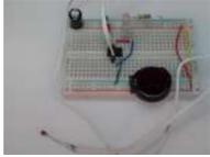
[Hot Yet? This faucet water monitor will prevent plunging your hands into cold water](#) Hot Yet? Attiny85 Faucet Water Temperature Sensor Testing Real life testing in the kitchen sink! Note the tri-color LED. Blue is cold and fades into Green which then flips to increasing Red at 85F. Notes This project is an Attiny85 Arduino circuit and uses..... Listed under: [Metering – Instrument Project Ideas](#)
