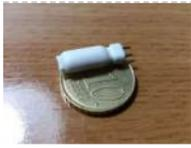
287. [DIY Tilt Switch](#) In this instructable I'll show you how to make a simple tilt switch, this tilt switch works best with microcontrollers that can debounce the signal and overcome interferences produced by vibrations. There are many ways to make a tilt switch, this one is a cheap..... Listed under: [Other Projects](#)
