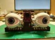
[Motion Follow Animatronics Eyes](https://youtu.be/Ep9fWQifmoM) <https://youtu.be/Ep9fWQifmoM> This Arduino project uses an Optical Flow Sensor (ADNS3080) to capture movement. Then translate the data to move servo's making it look as eyes are following moving object. This is not an easy build. It requires 3d printing, soldering, some general technical understanding and..... Listed under: [LED Projects](#)
