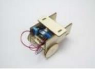
[MKR1000 Robot Controlled Via WiFi Using Arduino](#) This project consists of a small robot controlled via WiFi using an Arduino MKR1000, MKR2UNO Shield Adapter and Arduino Motor Shield! Things used in this project Hardware components Arduino MKR1000 × 1 Arduino MKR2UNO Adapter × 1 Arduino MotorShield Rev3 × 1 Arduino Small DC..... Listed under: [Battery Projects](#), [Robotics – Automation Project Ideas](#)
