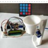
[Automatic Pet Feeder using Arduino](#) Today we are building an Automatic Pet Feeder Using Arduino which can automatically serve food to your pet timely. It has a DS3231 RTC (Real Time Clock) Module, which used to set time and date on which your pet should be given food. So, by..... Listed under: [Clock – Timer Projects](#)
