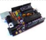
[DIY Arduino-Compatible Clone](#) The Arduino is the ultimate tool in the Maker's arsenal. You should be able to build your own! In the early days of the project, circa 2005, the design was all through-hole parts and communication was via a RS232 serial cable. The files are still available, so you can..... Listed under: [Interfacing\(USB – RS232 – I2c -ISP\) Project Ideas](#)
