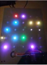
[5x5 rgb lpd6803-led matrix arduino controlled](#) what: a 5\*5 rgb led matrix, made with arduino and lpd6803 based leds from adafruit. with an pir sensor, it goes on if it detects movements and a ir distace sensor, 1 animation shows the distance you have from the sensor :). why: because its..... Listed under: [LED Projects](#), [Projects](#)
