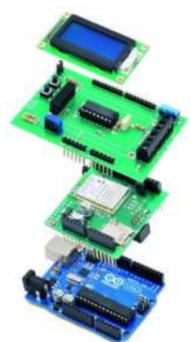
540. [Wi-Fi Body Scale with Arduino Board](#) In this post we present the design of a scale that connects to the Internet and automatically sends weight info on a Google Document. The project is composed of Arduino Uno board Wi-Fi shield additional shield that we used to manage data collection and I/O with..... Listed under: [Internet – Ethernet – LAN Projects](#), [Medical – Health based Projects](#), [Projects](#)
