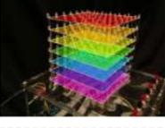
[Self-Contained 7x7x7 LED Cube using Arduino](#) LED cubes are true 3D displays that work by lighting up points in a 3D lattice of LEDs. On the 3D display you can produce some truly mesmerizing animations. This Instructable will walk you through creating an LED cube for yourself that is completely self-contained and powered..... Listed under: [LED Projects](#), [Projects](#)
