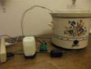
[Precision Fermentation: Arduino-Controlled Crock Pot Yogurt Maker](#) A homemade thermostat attachment for a crock pot (or other electric heating device). It can be used to precisely control the temperature of the crock pot for things like yogurt fermentation. Why Making yogurt is fun. It is also way cheaper than buying it. You..... Listed under: [Home Automation Projects](#)
