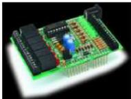
54. [A useful and simple IO Shield for Arduino](#) In order to "visually" highlight the behavior of Arduino programs you must connect a device to the I/O pins, which gives you tangible signals. Normally, if you want to check if a program changes a level of an output pin, answering a command or executing..... Listed under: [Development Board – Kits Projects](#), [How To – DIY – Projects](#)
