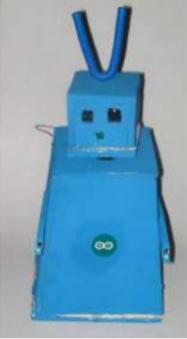
[Uno The Arduino Robot](#) Age: 13 Meet Uno the Arduino powered robot. Some functions include a blinking nose, moving antennas, rotating head, IR distance sensor, twin motor gear box and rotation counters. Uno is made with relatively easy to obtain parts. This project provides a good introduction to Arduino. robot.skp475 KB Step 1: Materials Material and tools • Foam board..... Listed under: [Projects](#), [Robotics – Automation Projects](#)
