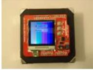
214. [Arduino-Square with Color LCD](#) B-Squares is a modular electronics platform that enables users to build, customize, and continuously update their own electronics applications. In this B-Squares App we will cover how to assemble a simple Color-LCD Application using the Arduino-Square. Hardware: 1. Arduino-Square. 2. Battery-Square 3. Color LCD Shield..... Listed under: [LCD Projects](#), [Projects](#)
