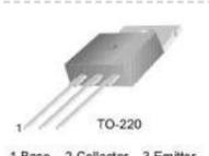
[Using a transistor to control high current loads with an Arduino](#) In this tutorial, you'll learn how to control a high-current DC load such as a DC motor or an incandescent light from a microcontroller. (:toc Table of Contents:) Connect a transistor to the microcontroller The transistor allows you to control a circuit that's carrying higher..... Listed under: [Interfacing\(USB – RS232 – I2c -ISP\) Project Ideas](#)
