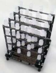
[Arduino LED Cube Spectrum Analyzer](#) In this project we'll create a small add-on PCB containing the a MSGEQ7 spectrum analyzer circuit and show how it can drive the RGB LED cube kit from Freetronics. This allows the cube to display the seven bands over four horizontal planes. There is a small amount..... Listed under: [LED Projects](#)
