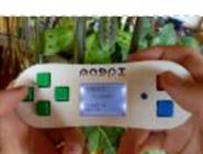
[Magpi: The Micro Arduino Gaming Platform Interface](#) Here's a retro hand-held gaming console I built with my son. It uses an Arduino micro-controller, a small LCD screen, push-buttons, a 3D printed case and home-grown "PC" board. It's really pretty easy to solder and put together. My son & I wrote two games..... Listed under: [Game – Entertainment Projects](#)
