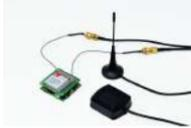
[Localizer with SIM908 module using Arduino](#) The device is based on a GSM/GPRS module with included GPS. Its main function is to detect and communicate its own geographical position using, on the choice, the cellular phone reference system or the GPS. Its small dimensions are due to the use, for the..... Listed under: [GPS Based Projects](#), [Phone Projects](#), [Projects](#)
