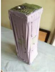
45. [New Textiles 2012 using arduino](#) Twist Switch by ttseng Through the action of twisting, swatches of conductive fabric are folded in upon each other, completing a circuit that then turns on LEDs. On each face of stretched spandex are swatches of conductive fabric. Before choosing which swatches to designate as..... Listed under: [LED Projects](#)
