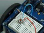
[Making a program start using a switch](#) Connecting the Switch To connect the switch to the Arduino, you will need the switch, two jumper wires, and a 10kΩ (brown-black-orange) resistor. Once you have all the required parts, you will need to wire the switch to the Arduino using the breadboard. NOTE: The..... Listed under: [Arduino Programmer Projects](#)
