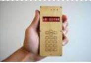
[Make your own cellphone from scratch](#) The DIY Cellphone is a working (albeit basic) cellphone that you can make yourself. It can make and receive phone calls and text messages, store names and phone numbers, display the time, and serve as an alarm clock. It connects to GSM networks (like AT&T and T-Mobile..... Listed under: [How To – DIY – Projects](#), [Phone Projects](#)
