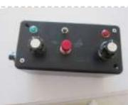
[Arduino compatible Luna Mod Looper](#) The Luna Mod Looper, basically lets you record a sequence using a potentiometer to control the pitch of the note, and then play it back and add affects. Ever since I saw videos of the Luna Mod being played, I wanted to build my own..... Listed under: [Projects](#), [Sound – Audio Projects](#)
