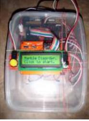
[Marble Disorder – a marble maze simulator with tilt switches using Arduino](#) Marble Disorder is a borderline case of Marble Madness 😊 It simulates a marble maze by sensing the box's orientation with 2 tilt switches. Stop the press: there's a new and more intuitive version that doesn't require the spin knob (See video). I keep documenting the original..... Listed under: [Game – Entertainment Projects](#), [Projects](#)
