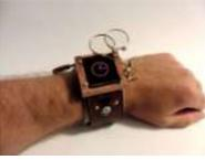
[Arduino Watch Build Instructions](#) Update: New version out that works with Arduino 1.0 and higher! The Arduino Watch provides augmented sensing of temperature and range, 16-bit color drawing program, Breakout game, and also tells the time in your choice of digital, binary, or analog. Additional sensors, devices, and programs..... Listed under: [Clock – Timer Projects](#), [Projects](#)
