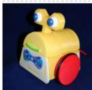
262. [Sensor Less 3d Printed Robot](#) Tyree (he wears a tie and he has tires) actually smiles after he bumps into something (see video). Using an Arduino motor shield, he detects obstacles using the "more current into the motor means something is in the way" principle. Tyree started out as a..... Listed under: [Robotics – Automation Projects](#), [Sensor – Transducer – Detector Projects](#)
