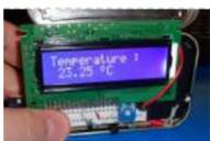
817. [Arduino Temperature Sensor Code](#) This arduino projects show how to read Celsius and Fahrenheit temperature with LM35 temperature sensor. Parts List; 1) 1x 16x2 parallel LCD display (compatible with Hitachi HD44780 driver) 2) 1x Arduino 3) 1x 10kΩ potentiometer 4) 1x LM35 temperature sensor 5) Jumper wire Instruction; 1)..... Listed under: [Projects](#), [Sensor – Transducer – Detector Projects](#), [Temperature Measurement Projects](#)
