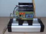
[Arduino-Controlled Physics Lab Fan-Cart](#) A "fan cart" is a roughly constant-force device used in introductory physics labs. It consists of a fan (usually a model airplane propeller on a brushed DC motor) mounted on top of a low-friction cart. Students use it to pretend they're learning something about force,..... Listed under: [Interfacing\(USB – RS232 – I2c -ISP\) Project Ideas](#)
