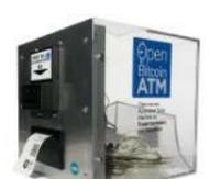
[Open Bitcoin ATM using arduino](#) The world's first completely open-source Bitcoin ATM for Education and Experimentation. <http://openbitcoinatm.org> for more information. Step 1: Fabricate Box and Faceplate Out of a piece of 12"x12" aluminum sheet metal, cut two rectangles and drill six rivet holes and four holes to attach the bill acceptor..... Listed under: [Robotics – Automation Projects](#)
