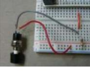
[Momentary Switch as Digital Sensor](#) In many cases switches are just switches. They directly control the flow of electricity to an appliance, flashlight or mains-voltage lamp. An example of this is the switch on the wall in your living room. In many cases nowadays however, switches are digital sensors, meaning..... Listed under: [Sensor – Transducer – Detector Projects](#)
