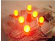
213. [Arduino Led Dice](#) This instructable will show you how to create a dice using Arduino and few components. It's an easy and fun project, suitable for beginners and those who want to start with Arduino; it also requires a minimal amount of components. This explains how to create..... Listed under: [LED Projects](#), [Projects](#)
