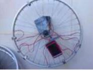
[Solar theremin with Arduino using arduino](#) materials: arduino uno 3 photoresistors 4 buzzers 3 10k resistor (optional) usb solar pannel or usb battery Step 1: Why? During the 2014 art Exhibition at Met (M. di Ragusa), I created (with the technical collaboration of Carmel Iurato), this theremin made from three photoresistors,..... Listed under: [Solar energy project Ideas](#)
