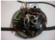
[LINUSBot – Line Follower Robot using Arduino](#) The operation of this Robot is quite simple. Infra-red sensors placed at the front of the chassis will monitor when our Robot is over a black line or when it is over a white background. In this project we will use the appropriate rounded chassis..... Listed under: [Projects](#), [Robotics – Automation Projects](#)
