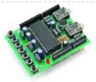
[A Voice Shield for Arduino Board](#) The objective of this project is to build an Arduino voice shield to empower thousands of voice related applications! All this mostly thanks to an integrated ISD1790PY chip. This particular voice/TTS feature can be useful to integrate voice messages in alarm systems, to implement generic..... Listed under: [Projects, Sound – Audio Projects](#)
