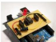
723. [Stripboard Arduino shield for programming ATtiny45 and ATtiny85](#) This instructable (entered in the Arduino Challenge contest - you can vote for it above) shows how to make a stripboard Arduino shield for programming either ATtiny45 or ATtiny85 microcontrollers with an Arduino, as per these tutorials from the High-Low Tech group at MIT: Arduino..... Listed under: [Arduino Programmer Projects](#), [Interfacing\(USB – RS232 – I2c -ISP\) Projects](#), [Projects](#)
