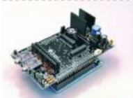
[GSM GPS shield for Arduino Board](#) Shield for Arduino designed and based on the module GSM/GPRS SIM900 or the GSM/GPRS & GPS module SIM908, to make calls, voice and data connections via GPRS. HARDWARE INNOVATIONS This new version (old Arduino GSM shield) has several new hardware features, that allow maximum customization..... Listed under: [GPS Based Projects](#), [Phone Projects](#), [Projects](#)
