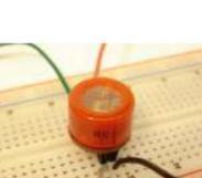
[Arduino Breathalyzer: Calibrating the MQ-3 Alcohol Sensor](#) The MQ-3 is an alcohol gas sensor that is available for about \$5 from Sparkfun, Seeed Studio, and others. It's easy to use and has sparked the imagination of anyone who has dreamed of building their own breathalyzer device for measuring the amount of alcohol..... Listed under: [Sensor – Transducer – Detector Projects](#)
