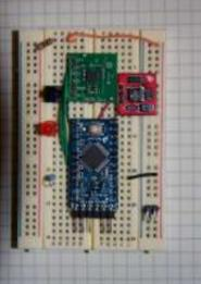
[Simple Datalogger](#) Here's a simple Arduino-based datalogger I'm currently developing: This test-of-concept model is based on the Arduino Pro Mini (ATMega168). It runs on a 1.5-V battery, using a voltage up-converter from Sparkfun.com. For a sensor, it's using a 3-axis accelerometer on a breakout board, also from..... Listed under: [Development Board – Kits Projects](#)
