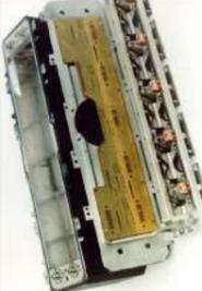
[The Photometric Camera and the CCDs](#) The Photometric System The photometric camera for the SDSS consists of two TDI scanning CCD arrays, one, using 30 Tektronix/SITe 2048 x 2048 CCDs in a 5 by 6 array for five-color photometry, and the other using 24 2048 x 400 chips for astrometry and..... Listed under: [Video – Camera – Imaging Projects](#)
