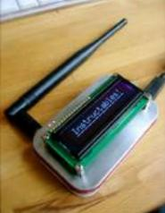
[Wireless Altoids Display using an Arduino](#) This Instructable will show you how to modify an Altoids tin for a wireless 2x16 character display. Using an Altoids tin was inspired by the need to have a small yet protective enclosure for a pair of Xbee modules recently bought from Sparkfun. I purchased the..... Listed under: [LCD Projects](#), [Projects](#)
