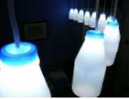
[Addressable Milk Bottles \(LED Lighting + Arduino\) using arduino](#) Make PPE milk bottles into good looking LED lights, and use an Arduino to control them. This recycles a number of things, mainly the milk bottles, and uses a very low amount of power: the LEDs apparently dissipate less than 3 watts but are bright..... Listed under: [LED Projects](#)
