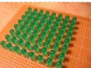
[LED matrix using shift registers using arduino](#) This instructable is meant to be a more complete explanation than others available online. Notably, this will provide more hardware explanation than is available in the LED Marquee instructable by led555. Goals This instructable presents the concepts involved with shift registers and high side drivers..... Listed under: [LED Projects](#)
