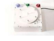
[Wrap Beats – Capsense Arduino Instrument](#) Wrap Beats is an instrument that lets you string together notes in order to create different melodies and visual patterns. I constructed it using the Capacitive sensing library for Arduino and combining that with the music abilities of processing to create a dynamic instrument that..... Listed under: [Sound – Audio Projects](#)
