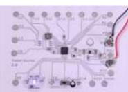
[Paperduino 2.0 with Circuit Scribe – Paper Arduino](#) What if making an Arduino, or wiring up an Arduino was as easy as printing one out? In this tutorial we printed our own Arduino Pro Mini board using a pen plotter and the Electroninks Circuit Scribe (a rollerball pen with highly conductive ink). Within..... Listed under: [LED Projects](#)
