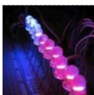
522. [How to Control a Ton of RGB LEDs with Arduino & TLC5940](#) This video explains how to use the 16 channel PWM controller TLC5940 The CODE: `//Texas Instruments TLC 5940 with Arduino //www.kevindarrah.com #include <SPI.h> //Serial Peripheral Interface Library byte ch=0, chbit=0, spibit=0, spibyte=0; // variables used by tlc sub routine int SINData; //variable used to shift data to the.....` Listed under: [LED Projects, Projects, PWM Projects](#)
