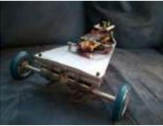
[CARduino – Arduino-Powered, LabVIEW-Controlled Vehicle](#) The CARduino is a remote-operated vehicle which is controlled by a controller attached to a computer running LabVIEW. The vehicle is powered by the Arduino, and can be expanded upon through the addition of sensors or other devices. Using LabVIEW, one can easily modify the..... Listed under: [Car Projects](#)
