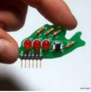
[Blinky Fish using an Arduino](#) Assembly instructions for an add-on board for the Arduino. \*\*\*\* FOR INSTRUCTIONS FOR MARCH 2013, KICKSTARTER PROJECT GO HERE <http://www.instructables.com/id/Blinky-Fish-Kickstarter-Project/> \*\*\*\*\* It has some LED's and a button. It connects to digital pins 9-13 and ground. My hope is that this will be useful to people that want to..... Listed under: [Game – Entertainment Projects](#), [LED Projects](#), [Projects](#)
