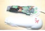
[Arduino and CueCat barcode scanner](#) I've had a cuecat barcode scanner sitting around for over 10 years. Basically it connects to a PS2 port (apparently there is a USB version) like a keyboard and spits out a barcode when scanned. Nice!. The annoying thing is that it is "encrypted". What..... Listed under: [Sensor – Transducer – Detector Projects](#)
