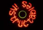
[Woooshing leds – Rotated animation by arduino](#) This project allows you draw in the air letters, symbols or other shapes - as you like. Controlled by the Arduino, the 7 simple leds blinking on and off - creating the illusion of floating text in the air. This combination of simple components with..... Listed under: [LED Projects](#)
