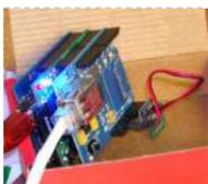
818. [Web Server using Arduino](#) In this example, you will use your Ethernet Shield and your Arduino to create a simple Web server. Using the Ethernet library, your device will be able to answer a HTTP request with your Ethernet shield. After opening a browser and navigating to your Ethernet..... Listed under: [Internet – Ethernet – LAN Projects](#), [Projects](#)
