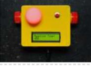
[Reaction Time Tester using an Arduino](#) A month ago I knew nothing about Arduino and now.....my first project! Looking back, this project combines almost all of the tutorials that I have read in this short period: blinking LED, push button, piezo and LCD display. A useful project for every beginner! I..... Listed under: [Clock – Timer Projects](#), [Projects](#)
