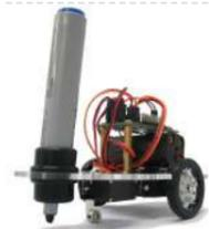
[Building a Doodle Bot kit from DAGU](#) Doodle Bot is a very simple beginners robot that can write messages using white board markers, jumbo chalk or crayons. The kit comes with all parts including an Arduino compatible controller and a screwdriver. You will need to supply 4x AAA batteries and a suitable..... Listed under: [Robotics – Automation Projects](#)
