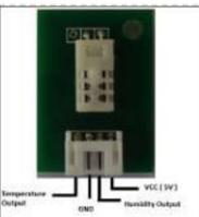
[HSM-20G Interface with Arduino Uno](#) The HSM-20G is an analog humidity and temperature sensor that outputs analog voltage respects to relative humidity and temperature. However from this sensor relative humidity is found along with temperature. Relative humidity is the percentage of moistures of airs for a particular temperature [1]. Feature:..... Listed under: [Interfacing\(USB – RS232 – I2c -ISP\) Projects](#)
