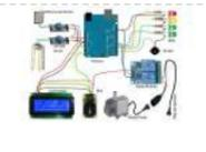
[Arduino Automatic Watering System](#) INTRODUCTION & OBJECTIVES: I is a simple system, using Arduino to automate the irrigation and watering of small potted plants or crops. This system does the control of soil moisture, doing indications via LEDs and in case of dry soil emitting a alarm beep. In..... Listed under: [Home Automation Projects](#), [Projects](#)
