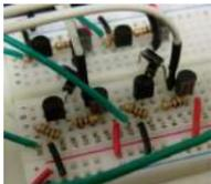
[Arduino MicroBot Project](#) Steps On the breadboard, build two bi-directional motor control circuits (also known as "H-bridge") circuits. These circuits will control the two DC motors that drive the wheels. Each circuit will have two wires from the Arduino (one for forward, one for backward) to control the..... Listed under: [Robotics – Automation Projects](#)
