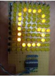
[Make a 8x10 L.E.D Matrix using arduino](#) UPDATE 1: I HAVE ADDED THE CODE FOR CONWAY'S GAME OF LIFE UPDATE 2: NOW YOU CAN SAVE SOME ARDUINO PINS WITH THE HELP OF 1 SHIFT REGISTER. In this instructable I will show you how to build a quite fancy 8 by 10 L.E.D matrix(with scrolling text and animations) using the Arduino and 4017 decade..... Listed under: [LED Projects](#)
