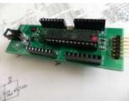
[Hobbyduino Mini V1.0 using arduino](#) Introduction The Hobbyduino Mini is a clone of the Arduino main-board. It contains a ATmega328 processor programmed with the Arduino bootloader. The Hobbyduino does not contain the circuitry for USB communication. I opted to rely on the FTDI232R serial boards to handle the USB-to-Serial protocol. Here..... Listed under: [Development Board – Kits Projects](#)
