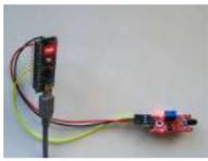
31. [Capturing IMU Data with a BNO055 Absolute Orientation Sensor](#) The Bosch BNO055 combines tri-axis accelerometers, gyroscopes, and magnetometers to provide orientation to users. About the Sensor The BNO055 uses three triple-axis sensors to simultaneously measure tangential acceleration (via an accelerometer), rotational acceleration (via a gyroscope), and the strength of the local magnetic field (via.....
