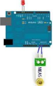
[How to Build a Vibration Detector Circuit](#) In this project, we will go over how to build a vibration detector circuit. This is a circuit which can detect and measure flex, touch, vibration, and shock. The sensor we will use to detect these movements is a piezo vibration sensor from Measurement Specialists (MEAS). The..... Listed under: [Sensor – Transducer – Detector Projects](#)
