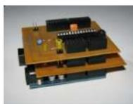
[Core3duino using arduino](#) This is an add-on shield to an add-on shield. That's right, you have to have the Core2duino on your Arduino to be able to understand why you would want this in the first place. So once you have your Core2duino saddled up, give this one..... Listed under: [Development Board – Kits Project Ideas](#)
