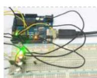
230. [RGB LED with Arduino](#) In this project we are going to interface 5 RGB (Red Green Blue) LEDs to Arduino Uno. These LEDs are connected in parallel for reducing PIN usage of Uno. The RGB LED will have four pins as shown in figure. PIN1: Color 1 negative terminal..... Listed under: [LED Projects](#)
