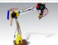
[Tertiarm – 3d Printed Robot Arm](#) This is first version of my low cost 3d printed robot arm. It is based on Ikea Tertial lamp. I choose it because it has very good kinematic with using springs to unload servos. So you can use different number of springs to achive different..... Listed under: [Robotics – Automation Projects](#)
