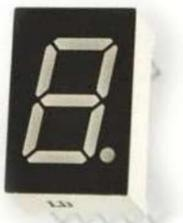
[How to Drive a 7 Segment LED Display with an Arduino](#) In this project, we will show how to drive a single 7 segment LED display with an arduino microcontroller. A 7 Segment LED Display is an electronic device housing 8 individual LEDs. Using this device, we can display all numerals and many alphabetical characters and many more..... Listed under: [LED Projects](#)
