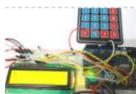
222. [Keypad Interfacing with Arduino Uno](#) In this tutorial we are going to interface a 4x4 (16 key) keypad with ARDUINO UNO. We all know keypad is one of the most important input devices used in electronics engineering. Keypad is the easiest and the cheapest way to give commands or instructions to..... Listed under: [Other Projects](#)
