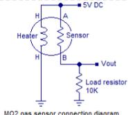
[LPG sensor using arduino](#) LPG sensor using Arduino with alarm and cutoff. A simple LPG sensor using Arduino is shown in this article. This circuit indicates the amount of LPG in the air. The circuit sounds an alarm and trips a relay when the concentration is above a predetermined..... Listed under: [Sensor – Transducer – Detector Projects](#)
