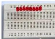
[Arduino Knight Rider](#) In this tutorial, eight LEDs are interfaced to the Arduino Uno board. This is not complicated – it is just like interfacing a single LED to the Arduino as done in tutorial 3, but eight times over. A program is then loaded to the Arduino..... Listed under: [LED Projects](#)
