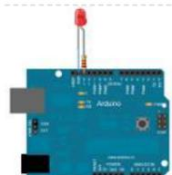
465. [Blink An LED Using Arduino](#) This example shows the simplest thing you can do with an Arduino to see physical output: it blinks an LED. Hardware Required Arduino Board LED Resistor, anything between 220 ohm to 1K ohm Circuit To build the circuit, connect one end of the resistor to..... Listed under: [LED Projects](#)
