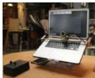
547. [The EyeWriter 2.0](#) The EyeWriter is a low-cost eye-tracking apparatus + custom software that allows graffiti writers and artists with paralysis resulting from Amyotrophic Lateral Sclerosis to draw using only their eyes. The original design, as shown here, featured a pair of glasses as the basis for the..... Listed under: [Development Board – Kits Projects](#)
