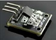
[Temperature Sensor DS18B20 Electronic Brick, Waterproof and other Versions](#) NOTE: There are different-appearing versions but they work the same. This is an electronic thermometer which has high accuracy over a wide range (accurate to  $\pm 0.5^{\circ}\text{C}$  over the range of  $-10^{\circ}\text{C}$  to  $+85^{\circ}\text{C}$ ) (Workable from  $-55^{\circ}\text{C}$  to  $+125^{\circ}\text{C}$ ). You..... Listed under: [Metering – Instrument Projects](#)
