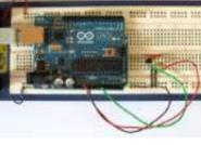
[Tutorial 15: Arduino Serial Thermometer](#) The Arduino reads temperature from a MCP9700 temperature sensor IC and displays the temperature in the Arduino IDE serial monitor window. Also see the Arduino LCD thermometer tutorial (tutorial 14). Prerequisites Complete Tutorial 9: Using the Arduino Serial Port before attempting this tutorial. Components Besides..... Listed under: [Sensor – Transducer – Detector Projects](#)
