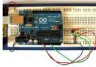
[Arduino Serial Thermometer](#) The Arduino reads temperature from a MCP9700 temperature sensor IC and displays the temperature in the Arduino IDE serial monitor window. Also see the Arduino LCD thermometer tutorial (tutorial 14). Prerequisites Complete Tutorial 9: Using the Arduino Serial Port before attempting this tutorial. Components Besides an Arduino Uno board,..... Listed under: [Metering – Instrument Projects](#)
