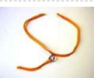
[How to make \(and connect\) a soft potentiometer](#) This instructable will tell you how to make and connect a soft potentiometer to a microcontroller, in particular we will connect it to a LilyPad Arduino. In our case soft potentiometer means a potentiometer made of a textile conductive ribbon. What you need: 1. soft..... Listed under: [Metering – Instrument Projects](#)
