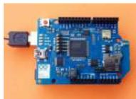
773. [New Arduino WiFi Shield \(Testing\) usign arduino](#) The WiFi Shield was delivered by Amazon. The Arduino UNO Rev 3 was found at RadioShack... First you need to load the last Arduino IDE (Ver 1.0.2) it has the necessary library to use the WiFi shield. Tried the examples "Scan for available networks" and ..... Listed under: [Wifi - Wlan Projects](#)
