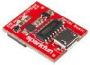
[Serial Basic Hookup Guide](#) Introduction The Serial Basic is an easy to use USB to Serial adapter based on the CH340G IC from WCH. It works with 5V and 3.3V systems and should auto install on most operating systems without the need for additional drivers. It's a great lower..... Listed under: [Other Projects](#)
