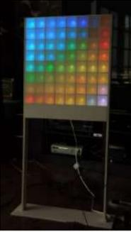
[Lampduino – an 8x8 RGB Floor Lamp using arduino](#) Lampduino is a computer-controlled free-standing floor lamp, comprised of an 8x8 RGB LED matrix. The lamp stands 45" high and 18" wide. Light emanates from both sides. It has various display modes, as well as an included editor for creating animations. The lamp is controlled..... Listed under: [Home Automation Project Ideas](#)
