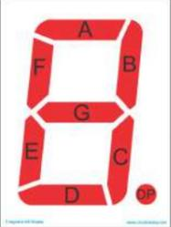
[Arduino and 7 Segment Display – Interfacing Tutorial](#) In this article, we are publishing a tutorial on how to interface seven segment LED display to Arduino. Seven segment displays are used in many embedded system and industrial applications where the range of outputs to be shown is known beforehand. Basic 1 digit seven segment..... Listed under: [LED Projects](#)
