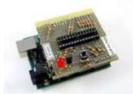
443. [SP0256-AL2 Speech With Arduino](#) Here's the Arduino version of a project to use the General Instruments (GI) SP0256-AL2 vintage speech synthesis chip to say "hello world". I'd previously shown how to do this with a Basic Stamp 2. Here's what it sounds like saying, "hello world" 20101215\_164333.mp3 How it..... Listed under: [Development Board – Kits Projects](#)
