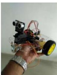
43. [Robot using Arduino and Bluetooth Module \(Obstacle Avoidance Robot\)](#) This project is designed to build a robot that automatically detects the obstacle on its path and guides itself whenever an obstacle comes ahead of it. This robotic vehicle is built, using Arduino UNO board. An ultrasonic sensor is used to detect any obstacle ahead..... Listed under: [Robotics – Automation Projects](#)
