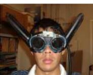
[How To Build Your Own Ultrasonic Batgoggles using an Arduino](#) Wish you were bat? Want to Experience Echolocation? Want to try to "see" with your ears? For my first Instructable, I will show you how to build your own ultrasonic Batgoggles using an Arduino microcontroller clone, Devantech ultrasonic sensor and welding goggles for around \$60..... Listed under: [Game – Entertainment Projects](#)
