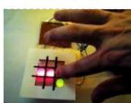
[Arduino and Touchpad Tic Tac Toe using arduino](#) Or, an exercise in input and output multiplexing, and working with bits. And a submission for the Arduino contest. This is an implementation of a tic tac toe game using a 3x3 array of bicolored LEDs for a display, a simple resistive touchpad, and an..... Listed under: [Game – Entertainment Project Ideas](#)
