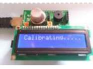
[Smoke Detector using MQ2 Gas Sensor and Arduino](#) Smoke Detectors are very useful in detecting smoke or fire in buildings, and so are the important safety parameters. In this DIY session, we are going to build a Smoke Detector Circuit which not only sense the smoke in the air but also reads and displays the level..... Listed under: [Sensor – Transducer – Detector Projects](#)
