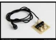
[Camera and flash trigger module using arduino](#) Here we go again, here is a picture of the camera and flash trigger module I made for my arduino photographic projects: It includes three 4N26 optocouplers. One (first one from the left side) to trigger a flash, as I did in the arduino controlled..... Listed under: [Video – Camera – Imaging Projects](#)
