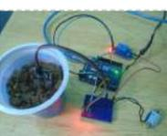
[DIY Soil Testing with Arduino and FC-28 Moisture Sensor](#) In this article, we are going to interface an FC-28 Soil moisture sensor with an Arduino. This sensor measures the volumetric content of water in soil and gives us the moisture level. The sensor gives us both analog and digital output, so it can be used..... Listed under: [Sensor – Transducer – Detector Projects](#)
