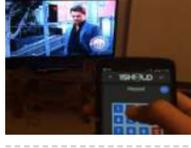
[Universal Remote Control](#) The transmitter in the remote control handset sends out a stream of pulses of infrared light when the user presses a button on the handset. A transmitter is often a light emitting diode (LED) which is built into the pointing end of the remote control..... Listed under: [Other Projects](#)
