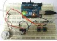
[DC Motor Control using Arduino](#) Here we are going to interface a DC motor to Arduino UNO and its speed is controlled. This is done by PWM (Pulse Width Modulation). This feature is enabled in UNO to get variable voltage over constant voltage. The method of PWM is explained here;..... Listed under: [Motor Projects](#)
