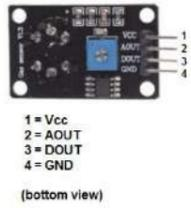
[MQ-8 Hydrogen Gas Sensor Circuit Built with an Arduino](#) In this project, we will go over how to build a hydrogen gas sensor circuit with an arduino. The hydrogen gas sensor we will use is the MQ-8 sensor. This is a sensor that is sensitive to effects of hydrogen gas. Hydrogen gas (H<sub>2</sub>), at..... Listed under: [Sensor – Transducer – Detector Projects](#)
