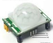
[Interfacing PIR Sensor to Arduino – Connect Motion Sensor/Detector to Arduino](#) In this article, we are going to learn how to interface/connect PIR Sensor or Passive Infrared Sensor to Arduino. We have written a tutorial on how to interface PIR sensor to 8051 previously in CircuitsToday! So a PIR sensor which is also known as Pyroelectric..... Listed under: [Sensor – Transducer – Detector Projects](#)
