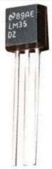
[How to Build a LM35 Temperature Sensor Circuit](#) In this project, we will demonstrate how to build temperature sensor circuit using a LM35 sensor. As a temperature sensor, the circuit will read the temperature of the surrounding environment and relay thi temperature to us back in degrees celsius. The IC we will use..... Listed under: [How To – DIY – Projects](#), [Temperature Measurement Projects](#)
