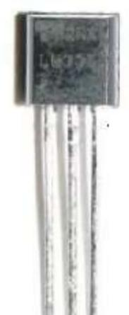
[How to Build a LM335 Temperature Sensor Circuit](#) In this project, we will demonstrate how to build temperature sensor circuit using a LM335 sensor. As a temperature sensor, the circuit will read the temperature of the surrounding environment and relay this temperature to us back in degrees Kelvin. The difference between an LM335..... Listed under: [Sensor – Transducer – Detector Projects](#)
