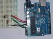
[Arduino UNO Tutorial 8 – NightLight](#) In this Arduino UNO tutorial, we are going to use a Light Dependent Resistor (LDR) to create a simple childrens bedroom nightlight which turns on automatically when it gets dark and turns off when it gets light. An LDR's resistance changes depending upon the amount..... Listed under: [Sensor – Transducer – Detector Projects](#)
