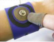
[Time Sensing Bracelet using arduino](#) The Time Sensing Bracelet is a fabric potentiometer. You select your desired time of day by making contact in the corresponding position on your wrist - where your watch would normally be. There is no point to it but fun. Update: Using some wire wrapped..... Listed under: [Sensor – Transducer – Detector Projects](#)
