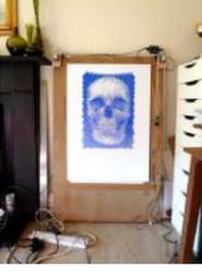
[Polargraph Drawing Machine](#) This machine, a variation on the hanging-pen plotter is a conspicuous and wilfully naive attempt to break out of the pristine, pixel perfect, colour-corrected space that exists inside our computers. It's a drawing machine, that takes a pen (a human tool) and uses it to..... Listed under: [Robotics – Automation Projects](#)
