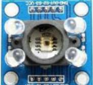
[How to Build a Color Sensor Circuit](#) In this project, we are going to build a color sensor circuit with an Arduino microcontroller. A color sensor is a device that can detect and differentiate between certain primary colors. This sensor can detect and differentiate between the colors white, blue, green, and red..... Listed under: [How To – DIY – Projects](#), [Sensor – Transducer – Detector Projects](#)
