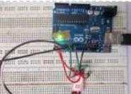
[7 Segment Display Interfacing with Arduino](#) In this tutorial we are going to interface a seven segment display to ARDUINO UNO. The display counts from 0-9 and resets itself to zero. Before going further, let us first discuss about seven segment displays. A seven segment display got its name from the very..... Listed under: [LED Projects](#)
