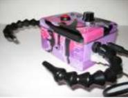
[High-speed Photography with Arduino and CHDK using arduino](#) This project uses an Arduino microcontroller and a laser break-beam trigger to fire via USB remote a Canon camera modified with CHDK (Canon Hack Development Kit) firmware. Immediate influences are the high-speed flash photography triggered by sound or light project by Glacial Wanderer and the..... Listed under: [Video – Camera – Imaging Projects](#)
