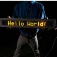
[PS/2/You: Go-anywhere, LED digital message board using Arduino microcontroller](#) Combine three inexpensive LED matrix display panels, an Ardweeny microcontroller and a standard PS/2 computer keyboard into your own go-anywhere, instantly updatable 768-pixel digital message board. The code can hold up to six lines of text with a maximum of 100 characters each. Pressing a..... Listed under: [LED Projects](#)
