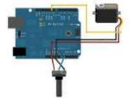
[Arduino Knob](#) Control the position of a RC (hobby) servo motor with your Arduino and a potentiometer. This example makes use of the Arduino servo library. Hardware Required Arduino Board (1) Servo Motor (1) Potentiometer hook-up wire Circuit Servo motors have three wires: power, ground, and signal:..... Listed under: [Motor Projects](#)
