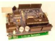
[How to Install the Arduino to the Lithium Backpack using arduino](#) The Arduino is an open source hardware input and output circuit and the Lithium Backpack is a Arduino accessory that will power the Arduino when it is away from a computer or a wall power. These products are sold at Liquidware for under \$34 each..... Listed under: [Interfacing\(USB – RS232 – I2c -ISP\) Projects](#)
