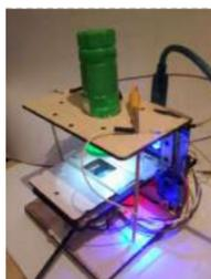
452. [Temperature Sensor v2.0](#) Overview This board allows you to use a thermistor to measure the temperature of something. It is designed to be used to measure things in the range of 100C - 300C, but with the proper calibration and resistors, it can be adapted to any temperature..... Listed under: [Temperature Measurement Projects](#)
