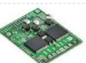
[Pololu Dual VNH5019 Motor Driver Shield for Arduino \(ash02a\)](#) Get your Arduino moving! This shield makes it easy to control two high-power DC motors with your Arduino or Arduino-compatible board. Its dual robust VNH5019 motor drivers operate from 5.5 to 24 V and can deliver a continuous 12 A (30 A peak) per motor, or a continuous..... Listed under: [Motor Projects](#)
