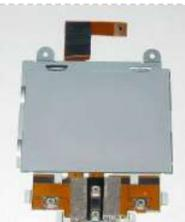
[Arduino + Laptop Touchpad using arduino](#) Yes, this is more or less your average touchpad that one can find from inside a laptop. This model, like majority of touchpads out there operates with PS/2 standard. This means that it can be directly plugged in to a PS/2 connector and with proper..... Listed under: [Sensor – Transducer – Detector Project Ideas](#)
