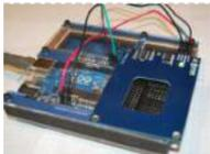
[Using the Parallax RFID Reader with an Arduino](#) f you've ever wanted the ability to use some form of hardware-based authentication in your projects then this is the board to do it with. The Parallax RFID (Radio Frequency Identification) reader is super easy to configure. It only takes four wires! It uses serial..... Listed under: [Projects](#), [RFID - NFC projects](#)
