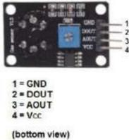
[MQ-7 Carbon Monoxide Sensor Circuit Built with an Arduino](#) In this project, we will go over how to build a carbon monoxide sensor circuit with an Arduino. The carbon monoxide sensor we will use is the MQ-7 sensor. This is a sensor that is sensitive to effects of CO. Carbon monoxide (CO) is a..... Listed under: [Sensor – Transducer – Detector Projects](#)
