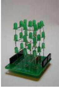
[3x3x3 LED cube shield using arduino](#) What should be in your kit: 1 – PCB 27 – LED's 2 – 6 Pins for Arduino 2 – 8 Pins for Arduino 3 – Resistors 1 – Foam Guide 1 – Small Wire 1 – Medium Wire 1 – Large Wire You will..... Listed under: [LED Projects](#)
