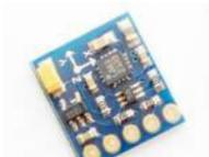
[Arduino + Compass Module 3-Axis HMC5883L](#) Background In this blogpost we're going to deal with the Compass Module 3-Axis HMC5883L from Parallax and how to integrate it into an Arduino. The Compass Module 3-Axis HMC5883L is designed for low-field magnetic sensing with a digital interface. This compact sensor fits into small..... Listed under: [CNC Machines Project Ideas, Robotics – Automation Project Ideas](#)
