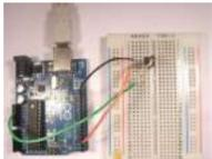
[Arduino – One Wire Digital Temperature Sensor – DS18B20](#) The one wire Digital Temperature Sensor - DS18B20 from Maxim (formerly Dallas) is a great chip for measuring temperature in your projects. Luckily, there is a Dallas Temperature library for the arduino which makes using this sensor very easy. The most recent version of this..... Listed under: [Interfacing\(USB – RS232 – I2c -ISP\) Project Ideas, Temperature Measurement Projects](#)
