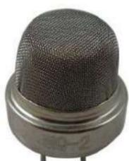
[MQ-2 Smoke Sensor Circuit Built with an Arduino](#) In this project, we will go over how to build a smoke sensor circuit with an arduino board. The smoke sensor we will use is the MQ-2. This is a sensor that is not only sensitive to smoke, but also to flammable gas. The MQ-2..... Listed under: [Sensor – Transducer – Detector Projects](#)
