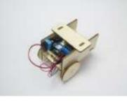
[MKR1000 Robot Controlled Via WiFi Using Arduino](#) This project consists of a small robot controlled via WiFi using an Arduino MKR1000, MKR2UNO Shield Adapter and Arduino Motor Shield! Things used in this project Hardware components Arduino MKR1000 × 1 Arduino MKR2UNO Adapter × 1 Arduino MotorShield Rev3 × 1 Arduino Small DC..... Listed under: [Battery Projects](#), [Robotics – Automation Project Ideas](#)
