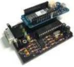
[IoT4Car \(2\)](#) ObdiiUartMkrShield is a socket board for Arduino MKR board to talk with vehicles through OBD-II interface. Things used in this project Hardware components Arduino MKR1000 × 1 OSH Park Custom fabricated PCB × 1 Sparkfun - OBDII to DB9 cable × 1 Software apps and..... Listed under: [Car Projects](#), [Projects](#)
