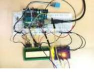
[Temp & Humidity Sensor With LCD Disp & LED Indicator](#) In this instructable, I have used the DHT11 Temperature & Humidity sensor & Arduino UNO to display the current temperature & humidity readings into a 16 x 2 LCD Display. Alongside, I have also created a 3-LED setup which indicates 3 sets of temperature readings (cold, hot, extreme). The DHT11 is a..... Listed under: [LED Projects](#)
