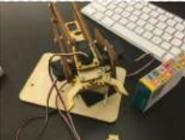
[Handmade Claw](#) These 6 easy steps will tell you how to make a wooden claw machine controlled with Arduino. Step 1: Print All of Your Pieces Either handcut or laser cut all of your pieces Step 2: Aquire Your Parts You will need 4 SG90 servos, 4..... Listed under: [Other Projects](#)
