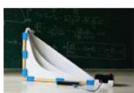
[The Brachistochrone Curve](#) <https://youtu.be/1BdO8J0iynY> The brachistochrone curve is a classic physics problem, that derives the fastest path between two points A and B which are at different elevations. Although this problem might seem simple it offers a counter-intuitive result and thus is fascinating to watch. In this instructables one will..... Listed under: [Other Projects](#)
