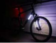
[Light your Bike, and use your Phone to Control It](#) Arduino, NeoPixels, Firmata, and a Windows Phone (picked one up for \$30 bucks) to control lighting. Things used in this project Hardware components Arduino MKR1000 × 1 SparkFun Bluetooth Modem - BlueSMiRF Silver × 1 Adafruit NeoPixel Digital RGB LED Strip - White 30 LED..... Listed under: [LED Projects](#), [Projects](#)
