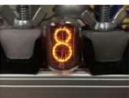
[How to Control a Nixie Tube With an Arduino](#) A Nixie Tube is a Neon gas-filled tube, that has a wiremesh anode with various cathodes shaped like numbers or symbols. Back in the 1950s they were used in computers, calculators, and laboratory equipment. Nixie tubes were replaced by LEDs and VFDs(vacuum fluorescent displays)in the..... Listed under: [Other Projects](#)
