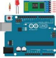
[Arduino Bluetooth Basic Tutorial](#) Ever thought of controlling any electronic devices with your smart phone ?Controlling your robot or any other devices with your smartphone will be really cool. Here is is a simple and basic tutorial for interfacing Bluetooth with arduino Step 1: Things You Need Hardware Bluetooth Module HC 05/06ArduinoLED220Ω ResistorAndroid device..... Listed under: [Bluetooth Projects](#)
