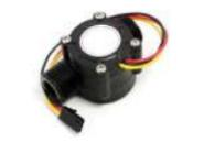
[How to Use Water Flow Sensor – Arduino Tutorial](#) In this tutorial you will learn how to use one water flow sensor with an Arduino board. The water flow sensor consists of a plastic valve body, a water rotor and a hall-effect sensor. When the water flows through the rotor, rotor rolls and the..... Listed under: [Sensor – Transducer – Detector Projects](#)
