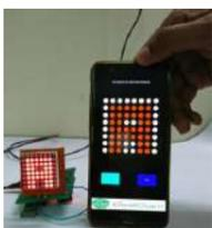
713. [Bluetooth Controlled 8×8 LED Matrix Sign Board Display using Arduino](#) Be it the long stretched highways or your doctors front door, we have sign boards placed everywhere to provide us information. But these sign boards are often boring and cannot be configured as per our interest from time to time. So in this project we..... Listed under: [LED Projects](#)
