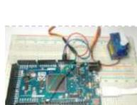
[Servo Motor Control with Arduino Due](#) As discussed earlier, Arduino Due is an ARM controller based board designed for electronic engineers and hobbyists. This DUE board can be used for making CNC machines, 3D printers, robotic arms etc. All these projects have a common feature that is Position Control. Any of..... Listed under: [Arduino Motor Project Ideas](#)
