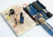
[Interfacing Flame Sensor with Arduino to Build a Fire Alarm System](#) In this article we interface Flame Sensor with Arduino and learn all the steps to build Fire Alarm System by using Arduino and flame sensor. Flame sensor module has photodiode to detect the light and op-amp to control the sensitivity. It is used to detect fire and provide HIGH signal upon..... Listed under: [Sensor – Transducer – Detector Projects](#)
