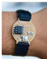
319. [The Nerd Watch](#) Hello! Welcome to another Other Machine project tutorial! I'm Sam DeRose, a former Other Machine Co. Summer Intern. I created the Nerd Watch last summer while working at OMC. The Nerd Watch displays the time in binary when the button is pushed. The watch shows the..... Listed under: [Clock – Timer Projects](#)
