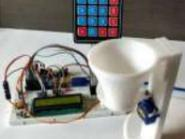
[Automatic Pet Feeder using Arduino](#) Today we are building an Automatic Pet Feeder Using Arduino which can automatically serve food to your pet timely. It has a DS3231 RTC (Real Time Clock) Module, which used to set time and date on which your pet should be given food. So, by..... Listed under: [Clock – Timer Projects](#)
