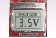
[DIY Voltmeter with Arduino and a Nokia 5110 Display](#) Story In this tutorial I am going to show you how to build a Voltmeter with a big Nokia 5110 LCD display using Arduino. Building a voltmeter is a great learning experience. When you finish building this project, you will have a better understanding of..... Listed under: [Metering – Instrument Projects](#)
