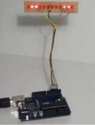
[Charlieplexed row of LED lights, for the Arduino](#) This is my instructable on charlieplexing a LED row/string with the arduino. I noticed that there weren't many instructables on charlieplexing using an arduino, so i made this. I tried to keep the project simple, but that didn't work very well. The soldering is complex,..... Listed under: [Arduino LED Project Ideas, Ideas](#)
