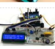
[LC Meter using Arduino: Measuring Inductance and Frequency](#) All embedded lovers are familiar with multimeter which a great tool to measure voltage, current, resistance etc. A multimeter can measure them easily. But sometimes we need to measure inductance and capacitance which is not possible with a normal multimeter. There are some special multimeters..... Listed under: [Metering – Instrument Projects](#)
