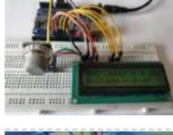
[Measuring PPM from MQ Gas Sensors using Arduino \(MQ-137 Ammonia\)](#) Right from the time of industrial age, we mankind have been rapidly developing. With every progress we also pollute our environment and eventually degrading it. Now global warming is an alarming threat and even the air that we breathe are getting critical. So air quality..... Listed under: [Other Projects](#)
