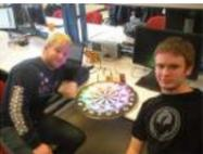
[RGB LED Strip Clock](#) For the final project we made an analog style clock with an Arduino microcontroller. To do this we used three major components: an RGB LED Strip, a DeadOn RTC, and a custom user interface. The LED strip is used to set the display around the..... Listed under: [LED Projects](#)
