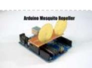
[Arduino Mosquito Repeller](#) In this instructable I'm going to show you how to build a mosquito repeller using an Arduino. The repeller is in the form of a shield that plugs into the Arduino board and the frequency of the repeller can be changed easily. This project is ideal..... Listed under: [Other Projects](#)
