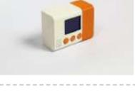
[Smart Thermostat](#) Connect your home heater to Internet and chat with it via Telegram! Things used in this project Hardware components Arduino MKR1000 × 1 DHT22 Temperature Sensor × 1 SparkFun Pushbutton switch 12mm × 3 Resistor 10k ohm × 4 LCD screen × 1 Software apps..... Listed under: [Projects](#), [Temperature Measurement Projects](#)
