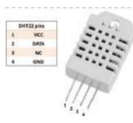
[Temperature and Humidity monitoring with DHT22 sensor Arduino Uno R3](#) The objective of this tutorial is to learn how to use the DHT22 sensor with Arduino uno. The room temperature and humidity will be printed to serial monitor and also will be displayed to the LCD 4x20 in Proteus ISIS. [caption id="attachment\_28379" align="aligncenter" width="300"] DHT22..... Listed under: [Temperature Measurement Projects](#)
