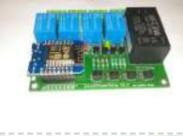
[Smart Power Strip With Cayenne Cloud](#) <https://youtu.be/uXSMAoU3B6Y> This instructable shows how you can build your own easy or simple DIY Internet-connected Smart Power Strip to control Electrical Appliances from remotely.You can also automate the daily repetitive task with scheduling feature, so the appliance will automatically be turned on and off on..... Listed under: [Other Projects](#)
