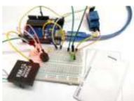
710. [Arduino RFID Door Lock](#) You have seen RFID Door Lock Mechanism in some Hotels and other places, where you don't need a key to unlock the room. You are given a card and you just need to put it in front of a RFID Reader box, and the lock gets unlocked..... Listed under: [Security – Safety Projects](#)
