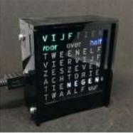
[Dutch 8x8 Word Clock](#) I know that I am not the first to make a word clock, using an Arduino. Still it was always something on my 'to do' list to make a Dutch one. For a different project I've bought a 'colorduino / rainbowduino / funduino' a long..... Listed under: [Clock – Timer Projects](#)
