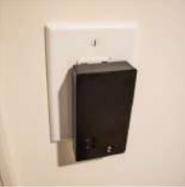
[The Ultimate Light Switch](#) The goal of this instructable is to explain how I made a wifi-connected light switch (also called remotes further). The goal of these remotes is to turn on and off several wifi-connected relays. The relays are not explained in this instructable. They are explained in..... Listed under: [LED Projects](#)
