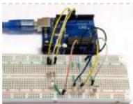
703. [Arduino Color Mixing Lamp using RGB LED and LDR](#) What if we can generate different colors using a single RGB led and make our room's corner more attractive? So, here is a simple Arduino based color mixing lamp which can change color when there is change in light in the room. So this lamp..... Listed under: [LED Projects](#)
