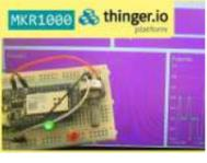
[Arduino MKR1000 & Thinger](#) A simple Internet of Things experiment, using an Arduino MKR1000 board to control two LEDs and monitor a potentiometer, via Thinger.io. Things used in this project Hardware components Arduino MKR1000 × 1 LED (generic) × 2 Rotary potentiometer (generic) × 1 Breadboard (generic) × 1..... Listed under: [Internet – Ethernet – LAN Projects](#), [LED Projects](#)
