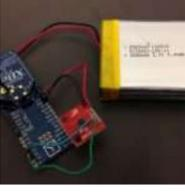
[Magnetometer Parking Sensor](#) The objective of our project was to develop a wireless sensor device to be used for detecting motor vehicles, along with their direction of travel. The sensor is to be used in a larger system to monitor parking lot traffic by counting ins and outs..... Listed under: [Sensor – Transducer – Detector Projects](#)
