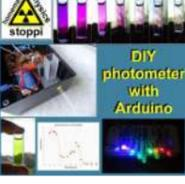
[DIY LED-photometer With Arduino for Physics or Chemistry Lessons](#) Liquids or other objects appear colored because they reflect or transmit certain colors and in turn swallow (absorb) others. With a so-called photometer, those colors (wavelengths) can be determined, which are absorbed by liquids. The basic principle is simple: with a LED of a certain color..... Listed under: [LED Projects](#)
