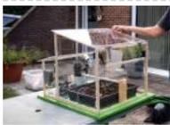
229. [Automated Greenhouse](#) We decided to design a greenhouse as subject for our electronic project. The goal was to regulate the temperature inside the greenhouse thanks a lamp, a servomotor to open a window and a PC fan. We wanted to maintain a quite constant level of soil..... Listed under: [Home Automation Projects](#)
