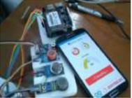
[Indoor Air Quality Monitoring System](#) An indoor air quality monitoring system for detecting toxic gases. Things used in this project Hardware components Arduino Yun Shield & Genuino Yun Shield × 1 Arduino Leonardo × 1 Arduino Yun × 1 Arduino MKR GSM 1400 × 1 Arduino MKR WAN 1300 ×..... Listed under: [Sensor – Transducer – Detector Projects](#)
