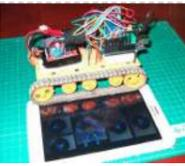
[Tracked Robot Bluetooth Controlled by Arduino Via Android Application](#) <https://youtu.be/J3DwgZvD2js> After trying to remote track a robot by IR remote control, I have proceeded to control the same robot platform by Bluetooth Arduino controller via Android application. This method is more reliable, longer distance, pretty Android application enhancement. Same principle, low cost play and home level technical skill. Programming knowledge is not..... Listed under: [Bluetooth Projects](#)
