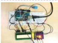
228. [Temp & Humidity Sensor With LCD Disp & LED Indicator](#) In this instructable, I have used the DHT11 Temperature & Humidity sensor & Arduino UNO to display the current temperature & humidity readings into a 16 x 2 LCD Display. Alongside, I have also created a 3-LED setup which indicates 3 sets of temperature readings (cold, hot, extreme). The DHT11 is a..... Listed under: [LED Projects](#)
