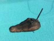
[Crocodile Solar Pool Sensor](#) This instructable shows how to build a rather special pool sensor measuring the pool temperature and transmitting it via WiFi to Blynk App and to a MQTT broker. I call it the "Crocodile Solar Pool Sensor".It uses the Arduino programming environment and an ESP8266 board (Wemos..... Listed under: [Solar energy projects](#)
