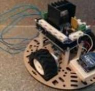
[Remote Controlled Robot](#) The purpose of this final project was to create a small mobile robot and control it via a wireless controller. To accomplish our goal, we decided to use the Arduino Uno microcontroller as the base for both the controller and robot. For the wireless functionality..... Listed under: [Robotics – Automation Projects](#)
