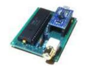
[Arduino MIDI Chiptune Synthesizer](#) Relive the fun of early computer game music with an authentic 8-bit chiptune synthesizer, which you can control over MIDI from the comfort of any modern DAW software. This simple circuit uses an Arduino to drive an AY-3-8910 programmable sound generator chip (or one of its many..... Listed under: [Interfacing\(USB – RS232 – I2c -ISP\) Projects](#)
