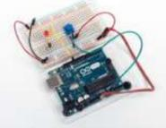
[Read a Potentiometer With Arduino's Analog Input](#) <https://youtu.be/-EDYMQ9IczA> Let's learn how to read a potentiometer, a type of rotating variable resistor, using Arduino's analog input! We'll connect up a simple circuit using a solderless breadboard and use some simple Arduino code to control a single LED. So far you've learned to control LEDs..... Listed under: [Other Projects](#)
