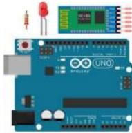
[Arduino Bluetooth Basic Tutorial](#) Ever thought of controlling any electronic devices with your smart phone ?Controlling your robot or any other devices with your smartphone will be really cool. Here is a simple and basic tutorial for interfacing Bluetooth with arduino Step 1: Things You Need Hardware Bluetooth Module HC 05/06ArduinoLED220Ω ResistorAndroid device..... Listed under: [Bluetooth Projects](#)
