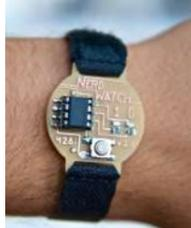
[The Nerd Watch](#) Hello! Welcome to another Other Machine project tutorial! I'm Sam DeRose, a former Other Machine Co. Summer Intern. I created the Nerd Watch last summer while working at OMC. The Nerd Watch displays the time in binary when the button is pushed. The watch shows the..... Listed under: [Clock – Timer Projects](#)
