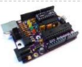
[DIY Arduino-Compatible Clone](#) The Arduino is the ultimate tool in the Maker's arsenal. You should be able to build your own! In the early days of the project, circa 2005, the design was all through-hole parts and communication was via a RS232 serial cable. The files are still available, so you can..... Listed under: [Interfacing\(USB – RS232 – I2c -ISP\) Project Ideas](#)
