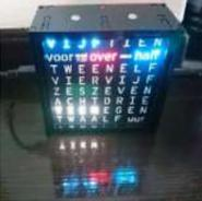
[Dutch 8x8 Neopixel Word Clock](#) A friend introduced me to neopixels (WS2812) programmable LED's. That would be great for my word clock, so I re-did the clock. It is very much a mixup with a slightly different size and code. The 8x8 WS2812 modules are also cheaper than the colorduino,..... Listed under: [Clock – Timer Projects](#)
