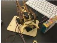
223. [Handmade Claw](#) These 6 easy steps will tell you how to make a wooden claw machine controlled with Arduino. Step 1: Print All of Your Pieces Either handcut or laser cut all of your pieces Step 2: Acquire Your Parts You will need 4 SG90 servos, 4..... Listed under: [Other Projects](#)
