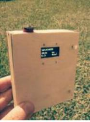
[Portable Luxmeter](#) This project is about making portable luxmeter. It can be used in schools, where children can measure different kinds of light sources.Functions: 1. measure intensity of light in lux. 2. calculate solar irradiation from lux to watts/m2 (factor 112) 3. charging battery using USB port..... Listed under: [Battery Projects](#)
