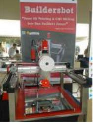
[Arduino Controlled CNC / 3D Printer Hybrid](#) The objective of this instructable is to guide your way throw the entire making process of building a BuildersBot machine. An open design Arduino Controlled CNC Router that can also perform 3D printing. The instructions will cover all areas such as design, mechanics, electronics and..... Listed under: [CNC Machines Projects](#)
