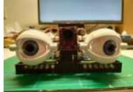
[Motion Follow Animatronics Eyes](#) <https://youtu.be/Ep9fWQiFmoM> This Arduino project uses an Optical Flow Sensor (ADNS3080) to capture movement. Then translate the data to move servo's making it look as eyes are following moving object. This is not an easy build. It requires 3d printing, soldering, some general technical understanding and..... Listed under: [LED Projects](#)
