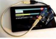
[Nexus 7 and the Arduino.](#) Will show several ways to show how to use an Arduino as a sensor using The Nexus 7 for a terminal and to do development. This can be very important for protecting your electronic equipment especially servers.Note 1: All connections are to a standard Arduino..... Listed under: [Other Projects](#)
