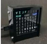
[Dutch 8x8 Word Clock](#) I know that I am not the first to make a word clock, using an Arduino. Still it was always something on my 'to do' list to make a Dutch one. For a different project I've bought a 'colorduino / rainbowduino / funduino' a long..... Listed under: [Clock – Timer Projects](#)
