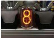
[How to Control a Nixie Tube With an Arduino](#) A Nixie Tube is a Neon gas-filled tube, that has a wiremesh anode with various cathodes shaped like numbers or symbols. Back in the 1950s they were used in computers, calculators, and laboratory equipment. Nixie tubes were replaced by LEDs and VFDs(vacuum fluorescent displays)in the..... Listed under: [Other Projects](#)
