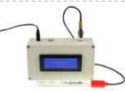
[ARDUINO PH METER](#) In this project, we will be making a benchtop pH meter using the gravity analog pH circuit and probe from Atlas Scientific and an Arduino Uno. Readings will be displayed on a liquid crystal display (LCD). MATERIALS 1 - Arduino Uno 1 - Gravity analog pH sensor..... Listed under: [Other Projects](#)
