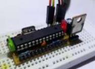
[YABBAS – Yet Another Bare Bones Arduino \(on Stripboard\)](#) This Instructable will demonstrate the building of a bare bones (and really inexpensive... less than \$5) Arduino compatible module that can be put together on a small piece of stripboard and can be used either on a breadboard or independently. The following links / similar..... Listed under: [Development Board – Kits Project Ideas](#)
