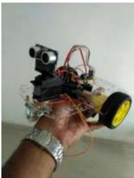
[Robot using Arduino and Bluetooth Module \(Obstacle Avoidance Robot\)](#) This project is designed to build a robot that automatically detects the obstacle on its path and guides itself whenever an obstacle comes ahead of it. This robotic vehicle is built, using Arduino UNO board. An ultrasonic sensor is used to detect any obstacle ahead..... Listed under: [Robotics – Automation Projects](#)
