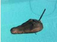
[Crocodile Solar Pool Sensor](#) This instructable shows how to build a rather special pool sensor measuring the pool temperature and transmitting it via WiFi to Blynk App and to a MQTT broker. I call it the "Crocodile Solar Pool Sensor". It uses the Arduino programming
