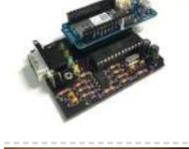
[IoT4Car \(2\)](#) ObdiiUartMkrShield is a socket board for Arduino MKR board to talk with vehicles through OBD-II interface. Things used in this project Hardware components Arduino MKR1000 × 1 OSH Park Custom fabricated PCB × 1 Sparkfun - OBDII to DB9 cable × 1 Software apps and..... Listed under: [Car Projects](#), [Projects](#)
