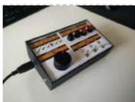
276. [Arduino Type K Temperature Indicator](#) There are lots of Arduino projects to read temperature with different devices, this is an easy one to measure high temperatures with type K thermocouples (1300°C).Skills necessary for this project are basic (buying max IC already mounted) but I have mount an MAX31855 in a..... Listed under: [Temperature Measurement Projects](#)
