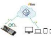
[Secure IOT With AWS and Hornbill ESP32 Using Arduino.](#) Security of connected devices is of paramount concern. There are several possible ways to make the devices secure. One of the most essential and widely used options is to use end to end encryption. The widely used Transport Layer Security (TLS) version 1.2 is the..... Listed under: [Other Projects](#)
