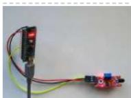
[Arduino Nano: Flame Sensor With Visuino](#) Recently somebody asked for tutorial on Infrared Flame Sensor. It took a while due to severe work overload, but finally I succeeded to make it. The Infrared flame sensors use infrared light to detect flame. While experimenting with my one I discovered that in direct..... Listed under: [Sensor – Transducer – Detector Projects](#)
