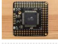
[DIY Bare Minimum Arduino Mega 2560](#) [2017 Update] Eagle files please click here. The objective of this project is to create a version of Arduino Mega 2560 board that has lower component count and smaller board size. Personally to be used for robotics projects that require ATmega2560's 256 KB flash and digital/analog..... Listed under: [LED Projects](#)
