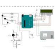
[Home Automation using Arduino and GSM Module](#) In this article, we are publishing a highly useful home application – GSM based home automation using Arduino. The project consists of a 16x2 LCD module for displaying the status of the home appliances. The status (turn ON or turn OFF) of the connected devices can..... Listed under: [Home Automation Projects](#)
