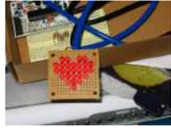
[Arduino Charliplexed Heart, Just in Time for Valentines Day.](#) Here is an Arduino controlled Charliplexed LED heart just in time for Valentine's Day. It uses a total of 6 wires to controll the 27 LEDs. A PIC or AVR could easily be used for this, but I have Arduinos lying around and they are..... Listed under: [LED Projects](#)
