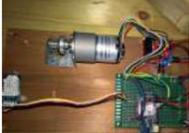
[Chicken Coop Automation](#) Automating a chicken coop with sensors and actors, using an Arduino MKR1000 and the Blynk internet dashboard. Things used in this project Hardware components Arduino MKR1000 × 1 CHIHAI DC Motor - 12V 200rpm Encoder with Mounting Bracket × 1 Geekcreit L298N Dual H Bridge..... Listed under: [Home Automation Projects](#), [Projects](#)
