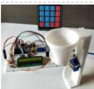
[Automatic Pet Feeder using Arduino](#) Today we are building an Automatic Pet Feeder Using Arduino which can automatically serve food to your pet timely. It has a DS3231 RTC (Real Time Clock) Module, which used to set time and date on which your pet should be given food. So, by..... Listed under: [Clock – Timer Projects](#)
