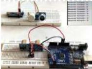
[How To Measure Distance Between Two Ultrasonic Sensors](#) Ultrasonic sensor (HC-SR04) is commonly used to find the distance of an object from one particular point. It has been fairly easy to do this with the Arduino and the code is also pretty simple. But in this article we are going to try something..... Listed under: [Calculator Projects](#), [Metering – Instrument Projects](#)
