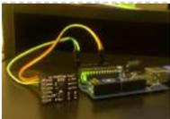
[MCP9802 temperature sensor and Arduino](#) MCP9802 is a digital temperature sensor from Microchip that measures temperatures between -55°C and +125°C to a digital word. It provides an accuracy of ±1°C (maximum) from -10°C to +85°C. The MCP9802 sensor comes with user-programmable registers that provide flexibility for temperature sensing applications. The..... Listed under: [Sensor – Transducer – Detector Projects](#)
