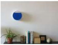
[Tidal Clock](#) This is a tutorial for making the Tidal Clock. The clock shows the ebb and flow between high and low tide by a rising and falling water level. It consists of an airtight acrylic container that has a front visible chamber and a back hidden..... Listed under: [Clock – Timer Projects](#)
