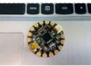
[How to Use the Adafruit Flora Board – Arduino Tutorial](#) In this tutorial you will learn how to use the Adafruit Flora board and how you can easily program it with Codebender! FLORA is Adafruit's fully-featured wearable electronics platform. It's a round, sewable, Arduino-compatible microcontroller designed to empower amazing wearables projects. The FLORA family also..... Listed under: [LED Projects](#)
