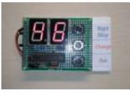
[Arduino Countdown Timer With Setup Buttons](#) In this Instructables guide I will show you how to make your own Arduino two digit countdown timer. I made my own circuit by using the ATmega328 micro controller but this is an optional step. In this guide I will help you to make it..... Listed under: [Other Projects](#)
