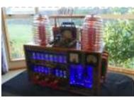
[SteamPunk Radio](#) This project is without doubt the most complex I have undertaken, with sixteen IV-11 VFD tubes, two Arduino Mega cards, ten LED Neon light circuits, a servo, an electromagnet, two MAX6921AWI IC Chips, five DC power supplies, a HV power supply, two DC Volt meters,..... Listed under: [Radio Projects](#)
