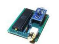
[Arduino MIDI Chiptune Synthesizer](#) Relive the fun of early computer game music with an authentic 8-bit chiptune synthesizer, which you can control over MIDI from the comfort of any modern DAW software. This simple circuit uses an Arduino to drive an AY-3-8910 programmable sound generator chip (or one of its many..... Listed under: [Interfacing\(USB – RS232 – I2c -ISP\) Projects](#)
