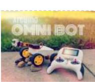
[Arduino RC Robot](#) <https://youtu.be/ytwDgwwSEc0> Description A durable, 3D printed, remote controlled Arduino based robot with several hundred meters range. A modular quick-connect motor scheme lets you rapidly prototype different robot designs without any tools. Perfect for robotics education for kids. Whats it all about? So you've just started..... Listed under: [Robotics – Automation Projects](#)
