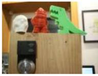
322. [RFID Door Unlock](#) Forgot your keys? Unlock the door using an RFID combination sequence from hidden tags. Things used in this project Hardware components Arduino MKR1000 × 1 Adafruit Metro Mini × 1 Adafruit Lockitron × 1 RFID reader (generic) I used a RFID-RC522 from ebay × 1..... Listed under: [Home Automation Projects](#), [Projects](#)
