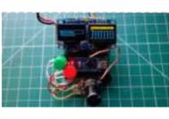
[ArduMeter: an Arduino Based Multimeter \(Sort Of\)](#) The ArduMeter is an Arduino Based Multimeter, which many people have made to perform different operations, and searching on google you could find all the variety of things it can do. I wanted to make one that is portable, quite easy to use, give decent..... Listed under: [Metering – Instrument Projects](#)
