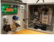
[Card Reading Shop Power Switch](#) This box reads any card with a magnet strip and, if you're on the registered personnel list, turn on the shop power via a relay. A sole person, to be added to the program file upon creation, has the power to add others to this..... Listed under: [Other Projects](#)
