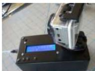
730. [Timelapse Panning controller for GoPro Cameras](#) This instructible will show you how I built (and you can also build) an Arduino Timelapse Panning controller for GoPro cameras. There are obviously some refinements that can be made to the design, but in general I am very happy with the results that I've..... Listed under: [Video – Camera – Imaging Projects](#)
