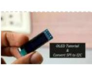
[OLED Tutorial | Convert SPI to I2C](#) In this tutorial, we are going to learn about OLED displays. Which can be very easily interfaced with Arduino and can display important parameters for your project, and see how to convert these screens from SPI to I2C, So let's get started! Step 1: Watch..... Listed under: [LED Projects](#)
