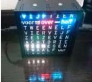
[Dutch 8x8 Neopixel Word Clock](#) A friend introduced me to neopixels (WS2812) programmable LED's. That would be great for my word clock, so I re-did the clock. It is very much a mixup with a slightly different size and code. The 8x8 WS2812 modules are also cheaper than the colorduino,..... Listed under: [Clock – Timer Projects](#)
