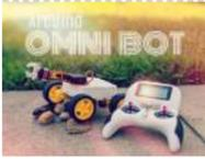
897. [Arduino RC Robot](#) <https://youtu.be/ytwDgwwSEc0> Description A durable, 3D printed, remote controlled Arduino based robot with several hundred meters range. A modular quick-connect motor scheme lets you rapidly prototype different robot designs without any tools. Perfect for robotics education for kids. Whats it all about? So you've just started..... Listed under: [Robotics – Automation Projects](#)
