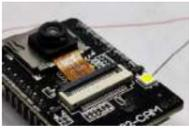
[ESP32 CAM WEB Server and Getting Started Guide](#) This Instructables is all about setting up ESP32 CAM Webserver. The goal here is to connect ESP32 CAM with FTDI Module and program it with the CAM WEB SERVER sketch which will allow us to monitor the camera feed via a web app. The Next..... Listed under: [Video – Camera – Imaging Projects](#)
