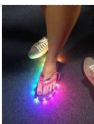
[Slipper Shining with LED strip & Xadow](#) mo.momi Led strips are amazing! Firewalker-led-sneakers(<http://learn.adafruit.com/firewalker-led-sneakers>) by Adafruit inspired me. I wanna change a way to control it, instead of "pressure-sensitive", I use an accelerometer sensor judging the motion of slipper. It's simple, I complete this version only calculating the acceleration on "z" axis, weather..... Listed under: [LED Projects](#)
