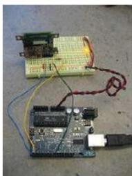
124. [ARDUINO AIRGUN CHRONOGRAPH](#) This is a chrono for measuring the speed and energy of an air rifle pellet. It's pretty fast and could probably be used for other types of gun, (airsoft , full bore etc) but I have not tested it on them. I initially made this..... Listed under: [Temperature Measurement Projects](#)
