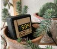
[CO2 Display](#) As its name suggests, the CO2 Display project is a small CO2 gas sensor to be plugged into USB to easily track indoor and outdoor pollution. The CO2 level is displayed live, but it is possible with the small application provided in the documentation to generate..... Listed under: [Sensor – Transducer – Detector Projects](#)
