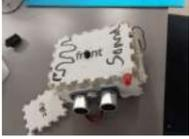
[Ultrasonic Theremin \(Teach Sound\)](#) <https://youtu.be/i9N0bSRXOZ8> The Ultrasonic Theremin is an Arduino project that uses a cheap theremin to teach sound waves. By changing the distance of my hand to the device, I am changing the frequency of the sound waves. Also, moving a potentiometer changes the amplitude of the..... Listed under: [Sound – Audio Project Ideas](#)
