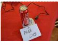
[The useless alarmed Coke can using Arduino](#) Hi all! This is the most useless project in the world! It consist in a Coke can attached to an Arduino trough a coaxial cable and two resistors that make a sound when an hand is near it. Step 1: Materials and Tools For make..... Listed under: [Game – Entertainment Projects, Projects](#)
