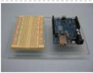
[Acrylic Arduino Prototyping Stand](#) I do a lot of projects with Arduino's and breadboards. Often as I work on a messy workbench, the Arduino or breadboard get jostled and the wires pop out of the headers or the breadboard. To solve this problem, I decided to make a simple..... Listed under: [Ideas, Interfacing\(USB – RS232 – I2c -ISP\) Project Ideas](#)
