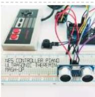
[NES Controller Piano / Ultrasonic Theremin Mash-Up](#) I recently built a simple 8 key piano using an original NES controller and Arduino UNO board. Unlike conventional Arduino piano projects which require one digital pin for each key / button the NES controller piano used only three digital pins (D5 for nesClock, D6 for nesLatch, D7..... Listed under: [Sound – Audio Projects](#)
