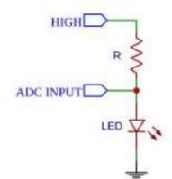
592. [An LED You Can Blow Out Like a Candle!](#) LEDs are designed to emit light, but they also make surprisingly capable sensors. Using only an Arduino UNO, an LED and a resistor, we will build a hot LED anemometer that measures wind speed, and turns off the LED for 2 seconds when it detects..... Listed under: [LED Projects](#)
