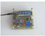
[Timer With TM1637 and Arduino](#) This timer is useful in both domestic and industrial applications. It is a countdown timer programmable in the range of 1s .... 9999s. During this time, the load is powered by a relay on the board. For repeated timings, it is possible to memorize the..... Listed under: [Clock – Timer Projects](#)
