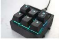
[Custom Macro Mechanical Keypad](#) In this Instructable I will be taking you through the basics of creating your own 6 keyed macropad, controlled by an Arduino. I will be taking you through what you need, how to assemble it, how to program it, and how to improve it or..... Listed under: [Other Projects](#)
