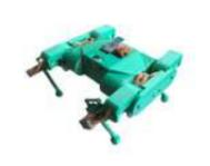
[Ez Arduino 12 DOF Quadruped Robot – Robot Dog Lassie](#) Since Boston Dynamics releases the quadruped robot - Spot, making robot dog has been very popular. There are number of attempts to build similar robot. Most are expensive and very difficult to follow and to make one. This instructable is trying to deliver a DIY..... Listed under: [Robotics – Automation Projects](#)
