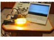
[Dimmer using an Arduino](#) This example shows how to send data from a personal computer to an Arduino board to control the brightness of an LED. The data is sent in individual bytes, each of which ranges in value from 0 to 255. Arduino reads these bytes and uses..... Listed under: [LED Projects](#), [Projects](#)
