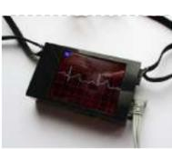
[ECG Display With Arduino](#) This ECG (Electrocardiogram) unit has an integrated display. The display can show individual heart beats in a large format, the train of heart beats in a small format and a Poincaré plot. It is battery powered and can be worn round your neck on a lanyard. It..... Listed under: [Other Projects](#)
