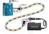
[Arduino Sketch WS2801LED](#) This sketch is used by Exercise: WS2801 RGB LED SPI Module. Full Source Code The full code is all in one file WS2801LED.ino. // \*- mode:c+; \*- /// @file WS2801LED.ino /// /// @brief Example for driving several WS2801 RGB LED modules over SPI on an Arduino UNO..... Listed under: [LED Projects](#)
