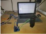
[DIY Programming Cable Using Arduino Uno – Baofeng UV-9R Plus](#) Hey Everyone, this is a simple guide on how to convert your Baofeng UV-9R (or plus) Headphone / ear piece cable into a programming cable using an Arduino UNO as a USB Serial Converter. [DISCLAIMER] I do not take any responsibility in any damage caused..... Listed under: [How To – DIY – Projects](#)
