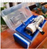
[Measuring Refrigerant Gases Sound Speed Using Arduino and App Inventor 2](#) The purpose of this Instructable is to build a portable device that can measure the speed of sound in refrigerant gases and use this data to identify them. The speed of sound in an ideal gas is related to two characteristics of the gaseous substance, its molecular..... Listed under: [Sound – Audio Projects](#)
