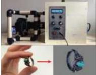
[Desktop CT and 3D Scanner With Arduino](#) Computed tomography (CT) or computed axial tomography (CAT) is most often associated with imaging the body because it enables clinicians to see the anatomical structure inside the patient without having to do any surgery. To image inside the human body, a CT scanner requires X-rays..... Listed under: [Other Projects](#)
