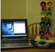
[Arduino Controlled Bell Tower or Carillon](#) This is a set of musical bells which are driven by solenoids and controlled by an Arduino microcontroller. There are 8 bells covering one octave. The bells are controllable from a PC, or the tower can stand alone and play pre-programmed melodies. Check out the..... Listed under: [Ideas, Sound – Audio Project Ideas](#)
