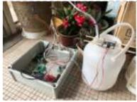
156. [Automatic Irrigation System \(Arduino\) With Usb Type DC Submersible Water Pump](#) This mini project is involved to use Arduino to control submersible water pump when soil reach below or above predefined moisture level. How it works ? 1. Soil moisture sensor is reading analog signal which transmit to Arduino. 2. Arduino control submersible water pump ON..... Listed under: [Interfacing\(USB – RS232 – I2c -ISP\) Projects](#)
