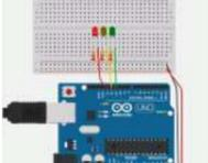
[Multiple LEDs & Breadboards With Arduino in Tinkercad](#) <https://youtu.be/MojSo7OtF9w> Let's learn how to control multiple LEDs using Arduino's digital outputs and a breadboard. Expanding upon the last lesson on blinking an LED, We'll connect some LEDs to the Arduino Uno and compose a simple program to light them up in a pattern. You can..... Listed under: [LED Projects](#)
