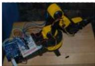
[Modifying a Robot Arm using Arduino](#) Essentially another tutorial involving controlling DC motors. In this post I'm going to first alter a robot arm I had built previously from a beginners kit so that it can be controlled from Arduino. Then I'm going to write a series of posts on different..... Listed under: [Projects, Robotics – Automation Projects](#)
