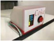
[Coke Machine Can Level Detector](#) Rev 2.5 - tidied up the 3D printed parts and updated the plug connector to a common PCB unit. Rev 2 - ultrasonic "button" replaces manual push-button. Pushing a button is so old fashion, particularly when I'm already using an Ultrasonic sensor. Why not use..... Listed under: [CNC Machines Projects](#)
