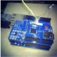
[Sending and Receiving String via UDP using Arduino](#) In this example, you will use your Ethernet Shield and your Arduino to send and receive text strings via the UDP protocol (Universal Datagram Packet). You'll need another device to send to and from. The Processing sketch included at the end of the code will..... Listed under: [Internet – Ethernet – LAN Projects](#), [Projects](#)
