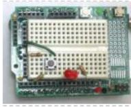
[Physical Pixel using Arduino](#) This example example uses the Arduino board to receive data from the computer. The Arduino boards turns on an LED when it receives the character 'H', and turns off the LED when it receives the character 'L'. The data can be sent from the Arduino..... Listed under: [LED Projects](#), [Projects](#)
