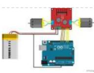
[Arduino Sketch Wheel Drive](#) This sketch is used by Exercise: DRV8833 Dual DC Motor Driver. Full Source Code The full code is all in one file WheelDrive.ino. // WheelDrive - move a pair of DC motors at varying rate and direction // // Copyright (c) 2016, Garth Zeglin. All rights reserved..... Listed under: [Motor Projects](#)
