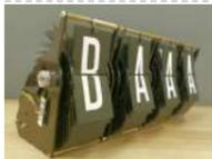
587. [IoT Split-flap Weather Forecast Powered by XOD](#) Hi everyone! In this instructable, I tell you how to make split-flap display and show the current weather conditions on it. Also how to fetch the weather information from the Web using Wi-Fi and API. I am a fan of the XOD visual programming environment. With..... Listed under: [Other Projects](#)
