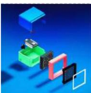
[RGB Box Clock](https://youtu.be/7inXakX4XOs) <https://youtu.be/7inXakX4XOs> This is a clock and decorative RGB Led Matrix It's controlled by a Colorduino Shield and NodeMCU v3 Board using i2C communication. With Blynk app you can setup the alarm,change colors and other things. Parts list is: LoLin V3 NodeMcu Lua CH340G ESP8266 Board..... Listed under: [Clock – Timer Projects](#)
