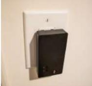
[The Ultimate Light Switch](#) The goal of this instructable is to explain how I made a wifi-connected light switch (also called remotes further). The goal of these remotes is to turn on and off several wifi-connected relays. The relays are not explained in this instructable. They are explained in..... Listed under: [LED Projects](#)
