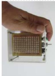
[GYRO & VOICE ARDUIGAMES](#) This gaming box is made from Arduino Uno R3, LoLShield, MPU6050 and Microphone module. With LoLShield, we can show a message/scrolling message or animation picture like: plasma effect, sinewave effect...With MPU6050, we can read value from accelerometer and gyroscope to control movement for simple games..... Listed under: [Game – Entertainment Projects](#)
