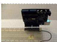
737. [Arduino Bracket](#) When you are tinkering around with your Arduino and a breadboard you might want to make yourself an "Arduino Bracket". Nothing more than header pins and a piece of wire, the "Arduino Bracket" keeps wiring neat and tidy, and lets you easily disconnect your Arduino..... Listed under: [Ideas](#), [Interfacing\(USB – RS232 – I2c -ISP\) Project Ideas](#)
