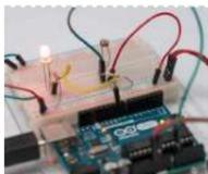
589. [Light Sensor \(Photoresistor\) With Arduino in Tinkercad](#) Let's learn how to read a photoresistor, a light-sensitive type of variable resistor, using Arduino's Analog Input. It's also called an LDR (light-dependent resistor). So far you've already learned to control LEDs with Arduino's analog output, and to read a potentiometer, which is another type of variable..... Listed under: [Sensor – Transducer – Detector Projects](#)
