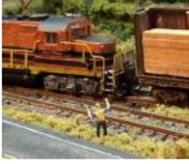
[Wii Nunchuk Controlled Model Train using Arduino](#) Using an Arduino microcontroller, an Adafruit motor shield, and a Wii Nunchuk, you can create a intuitive, programmable, model train controller to run your layout. Amaze your friends. Entertain your kids. Not quite DC, not quite DCC. You're headed for the hacker lands of PWM..... Listed under: [Game – Entertainment Projects, Projects](#)
