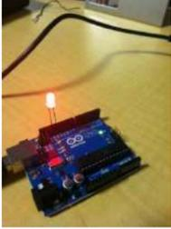
[Blink Without Delay using Arduino](#) Sometimes you need to do two things at once. For example you might want to blink an LED (or some other time-sensitive function) while reading a button press or other input. In this case, you can't use delay(), or you'd stop everything else the program while..... Listed under: [LED Projects](#), [Projects](#)
