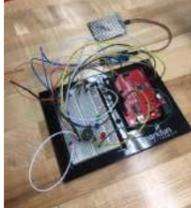
[Using Temperature, Rainwater, and Vibration Sensors on an Arduino to Protect Railways](#) In modern-day society, an increase in rail passengers means that rail companies must do more to optimize networks to keep up with the demand. In this project we will show on a small scale how temperature, rainwater, and vibration sensors on an arduino board can..... Listed under: [Temperature Measurement Projects](#)
