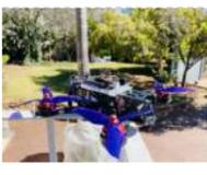
[How to Control Any Drone From Your Arduino Microcontroller Using Bluetooth](#) Hello Everyone!!! In this Instructable I am going to show you how I converted my (Commercial) RC drone that uses an RC radio system into a drone that is controlled by your Arduino using Bluetooth Why would I want to control my drone from an..... Listed under: [Bluetooth Projects](#)
