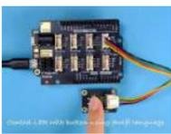
[Control an LED With Button Using Swift Language](#) In the two previous projects, the LED turns on and off automatically. Now, you will control the LED manually using a pushbutton. Step 1: What You Will Need The parts you will need are all included in this Maker kit. SwiftIO boardShieldButton module4-pin cable Step 2:..... Listed under: [LED Projects](#)
