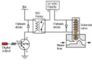
[Wiring of the Solenoid Valves](#) Overview of Wiring for the Salinity Sensor Other pages describing fish tank wiring: Connect electrical power to the pump and the breadboard Connect the salinity sensor to the breadboard and Arduino Connect the solenoids to the cascade control circuit (this page) Return to the main..... Listed under: [Interfacing\(USB – RS232 – I2c -ISP\) Projects](#)
