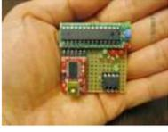
[ATtiny programmer using Arduino ISP](#) Thanks to: <http://jeonlab.wordpress.com/> For relatively small (less number of pins than ATmega328) projects, ATtiny series, ATtiny45 or Attiny85 are good choice in terms of its physical size (8-DIP or 8-SOIC) and low power consumption. There are many ways to program it. One of the popular..... Listed under: [Interfacing\(USB – RS232 – I2c -ISP\) Projects](#), [Projects](#)
