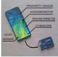
[Sensors in Phone and Arduino Serial Communication](#) Sensors are one of the crucial things when it comes to building projects/robots. Many a times the sensor might be not available locally or it might take too long to ship. Smart phone have most of the basic sensors like proximity, accelerometer, light, magnetometer, gyroscope,..... Listed under: [Sensor – Transducer – Detector Projects](#)
