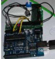
[How To Smell Pollutants using an Arduino](#) This Instructable explains how to use a gas sensor with your Arduino. This lets your Arduino smell (and hence you program responses to) overall gas levels for a variety of nasties, including ethanol, methane, formaldehyde, and a bunch of other volatile organic compounds. My cost..... Listed under: [Projects](#), [Sensor – Transducer – Detector Projects](#)
