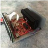
[Arduino Programmable Constant Current Power Resistance Dummy Load](#) Glad to see you have arrived on this page to learn how to build a programmable constant direct current dummy load. This load will allow you to draw a set current from any source. This load can also be set to a constant resistance or..... Listed under: [Arduino Programmer Projects](#)
