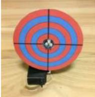
[Laser Shooting Game](#) This laser game is a simple project that utilizes an Arduino mini. All target boards have an Arduino, sensors, and servo control ports. Shooting the target center triggers the servo and the board falls flat. Step 1:What you need [box color="#985D00" bg="#FFF8CB" font="verdana" fontsize="14 "..... Listed under: [Game – Entertainment Projects](#)
