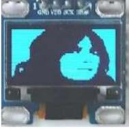
[Display Your Photo on OLED Display](#) The tiny 0.96 inches OLED display is the most popular among the Arduino fraternity for displaying data like room temperature, humidity, and text messages. Have you ever thought of displaying your own photo on the display! Yes, it's possible. In this Arduino-based project, we learn..... Listed under: [LED Projects](#)
