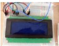
[Arduino LCD Metronome](#) Connecting the LCD The first step is to wire up the LCD. The HD44780 has 16 pins: Pin 1 - Vss Pin 2 - Vdd Pin 3 - Vo Pin 4 - RS Pin 5 - R/W Pin 6 - E Pin 7 - DB0..... Listed under: [LED Projects](#)
