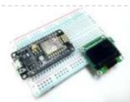
[OLED Interfaced to NodeMCU](#) OLED!! What is an OLED? OLED ( Organic Light Emitting Diodes ) is a flat light emitting technology, made by placing a series of organic thin films between two conductors. When electrical current is applied, a bright light is emitted. OLEDs can be used to make displays and lighting. Because..... Listed under: [LED Projects](#)
