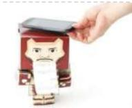
852. [Paper Man: a machine created by Arduino and NFC](#) Paper Man is a machine comprised of Arduino, NFC Shield, thermal printer and a papercraft shell—Iron Man. Thanks to the NFC Shield, you can directly sent messages from your mobile to the paper man, and the paper man will spit it out by printing with..... Listed under: [CNC Machines Projects](#), [Home Automation Projects](#)
