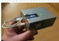
[CO2 Monitoring As an Anti-Covid19 Measure](#) pierre.carles@sorbonne-universite.fr, January 2021 Here, we propose an open-source, portable, autonomous, cheap and easy-to-use device to monitor and record the concentration of CO2 in ambient air in real-time. Using CO2 as a proxy for respiratory aerosols, the device can help define best practices regarding the ventilation..... Listed under: [Temperature Measurement Projects](#)
