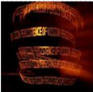
[Persistence of Vision Wand using Arduino](#) Persistence of Vision (POV) Wands are a fun way to create interesting long exposure photographs and light displays. The wand consists of a single row of LEDs controlled by an Arduino Uno. When the wand is turned on it appears to be flickering in a..... Listed under: [Game – Entertainment Projects](#), [Home Automation Projects](#), [Projects](#)
