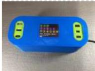
750. [Arduino Cable Tracer](#) Instantly diagnose the type and integrity of USB cables with this Arduino Cable Tracer. Suitable to trace USB A, Mini, Mico, and USB-C cables this is very useful to identify the exact wiring configuration and also diagnose broken connections. Step 1: Gather the Materials and..... Listed under: [Interfacing\(USB – RS232 – I2c –ISP\) Projects](#)
