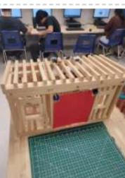
[How to Make a Garage Door \(EASY!!!\)](#) This is a EASY arduino project that you could create to impress your teacher and friends. This project is an IR sensor-controlled garage door. It uses 2 Servo motor's to move the garage door into an opened and closed orientation. The inferred sensor (IR) is effective and..... Listed under: [Other Projects](#)
