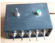
[Analog reading box using an Arduino](#) I made this box for my music project to our school. This is only tutorial for the box, no for playing melody. It's based on serial connected switches. You will need: Some wire 6x switch 1x LED 1x 330 ohm resistor 5x 2000 ohm resistor..... Listed under: [Metering – Instrument Projects](#), [Projects](#)
