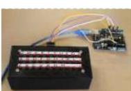
[Shift Register Keyboard for Arduino](#) A common problem that often comes up when working with micro controllers, is running out of IO for all the input the projects requires. So I came up with this solution that allows a user to have up to 4096 button inputs using only 4..... Listed under: [Other Project Ideas](#)
