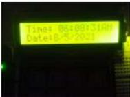
[Digital Clock using Arduino UNO Without RTC module](#) An interesting project of making a Digital Clock using Arduino UNO without the help of RTC Module. Description AIM To build a Digital Clock at Low Cost (Without using any External RTC Module) ject, I have used LCD 16X2 Display , an Arduino UNO ,..... Listed under: [Clock – Timer Projects](#)
