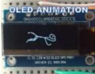
[Create Animation on OLED Display Controlled by Arduino](#) In this tutorial I will show you how to create animation on small OLED display connected to Arduino Nano. Step 1: Supplies We need following two components for this project Arduino NanoSSD1306 SPI 128x32 display You can also use SSD1306SPI 128x32 display but it will..... Listed under: [LED Projects](#)
