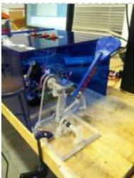
[Katrina And Maya](#) bOunce is a haptics-based learning game system that teaches the concepts behind wave dynamics, and in particular, resonance. The bOunce device (an adaptation of the Haptic Paddle) allows a user to "bounce" a ball in a virtual environment. By feeling the haptic force feedback from..... Listed under: [Robotics – Automation Projects](#)
