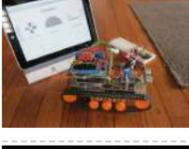
[Tankbot – Internet Controlled Tank Robot using Arduino](#) Do you remember a game called Tank Wars? This is an attempt to make a physical version of that classic arcade game. You, the player drive an Arduino powered tank and fire a laser at a target. This project uses an Arduino to control a tank..... Listed under: [Internet – Ethernet – LAN Projects](#), [Projects](#), [Robotics – Automation Projects](#)
