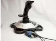
[Arduino Joystick Mouse Control Code](#) Using the Mouse library, you can controls a computer's onscreen cursor with an Arduino Leonardo, Micro, or Due. This particular example uses a pushbutton to turn on and off mouse control with a joystick. Cursor movement from the Arduino is always relative. So every time..... Listed under: [Interfacing\(USB – RS232 – I2c -ISP\) Projects](#), [Projects](#)
