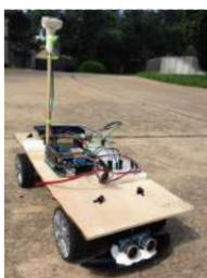
109. [Arduino Powered Autonomous Vehicle](#) A few months back I started playing around with Arduino micro controllers as a learning exercise (and for fun); this project is the culmination of that. The goal of the project was to create a vehicle that can autonomously navigate through a series of waypoints..... Listed under: [Car Projects](#)
