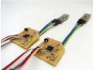
[Bluetooth 4.0 HM-10 cc2541 Duplex](#) In this example, I'll show you how to use the cc2541 to communicate from one microcontroller to another in BOTH DIRECTIONS (BLE-HM-10). <https://youtu.be/6zXYH9arHMI> Introduction The HM-10 is a Bluetooth Low Energy (BLE) module for embedded systems that allows for wireless communication with BLE-capable devices (e.g..... Listed under: [Bluetooth Projects](#)
