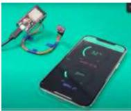
[How to Build a DIY WiFi Smart Oximeter Using MAX30102 and Arduino ESP32](#) This WiFi Smart Oximeter helps you scan Spo2 and BPM using MAX30102 and ESP32 and display the values on the Smartphone Step 1: In this tutorial, I will explain how to build your own WiFi Based Smart Oximeter using MAX30102 and ESP32 in detail. The..... Listed under: [Wifi - WLAN Projects](#)
