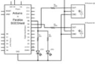
[Connecting an IR Sensor Using Arduino](#) Schematic Since the IR Sensor uses a light sensor, the schematic is very similar to that of the light sensor. The only difference is the addition of an IR LED and that the IR detector requires connection to 5V and ground. Breadboard Setup To setup..... Listed under: [Sensor – Transducer – Detector Projects](#)
