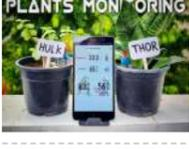
[Avengers plant monitoring device with Arduino uno \(Tuya IoT platform\)](#) I made a lot-based plant monitoring device. From this device, you can measure the condition of your plant from anywhere in the world. The device is able to measure temperature, humidity, and soil moisture. Description <https://youtu.be/cHMHhqCfUgU> I hope you are doing well because a few..... Listed under: [Other Projects](#)
