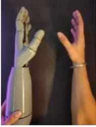
[Cyborg Hand : Robotic-cum-Prosthetic Servo Powered Hand](#) <https://youtu.be/gO7L46sZTY4> Supplies Hey there ! For this Instructable you will need: 1- 3d Printer 2- CAD software( TinkerCad / Fusion360 ) 3- PLA and TPU filament 4- Servos [ MG995 ] 5- Arduino 6- Wires and Breadboard 7- Rubber bands 8- Thread / String (..... Listed under: [Robotics – Automation Project Ideas](#)
