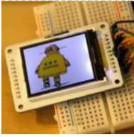
[Your Image on an Arduino! – TFT LCD Screen Guide](#) Have you ever heard of TFT LCD screens? They are great ways to display information from your Arduino, or display pictures. The Arduino team just released an official TFT LCD screen with their new Robot at Maker Faire 2013. It's very easy to get started..... Listed under: [Video – Camera – Imaging Projects](#)
