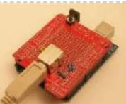
[Virtual USB Keyboard Using Arduino](#) Communicating with a host computer can allow a simple Arduino-based system to gain access to a wide variety of devices and information. Most people link an Arduino to a host using serial communications across a USB connection with custom code running on the host to..... Listed under: [Interfacing\(USB – RS232 – I2c -ISP\) Projects](#), [Projects](#)
