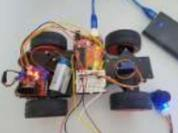
[Joystick Controlled Car](#) I have created a joystick-controlled car, capable of moving left, right, forwards, and backwards. I created this as I thought it would be a challenging project with a fun and exciting purpose. Supplies Arduino Uno R3L293D Motor Control2x DC MotorServo Motor2x 9v Battery (or 1..... Listed under: [Car Projects](#)
