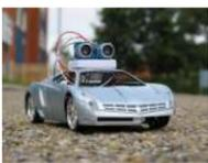
[Autonomous Race Car using Arduino](#) Build this autonomous driving robot car based on a old RC toy car. I removed the radio control board from the car and replaced it with a brain in the form of an Arduino UNO board (plus a motor driver board) and gave it an..... Listed under: [Car Projects](#)
