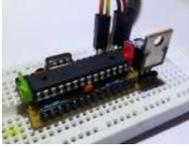
[YABBAS – Yet Another Bare Bones Arduino \(on Stripboard\)](#) This Instructable will demonstrate the building of a bare bones (and really inexpensive... less than \$5) Arduino compatible module that can be put together on a small piece of stripboard and can be used either on a breadboard or independently. The following links / similar..... Listed under: [Development Board – Kits Project Ideas](#)
