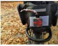
[Bicycle Backlight With Arduino](#) This is the first bicycle accessory gadget I made with Arduino. It's a pattern-based backlight attached to the back-bag mounted on the bicycle luggage compartment. I'm riding an electric bicycle which can speed up around 24km/h at maximum. But I had fallen already three times..... Listed under: [LED Projects](#)
