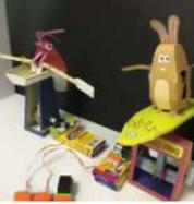
[Papercraft Automata Race Game littleBits Circuit using Arduino](#) This instructable will show you how to create a game using littleBits. The game will start with a sound trigger. Each player will have to press a button repeatedly. The first person to press their button 25 times wins. A buzzer will sound to end..... Listed under: [Game – Entertainment Projects](#)
