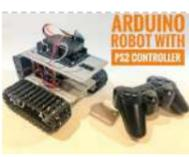
[Arduino Robot With PS2 Controller \(PlayStation 2 Joystick\)](#) In this tutorial, I'll show you how to use a wireless PlayStation 2 (PS2) controller and an Arduino Uno pilot a robotic tank. Story An Arduino Uno board was used at the core of this project. It receives commands from the wireless controller and sets..... Listed under: [Robotics – Automation Project Ideas](#), [Robotics – Automation Projects](#)
