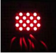
[Using a Dot Matrix LED with an Arduino and Shift Register](#) The Siemens DLO7135 Dot matrix LED is one amazing piece of optoelectronics. It's billed as a 5x7 Dot Matrix Intelligent Display (r) with Memory/Decoder/Driver. Along with that memory, it's got a 96-character ASCII display set with upper and lower case characters, a built-in character generator..... Listed under: [LED Projects](#), [Projects](#)
