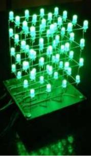
[The 4x4x4 LED cube using an Arduino](#) In this instructable I will show you how to make a 4x4x4 LED cube that will be controlled by an Arduino Demulionove. now yes you might say" that Arduino has only 14 I/O pins well also the 6 analog pins can be used as pins..... Listed under: [LED Projects](#), [Projects](#)
