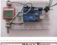
[2-Player Pong Game with Arduino Uno](#) Classical Pong game implemented on an Arduino Uno using a PCD8544 LCD screen which is better known as the Nokia 5110 screen. Player bars are controlled by a potentiometer for each player. If you want the bar to go left, just turn the potentiometer left..... Listed under: [Game – Entertainment Projects](#), [Projects](#)
