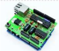
[Low cost Ethernet shield with ENC28J60 using Arduino](#) Economical alternative to original Arduino ethernet shields, allows data rates up to 10 Mbps and is achieved with a traditional assembly components. One of the most interesting shield that you can mount on the Arduino platform is certainly the ethernet shield, because enable numerous networking..... Listed under: [Internet – Ethernet – LAN Projects](#), [Projects](#)
