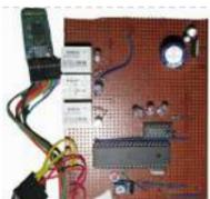
[DIY Cheapest Bluetooth Controlled Home Automation](#) Step 1: COMPONENTS REQUIRED Bluetooth module (HC-05)AT89S52/C51/S51/C52 microcontrollerRelay Driver ULN2003ARelayResistances and capacitors as circuit diagram depicts(below)power module(if the input is more than 5V or else not necessary)IC 7805(5V voltage regulator)1000uF capacitor10uF capacitorled and resistance(as per convenience so that led doesn't get damaged) IMPORTANT NOTE: USE..... Listed under: [Bluetooth Projects](#)
