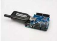
[Network Time Protocol \(NTP\) Client using Arduino](#) In this example, you will use your Ethernet Shield and your Arduino to query a Network Time Protocol (NTP) server. This way, your Arduino can get the time from the Internet. Circuit The Ethernet shield allows you to connect a WizNet Ethernet controller to the..... Listed under: [Internet – Ethernet – LAN Projects](#), [Projects](#)
