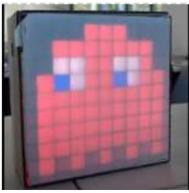
[Pacman/Ghost LED Matrix](#) We created a LED matrix that shows a Pacman and a Ghost. The figure changes by pressing a button. Also, the ghost takes the color according to the external temperature. It means, if it is cold, the figure turn blue, but if it is warm..... Listed under: [Blog](#), [LED Projects](#)
