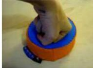
[Analog Fabric Joypad using an Arduino](#) How to make an "analog" input device from fabric and a few other necessary materials. "Analog" in parenthesis because, although it is made up of 4 analog inputs, the only analog transition between the directions (up, right, down and left) comes from the buffering material..... Listed under: [Game – Entertainment Projects, Projects](#)
