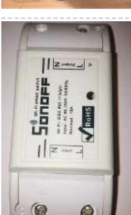
[Hacking a Sonoff to Work With Home-Assistant and MQTT](#) OK So my third Instructable and here we're dealing with another Sonoff device, the original Sonoff WiFi smart switch. Theses devices are again based around the ESP8266 and are easily hacked. The devices can switch up to 10A @ 240V so are ideal for switching..... Listed under: [Home Automation Projects](#)
