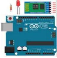
[Arduino Bluetooth Basic Tutorial](#) Ever thought of controlling any electronic devices with your smart phone ?Controlling your robot or any other devices with your smartphone will be really cool. Here is is a simple and basic tutorial for interfacing Bluetooth with arduino Step 1: Things You Need Hardware Bluetooth Module HC 05/06ArduinoLED220Ω ResistorAndroid device..... Listed under: [Bluetooth Projects](#)
