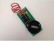
[ATtiny85 EMF Detector](#) Story This is a simple tutorial to create an EMF detector. You can use Arduino for this job, but is better use a microcontroller called Attiny85. It is possible program it throe the Arduino interface. What is a Magnetic Field [from Wikipedia] An electromagnetic field..... Listed under: [Sensor – Transducer – Detector Projects](#)
