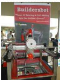
136. [Arduino Controlled CNC / 3D Printer Hybrid](#) The objective of this instructable is to guide your way throw the entire making process of building a BuildersBot machine. An open design Arduino Controlled CNC Router that can also perform 3D printing. The instructions will cover all areas such as design, mechanics, electronics and..... Listed under: [CNC Machines Projects](#)
