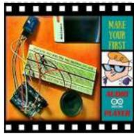
[How to Make an Audio Player with Speaker Using the Arduino Uno!](#) This Arduino project is a simple and fun project you can build in 10-15 minutes. The result of this make will be an Arduino audio player that plays ".wav" files. It consists of a speaker, a simple transistor acting as an amplifier, and a micro-SD card..... Listed under: [Other Projects](#)
