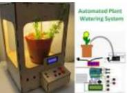
[Automated Plant Watering System](#) House Plant Babysitter Going away from a while? Need something to babysit your house plants?This box will automatically deliver an adjustable volume of water to four plants (or less) every day, or once every "x" day (up to seven days). A micro controller handles the..... Listed under: [Home Automation Projects](#)
