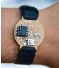
[The Nerd Watch](#) Hello! Welcome to another Other Machine project tutorial! I'm Sam DeRose, a former Other Machine Co. Summer Intern. I created the Nerd Watch last summer while working at OMC. The Nerd Watch displays the time in binary when the button is pushed. The watch shows the..... Listed under: [Clock – Timer Projects](#)
