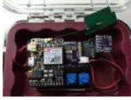
[Cellular Data Logger](#) I have been collecting data from Raleigh's trails and parks for the last couple years. My primary platform has been a custom Arduino board I developed for low-cost (hey, these things may get damaged or stolen) and long battery life. I wanted a connected sensor..... Listed under: [Internet – Ethernet – LAN Projects](#)
