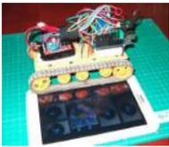
[Tracked Robot Bluetooth Controlled by Arduino Via Android Application](#) <https://youtu.be/J3DwgZvD2js> After trying to remote tracked robot by IR remote control.I have proceed to control same robot platform by Bluetooth Arduino controller via Android application.This method is more reliable,longer distance,pretty Android application enhancement. Same principle,low cost play and home level technical skill.Programming khownledge is not..... Listed under: [Bluetooth Projects](#)
