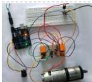
[Arduino DC Motor Speed and Direction Control using Relays and MOSFET](#) In this project we control direction and speed of a 24v high current motor using Arduino and two relays. No power switches are needed for this circuit, just two push buttons and in Potentiometer to control the direction and speed of DC Motor. One push button..... Listed under: [Motor Projects](#)
