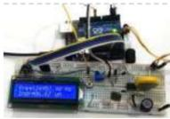
357. [Analog Speedometer Using Arduino and IR Sensor](#) Measuring the speed/rpm of a Vehicle or a motor has always been a fascinating project to try. In this project, we are going to build a Analog Speedometer using the Arduino. We will use IR Sensor module to measure the speed. There are other ways/sensors for..... Listed under: [Sensor – Transducer – Detector Projects](#)
