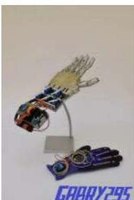
[How to Make a Remote Controlled Robotic Hand With Arduino](#) <https://youtu.be/efO-ooyS-mo> This is my school project for the 5th year of high school (I'm Italian, we have 5 years of high school). It consists in an artificial hand controlled by a glove with flex sensors. The artificial hand reproduces the movements of the hand with..... Listed under: [Robotics – Automation Projects](#)
