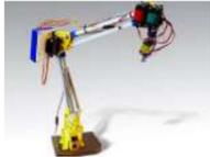
[Tertiarm – 3d Printed Robot Arm](#) This is first version of my low cost 3d printed robot arm. It is based on Ikea Tertial lamp. I choose it because it has very good kinematic with using springs to unload servos. So you can use different number of springs to achive diffrent..... Listed under: [Robotics – Automation Projects](#)
