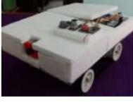
[Teleoperated Robot for Sensing the Toxic Gases](#) Remotely operated ground vehicle for sensing the toxic gases which is helpful for firefighters and researchers. Things used in this project Hardware components Arduino Yun × 1 Arduino MKR1000 × 1 Seeed Grove - Air quality sensor v1.3 × 1 Seeed Grove - Gas Sensor(MQ2)..... Listed under: [Projects](#), [Robotics – Automation Projects](#)
