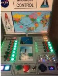
[A Shuttle Mission Control Mock-Up for Kids](#) A Mission Control Center for children was constructed to manage a pretend launch of the space shuttle. I wanted to play-out the make believe mission with nothing but LED lamps to tell the story; both 7-segment displays and graphic displays with LED lights strategically mounted..... Listed under: [Other Projects](#)
