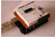
[Arduino Prototyping Shield on the cheap](#) Breadboards are very handy, but sometimes I just want to connect one IC or some LEDs and resistors to the controller. My simple solution was to cannibalize a cheap Breadboard to get two expandable PrototypingShields with some additional features. What I used: Breadboard (~3\$) 2..... Listed under: [Development Board – Kits Project Ideas](#), [Ideas](#)
