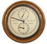
[Arduino Perpetual Calendar Clock](#) The clock uses 2 electro mechanical clock movements controlled by an Arduino to display the Day and Month. A third quartz controlled movement displays the time tide Low or High tide. The Calendar is fully automatic and takes into account leap years as well as..... Listed under: [Clock – Timer Projects](#)
