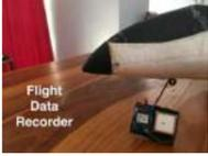
[RC Flight Data Recorder/Black Box](#) In this instructable I am going to be building a arduino based fight data recorder for RC vehicles, specifically RC aeroplanes. I am going to be using a UBlox Neo 6m GPS module connected to an arduino pro mini and a SD card shield to..... Listed under: [Temperature Measurement Projects](#), [Video – Camera – Imaging Projects](#)
