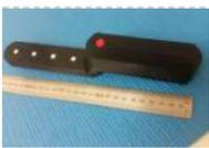
[Pocket Metal Locator – Arduino](#) This cool little Pocket Metal Locator is sensitive enough to identify small nails and tacks in wood and compact enough to fit into awkward spaces making it convenient to carry and use for metal locating. The unit has four independent search coils and color LED..... Listed under: [LED Projects](#)
