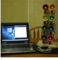
[Arduino Controlled Bell Tower or Carillon](#) This is a set of musical bells which are driven by solenoids and controlled by an Arduino microcontroller. There are 8 bells covering one octave. The bells are controllable from a PC, or the tower can stand alone and play pre-programmed melodies. Check out the..... Listed under: [Ideas, Sound – Audio Project Ideas](#)
