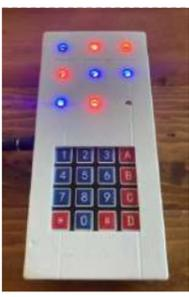
[Neo Pixel Tic Tac Toe \(Arduino Uno\)](#) Tic Tac Toe is a two player game in which the players compete to get 3 pieces in a row. In this project we constructed a Tic Tac Toe game using a number pad and neo pixels as pieces. This results in a portable Tic..... Listed under: [LED Projects](#)
