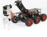
[6WD Shock Absorption Robot for Arduino](#) The new design of the 6WD mobile platform, the vehicle uses 2mm aluminum alloy, aluminum spray surface treatment. 6 high-speed DC motor (original 17000 rpm), with 1:34 full metal gear box, so that the car to obtain strong off-road performance. Shock absorption design is the..... Listed under: [Robotics – Automation Projects](#)
