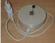
[Gas Detector](#) Let's create a simple Gas Detector connectable to WiFi. The gadget would offer: web UI including gauges for LPG, CO, Smokesimple data handler returning values in JSONcapable of regularly sending data to ThingSpeak server andobviously triggering loud alarm if threshold of dangerous concentrations exceeded. We..... Listed under: [Sensor – Transducer – Detector Projects](#)
