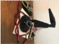
[Robotic Arm Controlled by Glove](#) Purpose: Gain experience, and problem-solving skills by creating a project to complete Outline- Use a glove to connect through an arduino to control a 3-D robotic printed "arm". Each of the joints on the 3-D printed arm has a servo which connects to the flex..... Listed under: [Robotics – Automation Projects](#)
