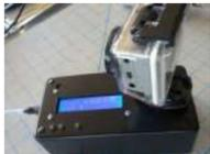
[Timelapse Panning controller for GoPro Cameras](#) This instructible will show you how I built (and you can also build) an Arduino Timelapse Panning controller for GoPro cameras. There are obviously some refinements that can be made to the design, but in general I am very happy with the results that I've..... Listed under: [Video – Camera – Imaging Projects](#)
