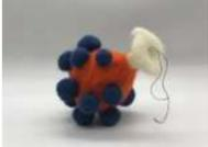
[Needle-Felted Pressure Sensor](#) Create a pressure sensor using: - Needle-felted wool - Thin muslin - Velostat - Conductive thread This sensor can be used an analog input for Arduino code. Step 1: Prepare the Core Components Component 1: A felted wool ball. This can be made using unwoven..... Listed under: [Sensor – Transducer – Detector Project Ideas](#)
