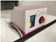
[Coke Machine Can Level Detector](#) Rev 2.5 - tidied up the 3D printed parts and updated the plug connector to a common PCB unit. Rev 2 - ultrasonic "button" replaces manual push-button. Pushing a button is so old fashion, particularly when I'm already using an Ultrasonic sensor. Why not use..... Listed under: [CNC Machines Projects](#)
