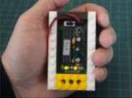
[Palm Arduino Board V3](#) I design and create this Palm Arduino V3 prototype PCB, as I was tired of recreating Arduino Compatible on perf board every time I prototyping a new project, especially when I had to spend a lot of time tracing the wiring to see that I..... Listed under: [Development Board – Kits Projects](#), [Projects](#)
