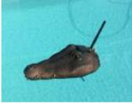
[Crocodile Solar Pool Sensor](#) This instructable shows how to build a rather special pool sensor measuring the pool temperature and transmitting it via WiFi to Blynk App and to a MQTT broker. I call it the "Crocodile Solar Pool Sensor".It uses the Arduino programming environment and an ESP8266 board (Wemos..... Listed under: [Solar energy projects](#)
