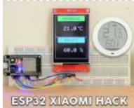
[ESP32 Xiaomi Hack – Get Data Wirelessly](#) Dear friends welcome to another Instructable! Today we are going to learn how to get the data that this Xiaomi Temperature and Humidity monitor transmits using the Bluetooth functionality of the ESP32 board. As you can see, I am using an ESP32 board and a 2.8" color..... Listed under: [Wireless Projects](#)
