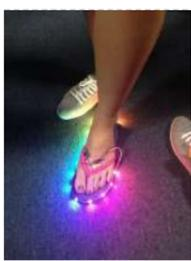
[Slipper Shining with LED strip & Xadow](#) mo.momi Led strips are amazing! Firewalker-led-sneakers(<http://learn.adafruit.com/firewalker-led-sneakers>) by Adafruit inspired me. I wanna change a way to control it, instead of "pressure-sensitive", I use a accelerometer sensor judging the motion of slipper. It's simple, I complete this version only calculating the acceleration on "z" axis, weather..... Listed under: [LED Projects](#)
