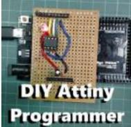
[DIY Attiny Programming Shield](#) If you are looking for a small and low powered Arduino board the Attiny is a really good option, its surprisingly featureful for it's size. It has 5 GPIO pins, 3 of which are Analog pins and 2 which have PWM output. It is also..... Listed under: [Arduino Programmer Projects](#)
