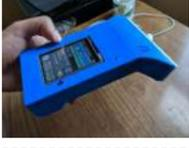
[DIY Geiger Counter With an ESP8266 and a Touchscreen](#) <https://youtu.be/rmFnbVB5gCM> I designed and built a Geiger Counter - a device that can detect ionizing radiation and warn its user of dangerous ambient radiation levels with the all-too-familiar clicking noise. It can also be used when scouting for minerals to see if the rock you..... Listed under: [Other Projects](#)
