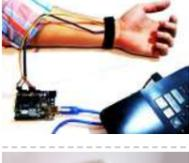
[Arduino Polygraph Machine \(Lie Detector\)](#) In this project, We'll try to get some information from the human body by using simple sensors and Arduino. You can use this information to create a lie detector machine. At the end of this article, you : Know Polygraph and basics of measuring and..... Listed under: [Sensor – Transducer – Detector Projects](#)
