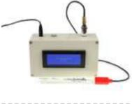
[ARDUINO PH METER](#) In this project, we will be making a benchtop pH meter using the gravity analog pH circuit and probe from Atlas Scientific and an Arduino Uno. Readings will be displayed on a liquid crystal display (LCD). MATERIALS 1 - Arduino Uno1 - Gravity analog pH sensor1 - pH..... Listed under: [Other Projects](#)
