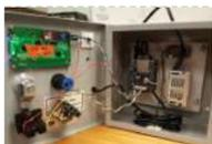
426. [Card Reading Shop Power Switch](#) This box reads any card with a magnet strip and, if you're on the registered personnel list, turn on the shop power via a relay. A sole person, to be added to the program file upon creation, has the power to add others to this..... Listed under: [Other Projects](#)
