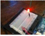
[Basic Arduino Tutorials : 01 Blinking LED](#) In this instructable, I'm going to show you how to make a simple circuit/code with an arduino, which will make an LED connected to it flash from off to on, with 1-second intervals, as shown below. This is a very easy, basic idea, however it..... Listed under: [LED Projects](#)
