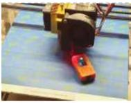
[3D Print Bed Leveling Tool Using M5StickC](#) Do you ever find it a hassle to manually level your 3D print bed every time you make a print? Even seasoned 3D printing pros need to level the printbed after every couple prints. We've created a device that helps tremendously improve this procedure. This..... Listed under: [Other Projects](#)
