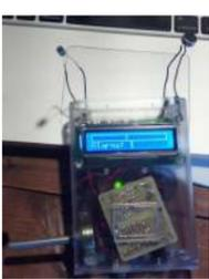
[Arduino Board Sound Alarm](#) I've just completed my second Arduino project, a sound level detector which sets off an "alarm" when there's the sound level is too high for too long. I built it for use in a school that wants to provide visual feedback to students when they..... Listed under: [Projects](#), [Security – Safety Projects](#)
