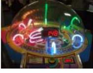
[Arduino Cyclone Reaction Time Game](#) In this instructable, we walk through how I made a "Cyclone" - type arcade game using an Arduino. This game also includes a reaction timer mode. Let's get started! A list of things you will need: Arduino Uno LCD Screen MCP23017 serial port expander 2 pushbuttons LEDs of differing..... Listed under: [Game – Entertainment Projects](#)
