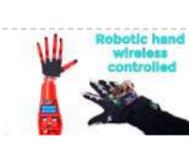
[Robotic Hand With Wireless Glove Controlled | NRF24L01+ | Arduino](#) In this video; 3D robot hand assembly, servo control, flex sensor control, wireless control with nRF24L01, Arduino receiver and transmitter source code are available. In short, in this project we will learn how to control a robot hand with a wireless glove. Step 1: Video..... Listed under: [Robotics – Automation Projects](#)
