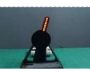
[Persistence of Vision \(PoV\) Display Using Arduino](#) Time for a fun-filled, easy-peasy Japan-easy to make a project! Today, we're going to show you how to make an LED POV Display. POV, an acronym for the persistence of vision, is a kind of optical illusion in which a visual image seems to persist..... Listed under: [LED Projects](#)
