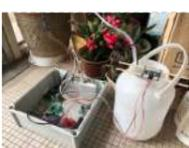
[Automatic Irrigation System \(Arduino\) With Usb Type DC Submersible Water Pump](#) This mini project is involved to use Arduino to control submersible water pump when soil reach below or above predefined moisture level. How it works ? 1. Soil moisture sensor is reading analog signal which transmit to Arduino. 2. Arduino control submersible water pump ON..... Listed under: [Interfacing\(USB – RS232 – I2c -ISP\) Projects](#)
