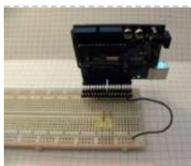
[Arduino Bracket](#) When you are tinkering around with your Arduino and a breadboard you might want to make yourself an "Arduino Bracket". Nothing more than header pins and a piece of wire, the "Arduino Bracket" keeps wiring neat and tidy, and lets you easily disconnect your Arduino..... Listed under: [Ideas](#), [Interfacing\(USB – RS232 – I2c -ISP\) Project Ideas](#)
