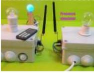
[Home Presence Simulator and Security Control Device](#) This project allow us to simulate presence and to detect movements in our home. We can configure a network of devices installed in differents rooms of our home all of them controlled by a main device. This project combines these features on a single device (PICTURE 1):..... Listed under: [Security – Safety Projects](#)
