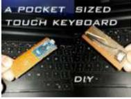
[A Pocket Sized Touch Keyboard](#) In this Instructables I am going to explain about my new project called " A Pocket Sized Touch Keyboard" .It is a Arduino based small physical device used to simplify your different keyboard operations.You plugs it into your computer usb port and touch it on..... Listed under: [Sensor – Transducer – Detector Projects](#)
