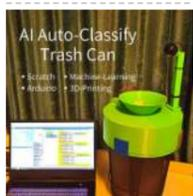
[AI Auto-Classify Trash Can](#) This project is a trash can that recognizes and classifies garbage automatically. Use Machine-Learning and Arduino in Scratch. How it works 1. Camera takes an image of garbage. 2. Machine-Learning model recognizes the classification of garbage by the image. 3. Electrical and mechanical parts drive the garbage..... Listed under: [Other Projects](#)
