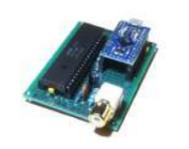
[Arduino MIDI Chiptune Synthesizer](#) Relive the fun of early computer game music with an authentic 8-bit chiptune synthesizer, which you can control over MIDI from the comfort of any modern DAW software. This simple circuit uses an Arduino to drive an AY-3-8910 programmable sound generator chip (or one of its many..... Listed under: [Interfacing\(USB – RS232 – I2c -ISP\) Projects](#)
