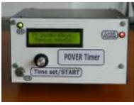
[Power Timer With Arduino and Rotary Encoder](#) This Power Timer is based on the timer presented at: <https://www.instructables.com/id/Timer-With-Arduin...> A power supply module and an SSR (solid state relay) were attached to it. Power loads of up to 1KW can be operated and with minimal changes the load power can be increased. The..... Listed under: [Clock – Timer Projects](#)
