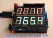
[Serial seven segment LED display shield](#) Seven segment LED displays are brighter, more attractive, and provide a far viewing distance as well as a wider viewing angle compared to LCD displays. This project describes a serial seven segment LED display shield for Arduino Uno or compatible boards. The shield consists of..... Listed under: [LED Projects](#)
