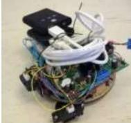
[Anti-Collision \(Wall Hugging\) Robot](#) Our project consists of a vehicle designed to avoid collisions with objects and walls. The vehicle achieves this through the use of an onboard sensor to determine when such an object was close by. [gallery columns="2" size="medium" ids="31197,31198"] After recognizing an object within a certain..... Listed under: [Robotics – Automation Projects](#)
