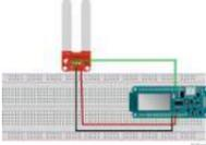
[IoT System To Monitor Soil Moisture With Arduino](#) This IoT system monitors the soil moisture using Arduino and sensors. Data are sent to an IoT cloud platform to access it anywhere. Things used in this project Hardware components Arduino MKR1000 × 1 SparkFun Soil Moisture Sensor (with Screw Terminals) × 1 Software apps..... Listed under: [Projects](#), [Sensor – Transducer – Detector Projects](#)
