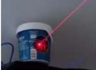
[Smartphone Controlled Cat Laser](#) <https://youtu.be/Q05TAoPIHtQ> I've been wanting to start exploring the world of microcontrollers and programming for some time now, so I came up with this simple project which uses an app called "Blynk" to allow you to wirelessly control an Arduino board through your wifi. Now obviously..... Listed under: [Phone Projects](#)
