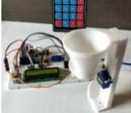
[Automatic Pet Feeder using Arduino](#) Today we are building an Automatic Pet Feeder Using Arduino which can automatically serve food to your pet timely. It has a DS3231 RTC (Real Time Clock) Module, which used to set time and date on which your pet should be given food. So, by..... Listed under: [Clock – Timer Projects](#)
