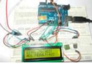
[How to Use ADC in Arduino Uno?](#) In this tutorial we are introducing concept of ADC (Analog to Digital Conversion) in ARDUINO UNO. Arduino board has six ADC channels, as show in figure below. Among those any one or all of them can be used as inputs for analog voltage. The Arduino Uno..... Listed under: [Other Projects](#)
