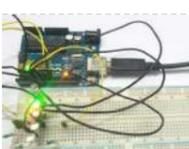
[RGB LED with Arduino](#) In this project we are going to interface 5 RGB (Red Green Blue) LEDs to Arduino Uno. These LEDs are connected in parallel for reducing PIN usage of Uno. The RGB LED will have four pins as shown in figure. PIN1: Color 1 negative terminal..... Listed under: [LED Projects](#)
