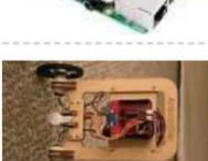
[BALANCE ROBOT ARDUINO UNO](#) Previously shared " Analog Balance Robot "project using Arduino Uno . Motor drive SparkFun Arduimoto this module is based on the L298 motor drive integration SMD materials are used because the size of the...Electronics Projects, Balance Robot Arduino Uno "arduino projects, " Previously shared " Analog Balance Robot "project using Arduino..... Listed under: [Robotics – Automation Projects](#)
