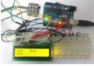
[Color Detector using Arduino Uno](#) In this project we are going to interface TCS3200 color sensor with Arduino UNO. TCS3200 is a color sensor which can detect any number of colors with right programming. TCS3200 contains RGB (Red Green Blue) arrays. As shown in figure on microscopic level one can see..... Listed under: [Other Projects](#)
