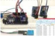
[Arduino Data Logger \(Log Temperature, Humidity, Time on SD Card and Computer\)](#) As Engineers/Developers we always rely upon the data collected to design or improve a system. Recording data and analyzing them is a common practice in most of the industries, here we are building Arduino Data Logger Project where we will learn how we can log..... Listed under: [Temperature Measurement Project Ideas](#)
