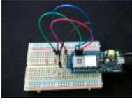
[Remote LED Mood Setter](#) Set LED RGB light Scenes remotely Things used in this project Hardware components Arduino MKR1000 × 1 Breadboard (generic) × 1 RGB Diffused Common Cathode × 1 Story Using MKR1000 to control an RGB LED device. In our shortened example we will use a single..... Listed under: [LED Projects](#), [Projects](#)
