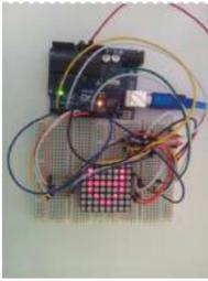
[Interfacing 8x8 LED Matrix with Arduino](#) LED matrix displays can be used to display almost anything. Most modern LED sign boards uses various types of matrix boards with controllers. In this tutorial we are going to interface a single color 8x8 LED matrix with Arduino and display a few characters in..... Listed under: [LED Projects](#)
