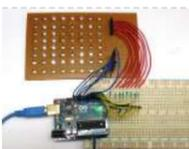
[Scrolling Text Display on 8x8 LED Matrix using Arduino](#) In this tutorial we are going to design an 8x8 LED Matrix Scrolling Display using Arduino Uno, which will show scrolling alphabets. 8x8 LED Matrix contains 64 LEDs (Light Emitting Diodes) which are arranged in the form of a matrix, hence the name is LED..... Listed under: [LED Projects](#)
