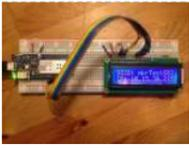
[Spartan WiFi Pager System](#) Simple Wifi pager system. Things used in this project Hardware components Arduino MKR1000 × 1 Adafruit Standard LCD - 16x2 White on Blue × 1 Story This project is an initial stage of the Spartan WIFI pager system (<https://www.hackster.io/challenges/arduino-microsoft-maker/ideas/2421>). First step in this stage is..... Listed under: [Projects](#), [Wifi - Wlan Projects](#)
