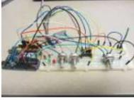
[Arduino Resistance Data Logger](#) I was working on a project were I needed a cheap and efficient way to log the changing resistance of a sensor while simultaneously logging the temperature. This project is similar in many respects to the other data loggers on my site. Three prototypes have..... Listed under: [Memory – Storage Projects](#)
