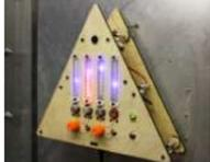
[Environmental Alert System](#) <https://youtu.be/gWZ6Z1ptUis> What's that smell? It's noxious gas of course! If you're in an environment where there's a possibility of gaseous release of which you'd rather not breathe, why not build an automatic system for sensing and alerting you? The design for the Environmental Alert System..... Listed under: [Security – Safety Projects](#)
