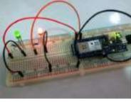
[Control your MKR1000 with aREST Framework](#) You can control your MKR1000 remotely with a RESTFUL interface. Things used in this project Hardware components Arduino MKR1000 × 1 LED (generic) × 2 Resistor 220 ohm × 2 Jumper wires (generic) × 5 Software apps and online services Arduino IDE Story It would..... Listed under: [LED Projects](#)
