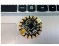
[How to Use the Adafruit Flora Board – Arduino Tutorial](#) In this tutorial you will learn how to use the Adafruit Flora board and how you can easily program it with Codebender! FLORA is Adafruit's fully-featured wearable electronics platform. It's a round, sewable, Arduino-compatible microcontroller designed to empower amazing wearables projects. The FLORA family also..... Listed under: [LED Projects](#)
