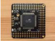
[DIY Bare Minimum Arduino Mega 2560](#) [2017 Update] Eagle files please click here. The objective of this project is to create a version of Arduino Mega 2560 board that has lower component count and smaller board size. Personally to be used for robotics projects that require ATmega2560's 256 KB flash and digital/analog..... Listed under: [LED Projects](#)
