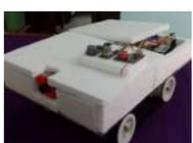
[Teleoperated Robot for Sensing the Toxic Gases](#) Remotely operated ground vehicle for sensing the toxic gases which is helpful for firefighters and researchers. Things used in this project Hardware components Arduino Yun × 1 Arduino MKR1000 × 1 Seeed Grove - Air quality sensor v1.3 × 1 Seeed Grove - Gas Sensor(MQ2)..... Listed under: [Projects](#), [Robotics – Automation Projects](#)
