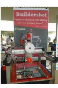
[Arduino Controlled CNC / 3D Printer Hybrid](#) The objective of this instructable is to guide your way throw the entire making process of building a BuildersBot machine. An open design Arduino Controlled CNC Router that can also perform 3D printing. The instructions will cover all areas such as design, mechanics, electronics and..... Listed under: [CNC Machines Projects](#)
