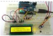
[Magnetic Field Strength Measurement using Arduino](#) In this project we are using the concept of ADC (Analog to Digital Conversion) in ARDUINO UNO. We are going to use a Hall Effect sensor and Arduino uno to measure the field strength of a magnet. The sensor which we have used here is UGN3503U. This..... Listed under: [Other Projects](#)
