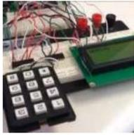
[Alarm System](#) The objective of our project was to create an alarm system that could detect an intruder using an IR motion sensor. We used a keypad so the user could enter their password to arm and disarm the system. [gallery columns="2" size="medium" ids="31154,31155"] We also included..... Listed under: [Clock – Timer Projects](#)
