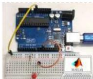
[Interfacing Arduino with MATLAB – Blinking LED](#) In this project, we are going to learn, How to set up hardware support for Arduino in MATLAB software. How to control an Arduino using MATLAB code. We normally use Arduino IDE to write and upload codes to Arduino. The advantage of MATLAB is, it..... Listed under: [LED Projects](#)
