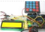
[Keypad Interfacing with Arduino Uno](#) In this tutorial we are going to interface a 4x4 (16 key) keypad with ARDUINO UNO. We all know keypad is one of the most important input devices used in electronics engineering. Keypad is the easiest and the cheapest way to give commands or instructions to..... Listed under: [Other Projects](#)
