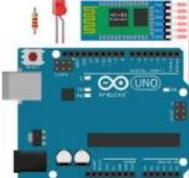
[Arduino Bluetooth Basic Tutorial](#) Ever thought of controlling any electronic devices with your smart phone ?Controlling your robot or any other devices with your smartphone will be really cool. Here is a simple and basic tutorial for interfacing Bluetooth with arduino Step 1: Things You Need Hardware Bluetooth Module HC 05/06ArduinoLED220Ω ResistorAndroid device..... Listed under: [Bluetooth Projects](#)
