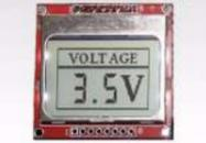
[DIY Voltmeter with Arduino and a Nokia 5110 Display](#) Story In this tutorial I am going to show you how to build a Voltmeter with a big Nokia 5110 LCD display using Arduino. Building a voltmeter is a great learning experience. When you finish building this project, you will have a better understanding of..... Listed under: [Metering – Instrument Projects](#)
