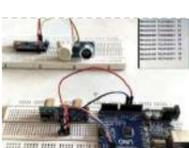
[How To Measure Distance Between Two Ultrasonic Sensors](#) Ultrasonic sensor (HC-SR04) is commonly used to find the distance of an object from one particular point. It has been fairly easy to do this with the Arduino and the code is also pretty simple. But in this article we are going to try something..... Listed under: [Calculator Projects](#), [Metering – Instrument Projects](#)
