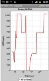
[Simple Remote Data Plotting using Android / Arduino / pfodApp](#) Simple Remote Data Plotting using Android / Arduino / pfodApp This Instructable shows you how to plot Arduino sensor data on your Android mobile and capture it for later downloading to your computer. These instructions are also available at [www.pfod.com.au](http://www.pfod.com.au) No Android programming is required..... Listed under: [Arduino Android](#), [Arduino Programmer Projects](#), [Phone Projects](#)
