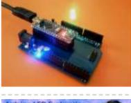
[Arduino Nano to Arduino Uno Adapter](#) Arduino Nano is a nice, small and cheap member of the Arduino family. It is based on the Atmega328 chip, what makes it as powerful as the biggest his brother Arduino Uno, but it can be obtained for less money. In Ebay now Chinese versions..... Listed under: [Arduino Programmer Projects](#)
