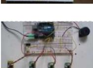
[Keyless piano using Arduino uno](#) Keyless piano using Arduino is sort of sequel to the DIY fun piano i have published in this website. In this project i have eliminated the need of buttons involved to play the piano. Here i have used IR in place of buttons. Let's get..... Listed under: [Other Projects](#)
