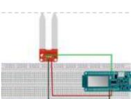
[IoT System To Monitor Soil Moisture With Arduino](#) This IoT system monitors the soil moisture using Arduino and sensors. Data are sent to an IoT cloud platform to access it anywhere. Things used in this project Hardware components Arduino MKR1000 × 1 SparkFun Soil Moisture Sensor (with Screw Terminals) × 1 Software apps..... Listed under: [Projects](#), [Sensor – Transducer – Detector Projects](#)
