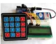
[Arduino Calculator using 4x4 Keypad](#) Programming is always fun and Arduino is a wonderful platform if you are just getting started with Embedded programming. In this tutorial we will build our own calculator with Arduino. The values can be sent in through a keypad (4x4 keypad) and result can be..... Listed under: [Battery Projects](#), [Blog](#), [Calculator Projects](#), [LCD Projects](#)
