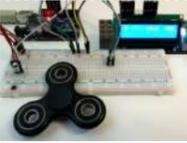
[Fidget Spinner RPM Counter](#) Hi everyone! This is my next project, Fidget Spinner RPM Counter or Arduino Tachometer with Hall-Effect Sensor. 1: Requirements Parts Required: Fidget Spinner neodymium magnet Arduino Uno LED + resistor 220 Ohm Hall-Effect Sensor - a3144 resistor 10 k Wires Breadboard LCD 1602 2: Hall-Effect..... Listed under: [Sensor – Transducer – Detector Projects](#)
