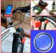
[DIY Speedometer using Arduino and Processing Android App](#) In this project we make a Cool Speedometer for bikes or any automotives by using Arduino which broadcast the speed using Bluetooth to an Android application that we created using Processing. The complete project is powered by an 18650 Lithium cell and hence highly portable along with your vehicle..... Listed under: [Bluetooth Projects](#)
