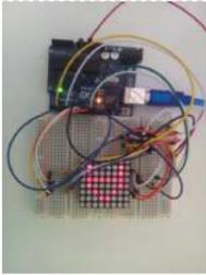
[Interfacing 8×8 LED Matrix with Arduino](#) LED matrix displays can be used to display almost anything. Most modern LED sign boards uses various types of matrix boards with controllers. In this tutorial we are going to interface a single color 8×8 LED matrix with Arduino and display a few characters in..... Listed under: [LED Projects](#)
