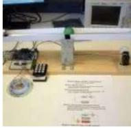
[Balance Beam Controller](#) The purpose of our final project was to create an unstable system that would allow us to investigate classical control design methods by controlling the system using a microcomputer. [gallery columns="2" size="medium" ids="31225,31226"] This was accomplished by creating a teeter-totter that pivoted around a central..... Listed under: [Sensor – Transducer – Detector Projects](#)
