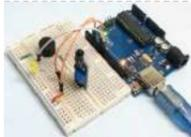
204. [Interfacing Flame Sensor with Arduino to Build a Fire Alarm System](#) In this article we interface Flame Sensor with Arduino and learn all the steps to build Fire Alarm System by using Arduino and flame sensor. Flame sensor module has photodiode to detect the light and op-amp to control the sensitivity. It is used to detect fire and provide HIGH signal upon..... Listed under: [Sensor – Transducer – Detector Projects](#)
