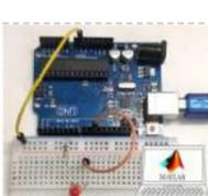
[Interfacing Arduino with MATLAB – Blinking LED](#) In this project, we are going to learn, How to set up hardware support for Arduino in MATLAB software. How to control an Arduino using MATLAB code. We normally use Arduino IDE to write and upload codes to Arduino. The advantage of MATLAB is, it..... Listed under: [LED Projects](#)
