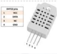
[Temperature and Humidity monitoring with DHT22 sensor Arduino Uno R3](#) The objective of this tutorial is to learn how to use the DHT22 sensor with Arduino uno. The room temperature and humidity will be printed to serial monitor and also will be displayed to the LCD 4×20 in Proteus ISIS. [caption id="attachment\_28379" align="aligncenter" width="300"] DHT22..... Listed under: [Temperature Measurement Projects](#)
