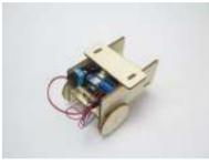
[MKR1000 Robot Controlled Via WiFi Using Arduino](#) This project consists of a small robot controlled via WiFi using an Arduino MKR1000, MKR2UNO Shield Adapter and Arduino Motor Shield! Things used in this project Hardware components Arduino MKR1000 × 1 Arduino MKR2UNO Adapter × 1 Arduino MotorShield Rev3 × 1 Arduino Small DC..... Listed under: [Battery Projects](#), [Robotics – Automation Project Ideas](#)
