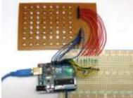
[Scrolling Text Display on 8x8 LED Matrix using Arduino](#) In this tutorial we are going to design an 8x8 LED Matrix Scrolling Display using Arduino Uno, which will show scrolling alphabets. 8x8 LED Matrix contains 64 LEDs (Light Emitting Diodes) which are arranged in the form of a matrix, hence the name is LED..... Listed under: [LED Projects](#)
