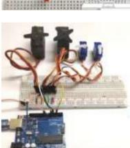
[Controlling Multiple Servo Motors with Arduino](#) Using one or two Servo with Arduino is Easy but what if we want to use more than one Servo Motors? Here, we are going to show you that how to control Multiple Servo Motors with Arduino. Connecting multiple Servo Motors with Arduino seems to..... Listed under: [Motor Projects](#)
