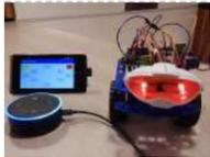
[Build A Voice-Controlled Robot Using Arduino](#) Story Voice-controlled Robot Voice-controlled robot is both hardware and cloud solution in one piece. The main components are: 1. Alexa Skill - to interpret voice commands and translate them to Google Cloud Messaging messages - deployed to Heroku cloud 2. Android application - to receive..... Listed under: [Robotics – Automation Projects](#)
