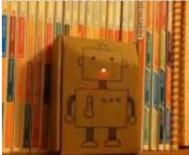
[Temperature Recording Arduino Robot](#) My son and myself made a little arduino robot that records temperature. He wanted me to draw a robot, I wanted to experiment with blinking LEDs relaying data so a plan was hatched. The way the LEDs work is as follows: Green = lowest temperature..... Listed under: [Ideas](#), [Robotics – Automation Project Ideas](#)
