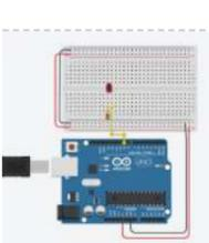
[Fading LED With Arduino Analog Output in Tinkercad](#) <https://youtu.be/X8dHbdhnGKY> Let's learn to adjust an LED's brightness using one of the Arduino's analog outputs. You've probably already learned how to use Arduino's digital i/o pins to send HIGH and LOW signals to an LED, but some of these pins are capable of simulating a signal..... Listed under: [LED Projects](#)
