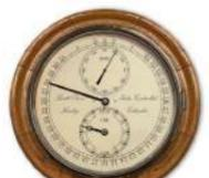
[Arduino Perpetual Calendar Clock](#) The clock uses 2 electro mechanical clock movements controlled by an Arduino to display the Day and Month. A third quartz controlled movement displays the time tide Low or High tide. The Calendar is fully automatic and takes into account leap years as well as..... Listed under: [Clock – Timer Projects](#)
