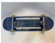
[LED Skateboard Rubiks Cube](#) This project uses LED lights controlled by an accelerometer and gyroscope to challenge your skateboarding creativity. The LED lights change according to what trick is being performed. For example, a shuvit (180-degree yaw rotation) changes the lights blue. a kickflip (360-degree roll) changes the color..... Listed under: [Game – Entertainment Projects](#), [LED Projects](#)
