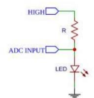
357. [An LED You Can Blow Out Like a Candle!](#) LEDs are designed to emit light, but they also make surprisingly capable sensors. Using only an Arduino UNO, an LED and a resistor, we will build a hot LED anemometer that measures wind speed, and turns off the LED for 2 seconds when it detects..... Listed under: [LED Projects](#)
