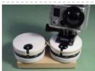
884. [Panner With Arduino](#) This project it's a new time-lapse tripod or panning with two axis that works with an arduino protoboard. Everyone will be able to create their own time-lapse trajectory without need to check it. With the arduino code we'll can change the value for the movement..... Listed under: [Motor Projects](#)
