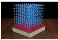
[How to Build 8x8x8 LED Cube](#) An 8x8x8 LED cube is a visual treat with 3D effects and patterns. It works on the concept of Persistence of Vision, a feature of the human eye which tricks our brain in to thinking that an object is present permanently at a place if..... Listed under: [LED Projects](#)
