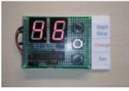
[Arduino Countdown Timer With Setup Buttons](#) In this Instructables guide I will show you how to make your own Arduino two digit countdown timer. I made my own circuit by using the ATmega328 micro controller but this is an optional step. In this guide I will help you to make it..... Listed under: [Other Projects](#)
