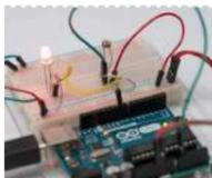
354. [Light Sensor \(Photoresistor\) With Arduino in Tinkercad](#) Let's learn how to read a photoresistor, a light-sensitive type of variable resistor, using Arduino's Analog Input. It's also called an LDR (light-dependent resistor). So far you've already learned to control LEDs with Arduino's analog output, and to read a potentiometer, which is another type of variable..... Listed under: [Sensor – Transducer – Detector Projects](#)
