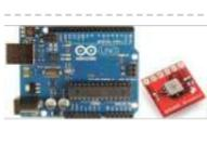
[Arduino Barometric Pressure Web Server](#) This example shows how to use SPI communications to read data from a SCP1000 Barometric Pressure sensor, and how to then post that data to the web by using your Arduino/Ethernet Shield combo as a simple web server. Using the Ethernet library, your device will..... Listed under: [Internet – Ethernet – LAN Projects](#), [Projects](#), [Sensor – Transducer – Detector Projects](#)
