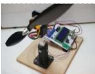
[Brushless Motor Thrust Stand](#) Back in the time when I was building my Arduino based Ludwik Drone I faced a problem of choosing proper motors and propellers. I didn't know anything about drones at that time so I had to trust motor manufacturer and the datasheet of a motor..... Listed under: [Motor Projects](#)
