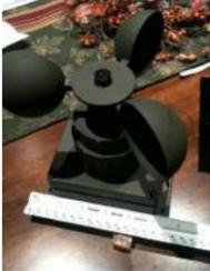
[A Self-Contained Data Logging Anemometer](#) I love collecting and analyzing data. I also love building electronic gadgets. A year ago when I discovered the Arduino products, I immediately thought, "I'd like to collect environmental data." It was a windy day in Portland, OR, so I decided to capture wind data..... Listed under: [Metering – Instrument Projects](#)
