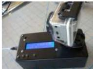
495. [Timelapse Panning controller for GoPro Cameras](#) This instructible will show you how I built (and you can also build) an Arduino Timelapse Panning controller for GoPro cameras. There are obviously some refinements that can be made to the design, but in general I am very happy with the results that I've..... Listed under: [Video – Camera – Imaging Projects](#)
