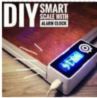
346. [DIY Smart Scale With Alarm Clock \(with Wi-Fi, ESP8266, Arduino IDE and Adafruit.io\)](#) In my previous project, I developed a smart bathroom scale with Wi-Fi. It can measure user's weight, display it locally and send it to the cloud. You can get more details about this on link below: <https://www.instructables.com/id/Wi-Fi-Smart-Scale-with-ESP8266-Arduino-IDE-Adafruit/> This solved part of my problems: how to..... Listed under: [Clock – Timer Projects](#)
