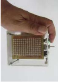
[GYRO & VOICE ARDUIGAMES](#) This gaming box is made from Arduino Uno R3, LoLShield, MPU6050 and Microphone module. With LoLShield, we can show a message/scrolling message or animation picture like: plasma effect, sinewave effect...With MPU6050, we can read value from accelerometer and gyroscope to control movement for simple games..... Listed under: [Game – Entertainment Projects](#)
