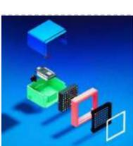
[RGB Box Clock](https://youtu.be/7inXakX4XOs) <https://youtu.be/7inXakX4XOs> This is a clock and decorative RGB Led Matrix It's controlled by a Colorduino Shield and NodeMCU v3 Board using i2C communication. With Blynk app you can setup the alarm,change colors and other things. Parts list is: LoLin V3 NodeMcu Lua CH340G ESP8266 Board..... Listed under: [Clock – Timer Projects](#)
