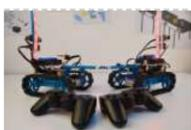
757. [Infrared Fighting Tank](#) <https://youtu.be/XMgdvILuDaU> This project is to make two infrared fighting tanks with Starter Robot Kits, some mechanical parts and electric modules. They are controlled with 2.4G wireless joystick. So, how to make it? Step 1: Parts Required 2 x Starter Robot Kit(Bluetooth or IR version) 4 x Beam0808-136-Blue 2..... Listed under: [Other Projects](#)
