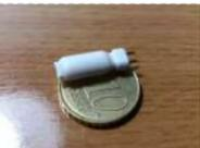
[DIY Tilt Switch.](#) In this instructable I'll show you how to make a simple tilt switch, this tilt switch works best with microcontrollers that can debounce the signal and overcome interferences produced by vibrations. There are many ways to make a tilt switch, this one is a cheap..... Listed under: [Other Projects](#)
