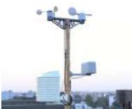
[Solar Powered WiFi Weather Station V3.0](#) In this Instructable, we will learn how to make a Solar-powered wireless weather station by using an ESP32 Wifi Module and few common weather sensors available in the market. The weather station is fully solar-powered, so no need to worry about the external power supply..... Listed under: [Wifi - Wlan Projects](#)
