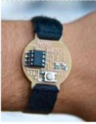
[The Nerd Watch](#) Hello! Welcome to another Other Machine project tutorial! I'm Sam DeRose, a former Other Machine Co. Summer Intern. I created the Nerd Watch last summer while working at OMC. The Nerd Watch displays the time in binary when the button is pushed. The watch shows the..... Listed under: [Clock – Timer Projects](#)
