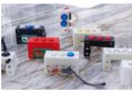
[Simple Arcade Button Ideas for Your Projects](#) One thing that I've always needed for my projects is a simple form of input and output. At first, it was a simple push button and an led on a breadboard. The breadboard mounted buttons are inconvenient. So I created a 3D printed stand to..... Listed under: [Ideas](#)
