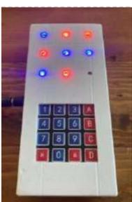
[Neo Pixel Tic Tac Toe \(Arduino Uno\)](#) Tic Tac Toe is a two player game in which the players compete to get 3 pieces in a row. In this project we constructed a Tic Tac Toe game using a number pad and neo pixels as pieces. This results in a portable Tic..... Listed under: [LED Projects](#)
