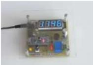
[Timer With TM1637 and Arduino](#) This timer is useful in both domestic and industrial applications. It is a countdown timer programmable in the range of 1s .... 9999s. During this time, the load is powered by a relay on the board. For repeated timings, it is possible to memorize the..... Listed under: [Clock – Timer Projects](#)
