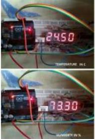
[Temperature and Humidity Monitor Using DHT22 & MAX7219](#) We always need to see the temperature and humidity when we sitting in our house to know whether we need to turn on/off AC, heater,cooler,etc. So here we have build this circuit to display temperature and humidity on the 7-segment displays, and we have used..... Listed under: [Temperature Measurement Projects](#)
