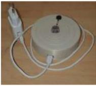
[Gas Detector](#) Let's create a simple Gas Detector connectable to WiFi. The gadget would offer: web UI including gauges for LPG, CO, Smokesimple data handler returning values in JSONcapable of regularly sending data to ThingSpeak server andobviously triggering loud alarm if threshold of dangerous concentrations exceeded. We..... Listed under: [Sensor – Transducer – Detector Projects](#)
