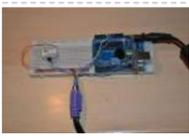
[The morse code generator by a PS/2 keyboard using Arduino](#) Hi, all! Today I'm trying to explain you my last project: "The morse code generator by a PS/2 keyboard" I've used an PS/2 keyboard to send input to my Arduino board (like described in here) and transform it in morse code that activate..... Listed under: [Arduino Programmer Projects](#), [Projects](#)
