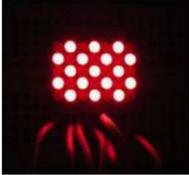
[Using a Dot Matrix LED with an Arduino and Shift Register](#) The Siemens DLO7135 Dot matrix LED is one amazing piece of optoelectronics. It's billed as a 5x7 Dot Matrix Intelligent Display (r) with Memory/Decoder/Driver. Along with that memory, it's got a 96-character ASCII display set with upper and lower case characters, a built-in character generator..... Listed under: [LED Projects, Projects](#)
