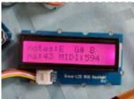
[Basic Arduino MIDI Arppegiator](#) In this instructable I will show you how to make a basic MIDI instrument using an Arduino Uno. This instrument plays three notes (a triad) in a row. Using the different potentiometers, you can move up and down the notes as well as up and down..... Listed under: [Other Projects](#)
