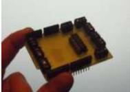
[Arduino stepper motor and servos shield](#) This instructable will show you show to build an Arduino shield which can be used to control 3 servos and 1 stepper motor using 4 potentiometers. You will need: access to a laser printer/cnc router/etching chemicals 7 x 3 pin 3.5mm terminal blocks 2 x..... Listed under: [Motor Projects](#), [Projects](#)
