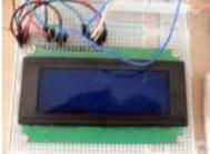
[Arduino LCD Metronome](#) Connecting the LCD The first step is to wire up the LCD. The HD44780 has 16 pins: Pin 1 - Vss Pin 2 - Vdd Pin 3 - Vo Pin 4 - RS Pin 5 - R/W Pin 6 - E Pin 7 - DB0..... Listed under: [LED Projects](#)
