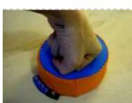
[Analog Fabric Joypad using an Arduino](#) How to make an "analog" input device from fabric and a few other necessary materials. "Analog" in parenthesis because, although it is made up of 4 analog inputs, the only analog transition between the directions (up, right, down and left) comes from the buffering material..... Listed under: [Game – Entertainment Projects](#), [Projects](#)
