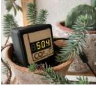
[CO2 Display](#) As its name suggests, the CO2 Display project is a small CO2 gas sensor to be plugged into USB to easily track indoor and outdoor pollution. The CO2 level is displayed live, but it is possible with the small application provided in the documentation to generate..... Listed under: [Sensor – Transducer – Detector Projects](#)
