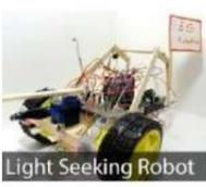
[LDR Robot using an Arduino](#) LDR Robot with IR and a Servo The LDR/IR Robot is designed to seek out light and avoid obstacles. The robot uses the Light Dependent Resistor to seek out light and the Infrared Sensor to detect and avoid objects in its path. The following are..... Listed under: [Projects](#), [Robotics – Automation Projects](#)
