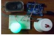
[Make a Mini LED Siren powered by Arduino](#) This is one of the first projects I have made with Arduino. It's a little siren with a LED that fades and blinks on and off. It demonstrates basic use of LEDs and speakers. Also check out this article: 8-Pin Programming Shield Constructive criticism is..... Listed under: [Arduino LED Project Ideas, Ideas, Sound – Audio Project Ideas](#)
