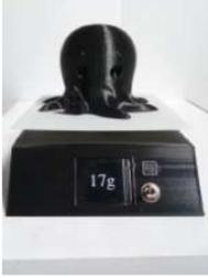
[3D Printed Kitchen Scale Using an ESP8266](#) Hello everyone ! Today I'm going to show you how I built this little kitchen scale during this lockdown ! It can measure weights up to several kilograms, has an included battery, a nice display and can even be turned into a connected scale thanks..... Listed under: [Temperature Measurement Projects](#)
