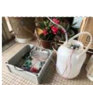
[Automatic Irrigation System \(Arduino\) With Usb Type DC Submersible Water Pump](#) This mini project is involved to use Arduino to control submersible water pump when soil reach below or above predefined moisture level. How it works ? 1. Soil moisture sensor is reading analog signal which transmit to Arduino. 2. Arduino control submersible water pump ON..... Listed under: [Interfacing\(USB – RS232 – I2c -ISP\) Projects](#)
