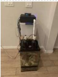
[Automated Bioactive Tropical Reptile Vivarium \(using Arduino\)](#) I have multiple bioactive tropical vivariums for my crested geckos, and I always need to spray them morning and night, as well as when the humidity is too low (which happens multiple times per day), and I have to turn on and off the lights..... Listed under: [Other Project Ideas](#)
