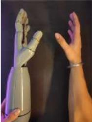
[Cyborg Hand : Robotic-cum-Prosthetic Servo Powered Hand](https://youtu.be/gO7L46sZTY4) <https://youtu.be/gO7L46sZTY4> Supplies Hey there ! For this Instructable you will need: 1- 3d Printer 2- CAD software( TinkerCad / Fusion360 ) 3- PLA and TPU filament 4- Servos [ MG995 ] 5- Arduino 6- Wires and Breadboard 7- Rubber bands 8- Thread / String (..... Listed under: [Robotics – Automation Project Ideas](#)
