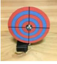
[Laser Shooting Game](#) This laser game is a simple project that utilizes an Arduino mini. All target boards have an Arduino, sensors, and servo control ports. Shooting the target center triggers the servo and the board falls flat. Step 1:What you need [box color="#985D00" bg="#FFF8CB" font="verdana" fontsize="14 "..... Listed under: [Game – Entertainment Projects](#)
