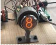
[Controlling Nixie Tube With Arduino Using K155ID1 Microchip](#) For those who don't know Nixie tubes are electronic devices used for displaying numbers and other character using glow discharge. They date back to 1950s not used commercially anymore. Currently they do experience second life though, as people do tons of cool projects. In this..... Listed under: [Other Projects](#)
