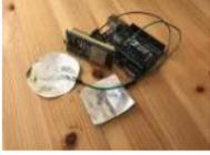
[Arduino/ESP32 Capacitive Touch Sensor](#) Adding touch interfaces to your projects might seem difficult at first, but it really isn't. In this Instructable I'll show you how to do it using an Arduino or ESP32 development board. What you will need: an Arduino\* or ESP32 development board a wiresome tinfolosome sticky..... Listed under: [Sensor – Transducer – Detector Projects](#)
