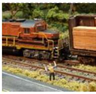
[Wii Nunchuk Controlled Model Train using Arduino](#) Using an Arduino microcontroller, an Adafruit motor shield, and a Wii Nunchuk, you can create a intuitive, programmable, model train controller to run your layout. Amaze your friends. Entertain your kids. Not quite DC, not quite DCC. You're headed for the hacker lands of PWM..... Listed under: [Game – Entertainment Projects](#), [Projects](#)
