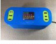
[Arduino Cable Tracer](#) Instantly diagnose the type and integrity of USB cables with this Arduino Cable Tracer. Suitable to trace USB A, Mini, Mico, and USB-C cables this is very useful to identify the exact wiring configuration and also diagnose broken connections. Step 1: Gather the Materials and..... Listed under: [Interfacing\(USB – RS232 – I2c –ISP\) Projects](#)
