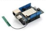
[Add Linux, WiFi, Ethernet and USB to Arduino](#) Web site: <http://www.dragino.com/products/yunshield/item/86-yun-shield.html> Project Summary: The model of this shield named Yun Shield, the feature of this shield is as its name. User can add this shield into Arduino (Leonardo, UNO, MEGA2560 etc) and "turn" the Arduino into device which has similar features as Arduino..... Listed under: [Interfacing\(USB – RS232 – I2c -ISP\) Projects](#), [Internet – Ethernet – LAN Projects](#)
