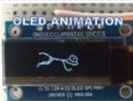
[Create Animation on OLED Display Controlled by Arduino](#) In this tutorial I will show you how to create animation on small OLED display connected to Arduino Nano. Step 1: Supplies We need following two components for this project Arduino NanoSSD1306 SPI 128x32 display You can also use SSD1306SPI 128x32 display but it will..... Listed under: [LED Projects](#)
