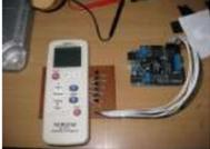
[Build a transistor circuit board for controlling Air Conditioner remote control with Arduino](#) I was supporting a group of student on their graduation project. One of the difficulties they faced was on controlling an A/C unit with Arduino microcontroller. The first experiment we tried to work it out was by record the A/C remote control beam signal for..... Listed under: [Home Automation Projects](#), [Projects](#)
