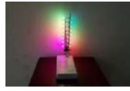
[Rainbow Led Circuit Sculpture](#) Today I would like to share how to make a sculpture circuit that controls 16 RGB leds using ATTINY85. We can adjust their colors separately according to the colorwheel rule with a touch button. Step 1: Things We Need The main components are as follows:..... Listed under: [LED Projects](#)
