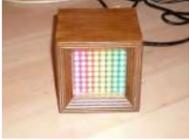
[64 pixel RGB LED Display – Another Arduino Clone](#) This display is based on an 8x8 RGB LED Matrix. For testing purposes it was connected to a standard Arduino board (Diecimila) using 4 shift registers. After getting it to work I permatized it on a fabbed PCB. The shift registers are 8-bit wide and..... Listed under: [LED Projects](#), [Projects](#)
