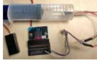
[Measure Pressure With Your Micro:bit](#) The following instructable describes a easy to build and inexpensive device to perform pressure measurements and demonstrate Boyle's law, using the micro:bit in combination with the BMP280 pressure/temperature sensor. Whereas this syringe/pressure sensor combination has already been described in one of my previous instructables, the combination..... Listed under: [Other Projects](#)
