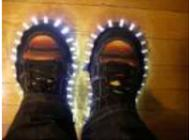
[Super Brite LED Sneakers 1.0 using an Arduino](#) Create your own Super Bright LED-lined sneakers that blink with multiple patterns. 1.0 FEATURES: - 1 color LEDs - 6 patterns - reed sensors + magnets that give you control to step through patterns - detachable velcro design - small, wearable microcontroller + power Step..... Listed under: [Game – Entertainment Projects](#), [Home Automation Projects](#), [LED Projects](#), [Projects](#)
