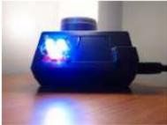
[Visual Network Threat Level Indicator v2 using Arduino](#) By popular request this is a new wireless version of the Visual Network Threat Level Indicator. This uses a Roving Networks WiFly RN-XV Module to do 802.11 WiFi along with an Arduino to display the threat level on your network. Network monitoring is very important in todays..... Listed under: [Internet – Ethernet – LAN Projects, Projects](#)
