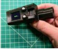
[3D Printed Spirometer](#) Spirometers are the classical instrument to perform the parsing of air as it is blown out of your mouth. They consist of a tube that you blow into that records the volume and speed of one breath which are then compared to a set of..... Listed under: [Metering – Instrument Projects](#)
