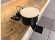
[A Simple Arduino Touchless Candy Dispenser](#) This is a simple touchless candy dispenser using an ultrasonic sensor for activation, a stepper motor to dispense candy, and an Arduino for controlling everything. The candy dispenser can be powered using the USB port or using a 9v battery. Inside the cylindrical container, there..... Listed under: [Other Projects](#)
