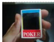
[Tiny MatchBox LCD Display – Desktop Decor](#) Have a nice day, in this instructable I'll explain how to make a little decorative display for your desktop. It connects to your PC via USB and you can upload any image you want (240\*240 BMP) It uses an Arduino pro micro for the serial..... Listed under: [LCD Projects](#)
