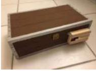
[Arduino Safe With Multivibrator Changeable 4-digit Combination](#) This instructable will explain how to wire, code, and build a functioning DIY arduino safe with multivibrator changeable 4-digit combination. Well what does that mean? A arduino safe with multivibrator changeable 4-digit combination is a functioning safe with a changeable password/combination, it features a series..... Listed under: [Security – Safety Project Ideas](#)
