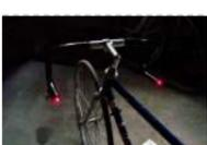
[Bike Turn Signal & Brake Light Handlebars](#) This project was inspired by a very cool kickstarter called Helios Bars. Essentially what this project does, is put an arduino, LEDs, and buttons into your bike handlebars. The LEDs can be used as turn signals, brake lights, or display ambient
