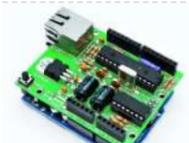
[Low cost Ethernet shield with ENC28J60 using Arduino](#) Economical alternative to original Arduino ethernet shields, allows data rates up to 10 Mbps and is achieved with a traditional assembly components. One of the most interesting shield that you can mount on the Arduino platform is certainly the ethernet shield, because enable numerous networking..... Listed under: [Internet – Ethernet – LAN Projects](#), [Projects](#)
