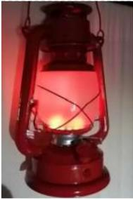
[NeoPixel Ancient Oil Lamp](#) In this Instructable, we will describe how to turn a "retro" oil lamp into a NeoPixels based rechargeable lamp with colorful light effects. Supplies Arduino nano 12 bits NeoPixel ring Micro USB 5V 1A TP4056 Lithium battery charger module 3.7V 9800mAh Lipo Li-polymer Battery Rotary encoder Ec11 or KY-040..... Listed under: [Other Projects](#)
