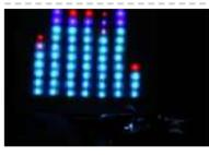
[Big Spectrum Analyzer with Arduino](#) Let's put together a pixel strip with an HL1606, an Arduino UNO and the Spectrum Shield to build a seven bands "large" Spectrum Analyzer of simple construction. The Strip used uses the HL1606 controller to allow direct management of each of the LEDs. The chip..... Listed under: [Game – Entertainment Projects](#), [Home Automation Projects](#), [Projects](#)
