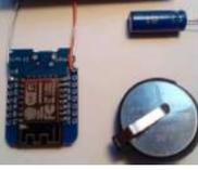
[Remote Control: ESP8266 With Coin Cell](#) The big problem using the ESPs is the power consumption when Wifi "goes up", about 100-200mA, peak up to 300mA. Normal coin cells deliver a few mA, peak up to 20-40mA. But for the ESPs the voltage will collapse. We need "a little help of my..... Listed under: [Other Projects](#)
