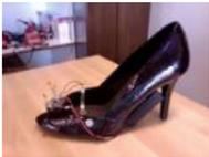
[High Heel Massage using an Arduino](#) My project is to make a heel (shoe) that senses when your foot is tired and then eases the pain. I will have a force sensor measure how much pressure is on your foot for 3 minutes. If the pressure is at a certain measure..... Listed under: [Home Automation Projects, Projects, Sensor – Transducer – Detector Projects](#)
