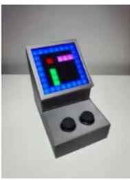
[Complete Arduino-based 3D-printed Battery-powered Mini Retro Arcade Machine](#) It's been a while since I've published my last Instructables. I'm back, and I'm 3D-printed-powered! Enjoy this mini retro arcade machine. It's literally my first complete end-to-end 3D-printed project: I made the design, printed it, assembled the electronics, programmed it, and now to the tutorial..... Listed under: [Battery Projects](#)
