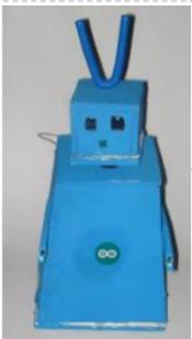
145. Uno The Arduino Robot Age: 13 Meet Uno the Arduino powered robot. Some functions include a blinking nose, moving antennas, rotating head, IR distance sensor, twin motor gear box and rotation counters. Uno is made with relatively easy to obtain parts. This project provides a good introduction to Arduino. robot.skp475 KB Step 1: Materials Material and tools • Foam board..... Listed under: Projects, Robotics – Automation Projects
