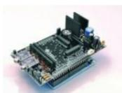
GSM GPS shield for Arduino Board Shield for Arduino designed and based on the module GSM/GPRS SIM900 or the GSM/GPRS & GPS module SIM908, to make calls, voice and data connections via GPRS. HARDWARE INNOVATIONS This new version (old Arduino GSM shield) has several new hardware features, that allow maximum customization..... Listed under: GPS Based Projects, Phone Projects, Projects
