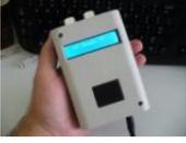
7. **Ultrasonic Combination Switch using an Arduino** Time for a follow-up to the Single Button Combination Lock by creating another oddball type of switch/lock. To activate this switch we make use of a Parallax Ping))) Ultrasonic sensor, an Arduino-style board and some other hardware – to make a device that receives a four-number code..... Listed under: Medical – Health based Projects, Projects
