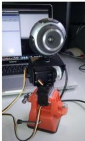
Remote controlled webcam using Arduino Web-enable your interactive sensors over desktop, smartphone and tablet devices. This tutorial describes in detail how to use the free SensorMonkey service to remotely control a pan and tilt webcam attached to an Arduino using nothing more than a simple webpage. The webpage can be..... Listed under: Internet – Ethernet – LAN Projects, Projects, Video – Camera – Imaging Projects
