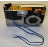
Time Lapse Digital Camera using Arduino Following the instructable here, I was able to turn an old digital camera into a time lapse camera using an arduino, a relay, and an open source software program called makeAVI (windows). To modify the camera I disassembled the camera cover and removed the button that..... Listed under: Projects, Video – Camera – Imaging Projects
