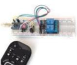
Controlling relay switches with an infrared remote The infrared (IR) communication technology, which existed long before WiFi and Bluetooth, is still a key component in implementing major components of a typical home automation system. For example, IR technology is still used in cordless headphones, for intrusion detection in home security systems, and in handheld..... Listed under: Other Projects
