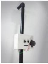
603. How to make a Smart Cane for the Visually Impaired with Arduino I wanted to make something for them to help the visually impaired become independent, so I created an open source Arduino project for a Smart Cane. This Arduino smart cane can assist with walking alone in new environments by taking inputs through an obstacle sensor..... Listed under: Other Projects
