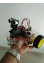
Robot using Arduino and Bluetooth Module (Obstacle Avoidance Robot) This project is designed to build a robot that automatically detects the obstacle on its path and guides itself whenever an obstacle comes ahead of it. This robotic vehicle is built, using Arduino UNO board. An ultrasonic sensor is used to detect any obstacle ahead..... Listed under: Robotics – Automation Projects
