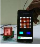
Bluetooth Controlled 8×8 LED Matrix Sign Board Display using Arduino Be it the long stretched highways or your doctors front door, we have sign boards placed everywhere to provide us information. But these sign boards are often boring and cannot be configured as per our interest from time to time. So in this project we..... Listed under: LED Projects
