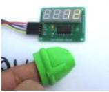
Arduino measures heart beat rate from fingertip The PIC16F628A based heart rate meter is one of the most popular projects published on Embedded Lab. In this article, I am going to show how to replicate the same project using a simpler platform like Arduino. The Arduino heart rate meter will use Arduino..... Listed under: Medical – Health based Projects
