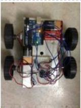
559. Remote Controlled Robot Using Arduino and T.V. Remote This remote controlled car can be moved around using practically any kind of remote such as TV,AC etc. It makes use of the fact that the remote emits IR(infrared). This property is made use of by using an IR receiver,which is a very cheap sensor..... Listed under: Robotics – Automation Project Ideas
