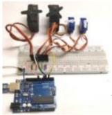
Controlling Multiple Servo Motors with Arduino Using one or two Servo with Arduino is Easy but what if we want to use more than one Servo Motors? Here, we are going to show you that how to control Multiple Servo Motors with Arduino. Connecting multiple Servo Motors with Arduino seems to..... Listed under: Motor Projects
