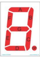
Arduino and 7 Segment Display – Interfacing Tutorial In this article, we are publishing a tutorial on how to interface seven segment LED display to Arduino. Seven segment displays are used in many embedded system and industrial applications where the range of outputs to be shown is known beforehand. Basic 1 digit seven segment..... Listed under: LED Projects
