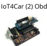
26. IoT4Car (2) ObdiUartMkrShield is a socket board for Arduino MKR board to talk with vehicles through ODB-II interface. Things used in this project Hardware components Arduino MKR1000 × 1 OSH Park Custom fabricated PCB × 1 Sparkfun - OBDII to DB9 cable × 1 Software apps and..... Listed under: Car Projects, Projects
