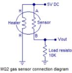
LPG sensor using arduino LPG sensor using arduino with alarm and cutoff. A simple LPG sensor using arduino is shown in this article. This circuit indicates the amount of LPG in the air. The circuit sounds an alarm and trips a relay when the concentration is above a predetermined..... Listed under: Sensor – Transducer – Detector Projects
