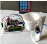
Automatic Pet Feeder using Arduino Today we are building an Arduino based Automatic Pet Feeder which can automatically serve food to your pet timely. It has a DS3231 RTC (Real Time Clock) Module, which used to set time and date on which your pet should be given food. So, by..... Listed under: Clock – Timer Projects
