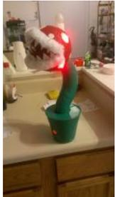
LED Super Mario Piranha Plant using an Arduino We are going to make an Arduino control LED Piranha Plant :] Step 1: What you'll need Arduino Uno 9 Resistors 9 LEDs - Red, Yellow, Orange is best since they need less amperage PIR sensor 9v battery arduino wall plug (you'll be cutting the connection..... Listed under: Game – Entertainment Projects, Projects
