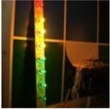
Audio VU meter with Extra wide Dynamic Range 69 dB using Arduino O'K, after having some fun with stereo version of the VU meter I described in my previous blog-post, now it's time to do a serious stuff. Studio grade VU meter !!! 24 steps, equally spaced every 3 dB, covering Extra wide Dynamic Range from -63 up to..... Listed under: Metering – Instrument Projects, Projects, Sound – Audio Projects
