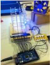
64. Quantitative Two-Dimensional Temperature Measurements Lab Experiments involving the Heat Equation are usually one-dimensional exercises involving a copper pipe and a half-dozen thermocouples. But with DS18B20 "One-Wire" thermometer chips and an Arduino, it's possible to measure hundreds of temperature values simultaneously. Here's what my students Daniel Lund and Lawrence Lechuga..... Listed under: Temperature Measurement Projects
