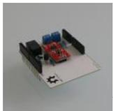
52. Energino: an Arduino-based energy consumption monitoring shield Energino is a plug-load meter that measures the amount of power consumed by whatever DC electrical appliance is plugged into its. It was originally designed to monitor the energy consumption of simple networking devices such as Ethernet switches and WiFi access points, but it can..... Listed under: Metering – Instrument Projects
