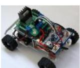
Simple RC car for beginners (Android control over Bluetooth) This is a simple project of Android Bluetooth Car with Bluetooth control. Arduino controller is used To control the car used Android-device with a built-in accelerometer. Tilt forward - car goes forward, tilt to the left - car turns to the left, tilt back - car..... Listed under: Car Projects, Game – Entertainment Projects, Internet – Ethernet – LAN Projects
