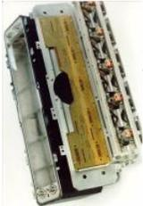
314. The Photometric Camera and the CCDs The Photometric System The photometric camera for the SDSS consists of two TDI scanning CCD arrays, one, using 30 Tektronix/SITE 2048 x 2048 CCDs in a 5 by 6 array for five-color photometry, and the other using 24 2048 x 400 chips for astrometry and..... Listed under: Video – Camera – Imaging Projects
