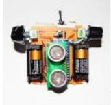
Haptic Proximity Module (HPM) for Low Vision users The Haptic Proximity Module (HPM) seeks to enable people with low vision, or other vision impairments, to engage with their direct surroundings through vibration feedback from a range detector, and do so cheaply with readily available components. The aim of this instructables is to share..... Listed under: Development Board – Kits Projects
