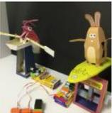
Papercraft Automata Race Game littleBits Circuit using Arduino This instructable will show you how to create a game using littleBits. The game will start with a sound trigger. Each player will have to press a button repeatedly. The first person to press their button 25 times wins. A buzzer will sound to end..... Listed under: Game – Entertainment Projects
