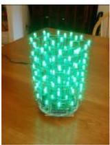
LED Cylinder using Arduino This is a little art project I made with 95 RGB LEDs arranged in a 3D cylinder shape, sitting atop a microcontroller-based driver circuit. The LEDs are individually addressable, and when you power it on, the software cycles through a series of animations, e.g. various..... Listed under: Game – Entertainment Projects, Home Automation Projects, LED Projects, Projects
