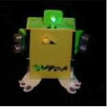
Wex, the One Eyed Watcher using an Arduino Wex detects your location with ultrasonic sensors then follows you with his one flashing eye. His red "heartbeat" can be seen through his mouth. Step 1: Parts needed include: Arduino Two ping ultrasonic sensors Futaba s3103 servo Radio Shack 276-0016 7 color led Radio Shack ..... Listed under: Projects, Robotics – Automation Projects
