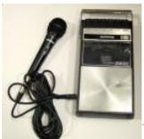
Breathalyzer Microphone using an Arduino The breathalyzer microphone is a system for the inconspicuous collection of blood-alcohol content level data sets. In other words, you can measure a person's sobriety with a device, that for all intents and purposes, looks no different than a standard microphone. This tool adds new..... Listed under: Medical – Health based Projects, Projects, Sound – Audio Projects
