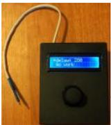
Intervalometer for Sony NEX 5n This intervalometer used infrared LED To built intervalometer you need: Arduino Nano (or Arduino-compability). I used Nano V3 Serial LCD Joystick Module IR Led and resistor ~200 Ohm Switch Push Button Plastic enclosure Battery 9V Schematic is very simple Step 2: Connection Serial LCD has..... Listed under: Metering – Instrument Projects
