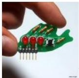
340. Blinky Fish using an Arduino Assembly instructions for an add-on board for the Arduino. \*\*\*\* FOR INSTRUCTIONS FOR MARCH 2013, KICKSTARTER PROJECT GO HERE <http://www.instructables.com/id/Blinky-Fish-Kickstarter-Project/> \*\*\*\*\* It has some LED's and a button. It connects to digital pins 9-13 and ground. My hope is that this will be useful to people that want to..... Listed under: Game – Entertainment Projects, LED Projects, Projects
