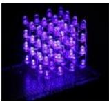
4x4x4 LED-cube based Arduino and Flower protoboard This instructable will teach you how to build your 4x4x4 LED cube with Flower ProtoBoard and control by Arduino. Why is Flower ProtoBoard ? not ProtoBoard ? Because of I often use protoboards to test out if a new idea works in practice. I do not use..... Listed under: Game – Entertainment Projects, Home Automation Projects, LED Projects, Projects
