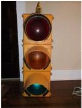
629. WAVEbuoy using Arduino The WAVEbuoy is a arduino lamp connected to the internet that displays the current wave height of any of the National Data Buoy Centre's wave buoys. This lamp is currently connected to the Sevenstones Lightship buoy that gives an indication of swell approaching Cornwall in..... Listed under: Home Automation Projects
