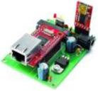
Arduino DDNS (Dynamic DNS) by Open-Electronics.org This device captures the IP address of your network and it publish on site DynDNS.com. All without PC. It allow a remote access to your LAN even if the IP address of the connections changes. For logistics reasons the provider can not assign a IP..... Listed under: Internet – Ethernet – LAN Projects, Projects
