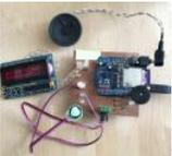
Talking Arduino Heart Rate Monitor My partner and I wanted to make heart rate monitor that does more than simply measure a user's heart rate. Our heart rate monitor talks! Each button gives a verbal description of its functionality and makes the measurements visible on the screen. This monitor will..... Listed under: Medical – Health based Projects
