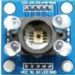
How to Build a Color Sensor Circuit In this project, we are going to build a color sensor circuit with an Arduino microcontroller. A color sensor is a device that can detect and differentiate between certain primary colors. This sensor can detect and differentiate between the colors white, blue, green, and red..... Listed under: How To – DIY – Projects, Sensor – Transducer – Detector Projects
