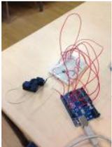
558. Connect the arduino and make the speaker play To make your Arduino to play a melody you need these accessories. One 5 ohm speaker One Arduino uno board One Push button One 10 kohm resistor 8 leds And a lot of core wires Step 1: Connect the arduino and make the speaker play This..... Listed under: Sound – Audio Projects
