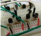
Arduino MicroBot Project Steps On the breadboard, build two bi-directional motor control circuits (also known as "H-bridge") circuits. These circuits will control the two DC motors that drive the wheels. Each circuit will have two wires from the Arduino (one for forward, one for backward) to control the..... Listed under: Robotics – Automation Projects
