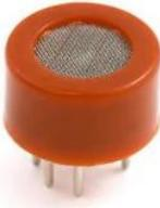
MQ-3 Alcohol Sensor Circuit Built with an Arduino In this project, we will go over how to build an alcohol sensor with an arduino. The alcohol sensor we will use is the MQ-3 sensor. This is a sensor that is not only sensitive to alcohol, particularly ethanol, which is the type of alcohol..... Listed under: Sensor – Transducer – Detector Projects
