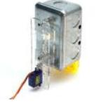
Easy DIY Home Automation (using servo switches) using arduino This Instructable is all about one of life's simple actions, flipping a light switch on and off. At oomlout we do it many times a day, so many in fact it came to a point where we asked ourselves "Can't we get an Arduino to..... Listed under: Home Automation Project Ideas
