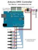
**Small Arduino DMX controller** In this post we show you how to make a small and useful Arduino DMX512 controller, which can use by example to handle a smoke machine with DMX, or as test equipment, etc... We can use Arduino Mega, Arduino UNO, and other with small changes..... Listed under: Sensor – Transducer – Detector Projects
