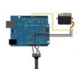
Knob Control the position of a RC (hobby) servo motor with your Arduino and a potentiometer. This example makes use of the Arduino servo library. Hardware Required Board (1) Servo Motor (1) Potentiometer hook-up wire Circuit Servo motors have three wires: power, ground, and signal..... Listed under: Motor Projects
