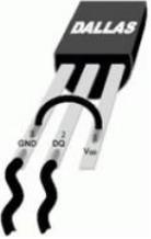
Temperature Sensing using DS18B20 Digital Sensors Note: When referring to Arduino below, this works in the same way on the emonTx which is arduino-based. The DS18B20 is a small thermometer with a built in 12bit ADC; it can be easily connected to Arduino digital input. The sensor communicates over a one-wire..... Listed under: Sensor – Transducer – Detector Projects
