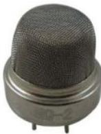
MQ-2 Smoke Sensor Circuit Built with an Arduino In this project, we will go over how to build a smoke sensor circuit with an arduino board. The smoke sensor we will use is the MQ-2. This is a sensor that is not only sensitive to smoke, but also to flammable gas. The MQ-2..... Listed under: Sensor – Transducer – Detector Projects
