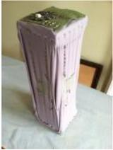
556. New Textiles 2012 using arduino Twist Switch by ttseng Through the action of twisting, swathes of conductive fabric are folded in upon each other, completing a circuit that then turns on LEDs. On each face of stretched spandex are swathes of conductive fabric. Before choosing which swathes to designate as..... Listed under: LED Projects
