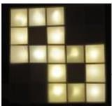
382. Yet Another Daft Punk Coffee Table (5x5 LED Matrix) using arduino Yes, I know this has been done before, but I wanted to build my own, using as few parts as possible. I built this as a table top or wall mount model, but it can be scaled up to make a coffee table. I built..... Listed under: LED Projects
