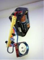
YAHMS: Temperature Probes My wireless temperature probes work by using an Xbee module to transmit readings from a TMP36 down to the Arduino base station. The XBees aren't too cheap, coming in around £19 or \$23 so I tried to be cheap and ordered mine from Sparkfun, I..... Listed under: Temperature Measurement Projects
