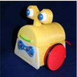
Sensor Less 3d Printed Robot Tyree (he wears a tie and he has tires) actually smiles after he bumps into something (see video). Using an Arduino motor shield, he detects obstacles using the "more current into the motor means something is in the way" principle. Tyree started out as a..... Listed under: Robotics – Automation Projects, Sensor – Transducer – Detector Projects
