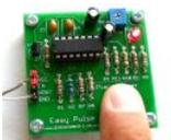
A DIY photoplethysmographic sensor for measuring heart rate Meet Easy Pulse: A kit that includes all it needs to make a DIY heart rate sensor. Although it is not built using an Arduino, it is still open and easy to build. From the site: "This project is based on the principle of photoplethysmography..... Listed under: Sensor – Transducer – Detector Project Ideas
