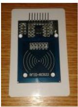
Arduino RFID Reader RC522 + Access Control System I just received my RC522 RFID reader and made this simple Arduino access control system that uses the reader, a buzzer for the alarm and a relay shield for the security system. The relay can be used to open a door lock and if you..... Listed under: RFID - NFC projects
