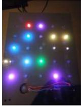
5x5 rgb lpd6803-led matrix arduino controlled what: a 5\*5 rgb led matrix, made with arduino and lpd6803 based leds from adafruit. with an pir sensor, it goes on if it detects movements and a ir distace sensor, 1 animation shows the distance you have from the sensor :). why: because its..... Listed under: LED Projects, Projects
