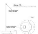
R.O.V.E.R.: Reactive Observant Vacuous Emotive Robot using arduino R.O.V.E.R. is an autonomous robot. He was built and designed as an interactive art installation specifically for the MAT EoYS 2013. He navigates the space with a heat array and bump sensors and interacts with attendees. When R.O.V.E.R. recognizes that a person is present he..... Listed under: Electronics News Updates, Robotics - Automation Project Ideas
