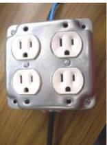
Yet Another Arduino 110v Power Controller This Instructable shows you how to build a four-gang outlet box in which each outlet is controlled via an Arduino (or any other level signals). It differs from the other relay boxes in that it uses no circuit boards and has very few parts (one..... Listed under: Projects, Solar energy projects
