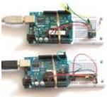
742. DIY Amp / Watt Hour Volt Meter – Arduino Major corrections and additions made 9/9/2014 For my off-grid Ham Radio and Solar projects, I needed a way to measure volts, amps, watts, amp hours and watt hours. There's a couple of commercial products that can do this, but not with the flexibility I wanted..... Listed under: How To – DIY – Projects, Metering – Instrument Projects
