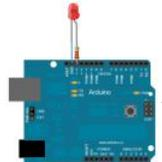
**Blink** This example shows the simplest thing you can do with an Arduino to see physical output: it blinks an LED. Hardware Required Arduino Board LED Resistor, anything between 220 ohm to 1K ohm Circuit To build the circuit, connect one end of the resistor to..... Listed under: LED Projects
