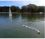
Make a swimming Robo-Snake Sneel is the name of my snake / eel swimming robot. This is documentation of hardware, software and mechanical design of Sneel\_003. urethane flex tubing, microcontrollers, Zigbee wireless radio, hose clamps, wires, servo motors, titanium servo brackets, silicon, marine grease, epoxy, pond pump Sneel is..... Listed under: Robotics – Automation Projects
