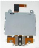
369. Arduino + Laptop Touchpad using arduino Yes, this is more or less your average touchpad that one can find from inside a laptop. This model, like majority of touchpads out there operates with PS/2 standard. This means that it can be directly plugged in to a PS/2 connector and with proper..... Listed under: Sensor – Transducer – Detector Project Ideas
