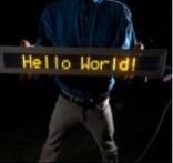
PS/2/You: Go-anywhere, LED digital message board using Arduino microcontroller Combine three inexpensive LED matrix display panels, an Ardweeny microcontroller and a standard PS/2 computer keyboard into your own go-anywhere, instantly updatable 768-pixel digital message board. The code can hold up to six lines of text with a maximum of 100 characters each. Pressing a..... Listed under: LED Projects
