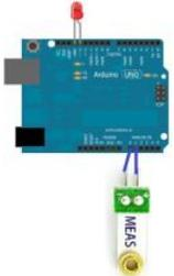
How to Build a Vibration Detector Circuit In this project, we will go over how to build a vibration detector circuit. This is a circuit which can detect and measure flex, touch, vibration, and shock. The sensor we will use to detect these movements is a piezo vibration sensor from Measurement Specialists (MEAS). The..... Listed under: Sensor – Transducer – Detector Projects
