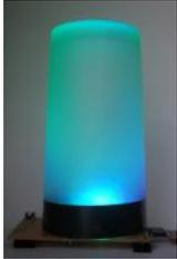
796. Arduino multi-mode lamp with soft touch switch In this Arduino-based project, we will build a lamp with multiple light displays: color sequencer, dimming light, color chaser, firelight - all selected by a touch bar on the circuit board. All the functions are done in software, including the touch sensor, which is a..... Listed under: Home Automation Projects, LED Projects, Projects
