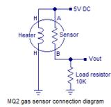
LPG sensor using arduino LPG sensor using arduino with alarm and cutoff. A simple LPG sensor using arduino is shown in this article. This circuit indicates the amount of LPG in the air. The circuit sounds an alarm and trips a relay when the concentration is above a predetermined..... Listed under: Sensor – Transducer – Detector Projects
