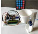
Automatic Pet Feeder using Arduino Today we are building an Arduino based Automatic Pet Feeder which can automatically serve food to your pet timely. It has a DS3231 RTC (Real Time Clock) Module, which used to set time and date on which your pet should be given food. So, by..... Listed under: Clock – Timer Projects
