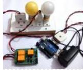
**DIY Arduino Relay Driver Shield** In this DIY project we make a 3-Channel Arduino Relay Shield Circuit for relay based applications. We designed an isolated PCB for 3 relays. By using this Arduino Relay Shield, we can operate 3 AC appliances at a time. We have put a two pin screw terminal blocks (Neutral, NO)..... Listed under: Other Projects
