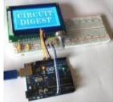
Interfacing Graphical LCD (ST7920) with Arduino There are many types of LCDs used in Electronic Projects. We have already used 16X2 LCD in many of our projects and also used TFT LCD with Arduino. You can find our entire 16X2 LCD related project by following this link, including interfacing with 8051, AVR, Arduino and many..... Listed under: LCD Projects
