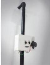
How to make a Smart Cane for the Visually Impaired with Arduino I wanted to make something for them to help the visually impaired become independent, so I created an open source Arduino project for a Smart Cane. This Arduino smart cane can assist with walking alone in new environments by taking inputs through an obstacle sensor..... Listed under: Other Projects
