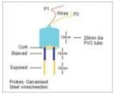
Digital Soil Moisture Meter A digital soil moisture meter is used for indicating the water content of a given soil sample. [caption id="attachment\_31551" align="alignright" width="300"] Soil moisture sensor head[/caption] As crop production requires water at different stages and in different amounts, it is important to measure soil moisture..... Listed under: Metering – Instrument Projects
