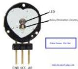
Pulse Sensor and Arduino – Interfacing In this article, we are going to interface a Pulse Sensor with Arduino. The pulse sensor we are going to use is a plug and play heart rate sensor. This sensor is quite easy to use and operate. Place your finger on top of the sensor..... Listed under: Sensor – Transducer – Detector Projects
