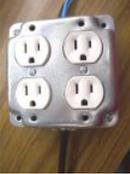
Yet Another Arduino 110v Power Controller This Instructable shows you how to build a four-gang outlet box in which each outlet is controlled via an Arduino (or any other TTL level signals). It differs from the other relay boxes in that it uses no circuit boards and has very few parts (one..... Listed under: Projects, Solar energy projects
