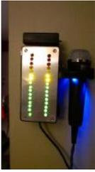
Boozeduino using arduino Now with more LED. Arduino mega powered breathalyser using the MQ-3 sensor. A relative gauge for judging how intoxicated you are. NOT TO BE USED AS MEANS OF BREATHALYZING NEVER DRINK AND DRIVE. This is more of a device to encourage one to drink..... Listed under: LED Projects
