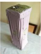
168. New Textiles 2012 using arduino Twist Switch by ttseng Through the action of twisting, swatches of conductive fabric are folded in upon each other, completing a circuit that then turns on LEDs. On each face of stretched spandex are swatches of conductive fabric. Before choosing which swatches to designate as..... Listed under: LED Projects
