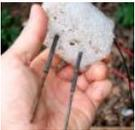
162. The Soil Moisture Sensor using arduino You are building a cheap soil moisture sensor so the brain can read the amount of moisture in the soil. The version we are building is very low tech, but it is also very cheap and easy to build. It consists of a block of..... Listed under: Home Automation Projects, Temperature Measurement Project Ideas
