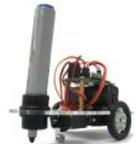
477. Building a Doodle Bot kit from DAGU Doodle Bot is a very simple beginners robot that can write messages using white board markers, jumbo chalk or crayons: The kit comes with all parts including an Arduino compatible controller and a screwdriver. You will need to supply 4x AAA batteries and a suitable..... Listed under: Robotics – Automation Projects
