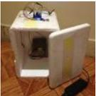
Cheap Arduino Controled Yogurt Maker These days I was reading an interesting post on how to make yogurt "by the gallon" (<http://www.instructables.com/id/Yogurt-By-The-Gallon/>). One thing needed was to maintain a rather constant temperature of 43°C (110°F), so the bacteria ca grow properly. Though you can buy commercial yogurt makers, they aren't..... Listed under: Home Automation Projects, Projects
