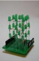
3x3x3 LED cube shield using arduino What should be in your kit: 1 – PCB 27 – LED's 2 – 6 Pins for Arduino 2 – 8 Pins for Arduino 3 – Resistors 1 – Foam Guide 1 Small Wire 1 – Medium Wire 1 – Large Wire You will..... Listed under: LED Projects
