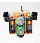
Haptic Proximity Module (HPM) for Low Vision users The Haptic Proximity Module (HPM) seeks to enable people with low vision, or other vision impairments, engage with their direct surroundings through vibration feedback from a range detector, and do so cheaply with readily available components. The aim of thi instructables is to share..... Listed under: Development Board – Kits Projects
