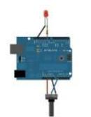
Pulse Width Modulation : PWM using Arduino Pulse Width Modulation or PWM is a method of Digital to Analog Conversion. It helps in delivering analog average voltage using digital pulses of variable pulse width. By controlling the on time and off time, we can generate an analog average voltage using the digital..... Listed under: PWM Projects
