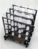
LED Cube Spectrum Analyzer In this project we'll create a small add-on PCB containing the a MSGEQ7 spectrum analyzer circuit and show how it can drive the RGB LED cube kit from Freertronics. This allows the cube to display the seven bands over four horizontal planes. There is a small amount..... Listed under: LED Projects
