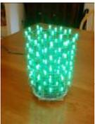
LED Cylinder using Arduino This is a little art project I made with 95 RGB LEDs arranged in a 3D cylinder shape, sitting atop a microcontroller-based driver circuit. The LEDs are individually addressable, and when you power it on, the software cycles through a series of animations, e.g. various..... Listed under: Games – Entertainment Projects, Home Automation Projects, LED Projects, Projects
