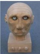
211. Arduino controlled animatronic wooden head (reading lamp) using Arduino This head is a reading lamp which can be adjusted for direction of lighting, and dimmed as required. This Instructable combines Arduino programming, some simple electronics, carving with hand and power tools, mechanical control and bit of woodwork. Apart from the Arduino and a..... Listed under: Home Automation Projects
