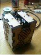
Arduino PCR (thermal cycler) for under \$85 This tutorial will show you how to make a thermal cycler from scratch for about \$85. In short, PCR (polymerase chain reaction) amplifies bits of DNA, creating millions of copies of a target sequence. You can use it to test a DNA sample for a..... Listed under: How To – DIY – Projects
