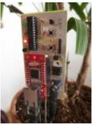
395. Arduino DDNS (Dynamic DNS) by Open-Electronics.org This device captures the IP address of your network and it publish on site DynDNS.com. All without PC allow a remote access to your LAN even if the IP address of the connections changes. For logistics reasons the provider can not assign a IP..... Listed under: Internet - Ethernet - LAN Projects, Projects
