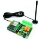
TiDiGino, the Arduino-based GSM remote control Using an ATmega 2560 and therefore the heart of Arduino, we have developed a universal remote control w GSM. This allows to control 2IN/2OUT, DTMF key, gate control and GSM thermostat activated remotely. We have already presented several remote control wit different functions. But now..... Listed under: Phone Projects, Radio Projects
