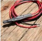
The Soil Temperature Sensor using arduino You are building a soil temperature sensor. We need a waterproof thermometer that we can burry in the soil. The sensor is made up of a small circuit enclosed in a piece of heat shrink (to waterproof it). Supplies: (see the parts page) an LM335..... Listed under: Home Automation Projects, Temperature Measurement Projects
