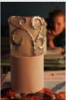
**Magic Light (Capacitance Sensor, First Arduino Project)** This was my very first arduino project. Its great for beginners. Fade the color or the lights my moving your hands near it. It fades from a pretty purple blue to a firey red-orange. Its was SUPER easy to build, not to hard to write..... Listed under: Sensor – Transducer – Detector Projects
