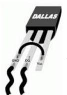
**Temperature Sensing using DS18B20 Digital Sensors** Note: When referring to Arduino below, this works in the same way on the emonTx which is arduino-based The DS18B20 is a small thermometer with a built in 12bit ADC; it can be easily connected to Arduino digital input. The sensor communicates over a one-wire.. Listed under: Sensor – Transducer – Detector Projects
