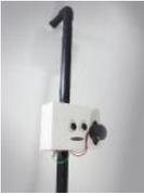
How to make a Smart Cane for the Visually Impaired with Arduino I wanted to make something for them to help the visually impaired become independent, so created an open source Arduino project for a Smart Cane. This Arduino smart cane can assist with walking alone in new environments by taking inputs through an obstacle sensor..... Listed under: Other Projects
