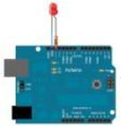
**Blink** This example shows the simplest thing you can do with an Arduino to see physical output: it blinks an LED. Hardware Required Arduino Board LED Resistor, anything between 220 ohm to 1K ohm Circuit To build the circuit, connect one end of the resistor to..... Listed under: LED Projects
