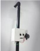
How to make a Smart Cane for the Visually Impaired with Arduino I wanted to make something for them to help the visually impaired become independent. I created an open source Arduino project for a Smart Cane. This Arduino smart cane can assist with walking alone in new environments by taking inputs from an obstacle sensor..... Listed under: Other Projects
