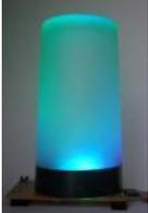
Arduino multi-mode lamp with soft touch switch In this Arduino-based project, we will build a lamp with multiple light displays: color sequencer, dimmin color chaser, firelight - all selected by a touch bar on the circuit board. All the functions are done in software, including the touch sensor, which is a..... Li under: Home Automation Projects, LED Projects, Projects
