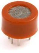
707. **MQ-2 Smoke Sensor Circuit Built with an Arduino** In this project, we will go over how to build a smoke sensor circuit with an arduino board. The smoke sensor we will use is the MQ-2. This is a sensor that is not only sensitive to smoke, but also to flammable gas. The MQ-2..... Listed under: [Sensor – Transducer – Detector Projects](#)
