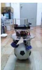
How to make a Ball Balancing Robot Last year, I have made this ball balancing robot.It can stand on a ball stable by the balance system of itself. There is one connect point between the robot and the ground, so it is more flexible than the traditional wheeled robot. It can..... Listed under: Robotics – Autom Projects
