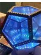
Infinite Disco In this project, I made an infinity mirror based on a dodecahedron that reacts to sound . Step 1: Materials Essential materials: Arduino Uno thick 100x50cm MDF2mm thick 100x50cm plexiglass3 meter WS2812B LEDstrip 60 LEDs/mSound Detection Sensor Module 3-PINThin electric wire (10isl total)BreadboardPerfboard/stripboardSimple rectangular..... Listed under: LED Projects
