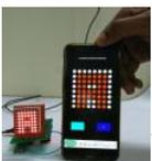
Bluetooth Controlled 8x8 LED Matrix Sign Board Display using Arduino Be it the long stretched highways or your doctors front door, we have sign board everywhere to provide us information. But these sign boards are often boring and cannot be configured as per our interest from time to time. So in this we..... Listed under: LED Projects
