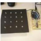
601. **Smart Aquarium** The goal of our project is to display the status of a previously implemented smart aquarium. The previously implemented system included external power supply, Arduino Uno, Ethernet Shield, ULN2803 driver, 4 120V AC relays, and 4 controlled 120V AC receptacles, and a servo motor..... Listed under: Game – Entertainment Projects
