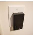
The Ultimate Light Switch The goal of this instructable is to explain how I made a wifi-connected light switch (also called remotes further). The goal of the remotes is to turn on and off several wifi-connected relays. The relays are not explained in this instructable. They are explained in..... Listed under: LED Projects
