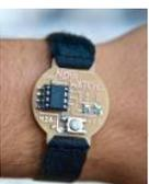
The Nerd Watch Hello! Welcome to another Other Machine project tutorial! I'm Sam DeRose, a former Other Machine Co. Summer Intern. I created the Nerd Watch last summer while working at OMC. The Nerd Watch displays the time in binary when the button is pushed. The watch shows the..... Listed under: Timer Projects
