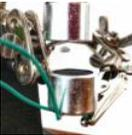
Mini Acoustic Levitation View this project on my website to see a circuit simulation and a video! Acoustic levitation is made possible through the fact that behaves as a wave. When two sound waves intersect each other, they can either constructively or destructively interfere with each other. (This is..... List under: Sound – Audio Projects
