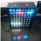
Dutch 8x8 Neopixel Word Clock A friend introduced me to neopixels (WS2812) programmable LED's. That would be great for my word clock, so I re-did it. It is very much a mixup with a slightly different size and code. The 8x8 WS2812 modules are also cheaper than the colorduino,..... Listed under: Clock - 7 Projects
