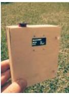
Portable Luxmeter This project is about making portable luxmeter. It can be used in schools, where children can measure different kinds of light sources.Functions: 1. measure intensity of light in lux. 2. calculate solar irradiation from lux to watts/m2 (factor 112) 3. charging battery using USB port..... Listed under: Battery Projects
