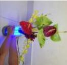
Interactive Cylindrical Cube This is a creative cylindrical LED cube with proximity sensing by infrared led and photo-transistors. Interactive Cylindrical Cub includes: 8X8 royal blue LEDs, 12 infrared LEDs, 16 photo-transistors and all of them are bent & formed a cylindrical shape. Please see video below wher Listed under: LED Projects
