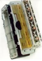
The Photometric Camera and the CCDs The Photometric System The photometric camera for the SDSS consists of two TDI scanning CCD arrays, one, using Tektronix/SiTe 2048 x 2048 CCDs in a 5 by 6 array for five-color photometry, and the other using 24 2048 x 400 chips for astrometry and..... Listed under - Camera - Imaging Projects
