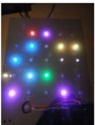
76. 5x5 rgb Ipd6803-led matrix arduino controlled what: a 5\*5 rgb led matrix, made with arduino and Ipd6803 based leds from adafruit. with an pir sensor, on if it detects movements and a ir distace sensor, 1 animation shows the distance you have from the sensor :). why: because its..... Listed under: LED P Projects
