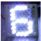
How to make a LED 7-segment display with or without Arduino I'm going to show you how to make a 7 segment display with LEDs. Combine with Arduino create countdown timers, simple text, and more. I like to make original projects. I searched the whole of instructables and didn't find one like this. In fact Listed under: LED Projects
