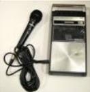
Breathalyzer Microphone using an Arduino The breathalyzer microphone is a system for the inconspicuous collection of blood-alcohol content level data. In other words, you can measure a person's sobriety with a device, that for all intents and purposes, looks no different than a standard microphone. This adds new..... Listed under: Medical – Health based Projects, Projects, Sound – Audio Projects
