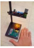
Build Your Own Sourcemeter This is an explanation and set of building plans for a USB-powered sourcemeter with a personal computer interface. The sourcemeter uses an open-source Arduino microprocessor and the user interface uses the open-source Processing environment. The sourcemeter was designed as a homemade current-voltage (IV) tester to measure the IV..... Listed under: Metering - Instrument Projects
