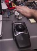
Proximity sensing mouse wheel scroller using Arduino List of tools: 1. Exacto 2. Arduino Nano / USB chord (Mini-B) 3. Dremel / Drill 4. Paper & Pencil 5. S Sensor (2Y0A21 F) 6. Hot glue gun 7. Solder gun / Solder 8. A small mirror Ok so you might ask, why..... Listed under: Projects, Sensor – Transducer – Det Projects
