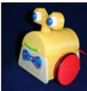
**Sensor Less 3d Printed Robot Tyree** (he wears a tie and he has tires) actually smiles after he bumps into something (see video). Using an Arduino motor he detects obstacles using the "more current into the motor means something is in the way" principle. Tyree started out as a..... Listed under: Robotics - Automation Projects, Sensor – Transducer – Detector Projects
