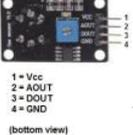
MQ-8 Hydrogen Gas Sensor Circuit Built with an Arduino In this project, we will go over how to build a hydrogen gas sensor circuit with an arduino. The hydrogen gas sensor we will use is the MQ-8 sensor. This is a sensor that is sensitive to effects of hydrogen gas. Hydrogen gas (H2), at..... Listed under: 9 Transducer – Detector Projects
