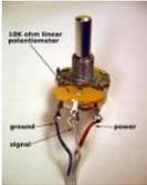
Analog Sensors using arduino Analog sensors produce an analog (continuous) voltage that typically varies from 0 to 5 volts. They have three wires – ground, power, and signal (typically red, black, and white, respectively). Examples shown below include: Potentiometers Proximity Accelerometers Ribbon Bend Flex Light Temperature Sound Multi-touch Touch..... Listed under: Sensor – Transducer – Detector Projects
