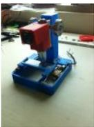
Low cost digital microscope with automated slide movement using arduino This is an easy-to-implement product modification that will be extremely useful for clinicians, pathologists, researchers or other microscopy enthusiasts interested in capturing whole slide images or creating virtual slides for later use. This allows one to take multiple images of the slide under high..... Listed under: Medical – Health based Projects
