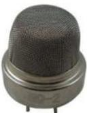
MQ-2 Smoke Sensor Circuit Built with an Arduino In this project, we will go over how to build a smoke sensor circuit with an arduino board. The smoke s we will use is the MQ-2. This is a sensor that is not only sensitive to smoke, but also to flammable gas. The MQ-2..... Listed under: Sensor - Transducer - Detector Projects
