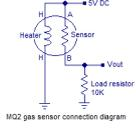
LPG sensor using arduino LPG sensor using arduino with alarm and cutoff. A simple LPG sensor using arduino is shown in this article. This circuit indicates the amount of LPG in the air. The circuit sounds an alarm and trips a relay when the concentration is above a predetermined level. Listed under: Sensor – Transducer – Detector Projects
