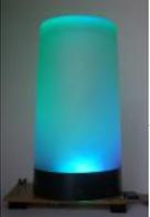
Arduino multi-mode lamp with soft touch switch In this Arduino-based project, we will build a lamp with multiple light displays: color sequencer, dimming color chaser, firelight - all selected by a touch bar on the circuit board. All the functions are done in software, including the touch sensor, which is a..... Li under: Home Automation Projects, LED Projects, Projects
