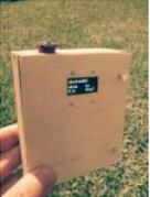
Portable Luxmeter This project is about making portable luxmeter. It can be used in schools, where children can measure different kinds of light sources.Functions: 1. measure intensity of light in lux. 2. calculate solar irradiation from lux to watts/m2 (factor 112) 3. charging battery using USB port... Listed under: Battery Projects
