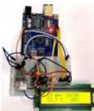
Reef Controller A Reef / Saltwater Aquarium controller based on an Arduino Mrk1000 and controlled remotely by an Universal Windows Platform app. Things used in this project Hardware components Arduino MKR1000 × 1 Adafruit Perma-proto board full size × 1 Adafruit I2C logic level converter × 1..... Listed under: LED Projects, Projects, Temperature Measurement Projects
