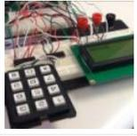
The objective of our project was to create an alarm system that could detect an intruder using an IR motion sensor. We used a keypad so the user could enter their password to arm and disarm the system. [gallery columns="2" size="medium" ids="31154,31155"] We also included..... Listed under: [Clock – Timer Projects](#)
