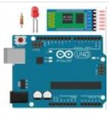
Ever thought of controlling any electronic devices with your smart phone ?Controlling your robot or any other devices with your smartphone will be really cool. Here is a simple and basic tutorial for interfacing Bluetooth with arduino Step 1: Things You Need Hardware Bluetooth Module HC 05/06ArduinoLED220Ω ResistorAndroid device..... Listed under: [Bluetooth Projects](#)
