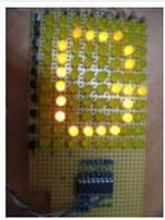
UPDATE 1: I HAVE ADDED THE CODE FOR CONWAY'S GAME OF LIFE UPDATE 2: NOW YOU CAN SAVE SOME ARDUINO PINS WITH THE HELP OF 1 SHIFT REGISTER. In this instructable I will show you how to build a quite fancy 8 by 10 L.E.D matrix(with scrolling text and animations) using the Arduino and 4017 decade..... Listed under: [LED Projects](#)
