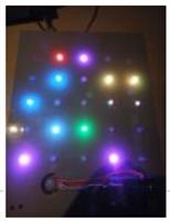
what: a 5\*5 rgb led matrix, made with arduino and lpd6803 based leds from adafruit. with an pir sensor, it goes on if it detects movements and a ir distace sensor, 1 animation shows the distance you have from the sensor :). why: because its..... Listed under: [LED Projects](#), [Projects](#)
