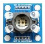
In this project, we are going to build a color sensor circuit with an Arduino microcontroller. A color sensor is a device that can detect and differentiate between certain primary colors. This sensor can detect and differentiate between the colors white, blue, green, and red..... Listed under: [How To – DIY – Projects](#), [Sensor – Transducer – Detector Projects](#)
