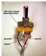
Analog sensors produce an analog (continuous) voltage that typically varies from 0 to 5 volts. They have three wires – ground, power, and signal (typically red, black, and white, respectively). Examples shown below include: Potentiometers Proximity Accelerometers Ribbon Bend Pressure Light Temperature Sound Multi-touch Touch..... Listed under: [Sensor – Transducer – Detector Projects](#)
