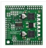
This shield makes it easy to control two brushed DC motors with your Arduino or Arduino-compatible board. Its dual MC33926 motor drivers operate from 5 to 28 V and can deliver a continuous 3 A per motor. These great drivers also offer current-sense feedback and accept ultrasonic..... Listed under: [Motor Projects](#)
