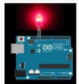
In this project, we will go over how to build a night light circuit using an arduino. A night light circuit is a circuit which will turn on when nighttime comes, which is when it gets dark and the place could use some illumination. It..... Listed under: [How To – DIY – Projects](#), [LED Projects](#)
