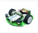
The idea Ardusumo is a universal platform to build robots on wheels that can move around avoiding obstacles using infrared sensors and follow routes marked with dark lines on a white background. We have created Ardusumo to bring young students to the world of robotics:..... Listed under: [Projects](#), [Robotics – Automation Projects](#)
