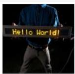
Combine three inexpensive LED matrix display panels, an Ardweeny microcontroller and a standard PS/2 computer keyboard into your own go-anywhere, instantly updatable 768-pixel digital message board. The code can hold up to six lines of text with a maximum of 100 characters each. Pressing a..... Listed under: [LED Projects](#)
