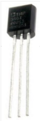
In this project, we will demonstrate how to build temperature sensor circuit using a TMP36 sensor. As a temperature sensor, the circuit will read the temperature of the surrounding environment and relay the temperature to us back in degrees fahrenheit. The IC we will use..... Listed under: [Sensor – Transducer – Detector Projects](#)
