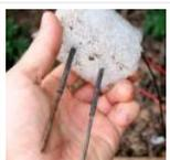
You are building a cheap soil moisture sensor so the brain can read the amount of moisture in the soil. The version we are building is very low tech, but it is also very cheap and easy to build. It consists of a block of..... Listed under: [Home Automation Projects](#), [Temperature Measurement Project Ideas](#)
