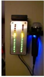
Now with more LED. Arduino mega powered breathalyser using the MQ-3 sensor. A relative gauge for judging how intoxicated you are. NOT TO BE USED AS MEANS OF BREATHALYZING NEVER DRINK AND DRIVE. This is more of a device to encourage one to drink..... Listed under: [LED Projects](#)
