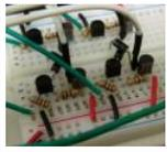
Steps On the breadboard, build two bi-directional motor control circuits (also known as “H-bridge”) circuits. These circuits will control the two DC motors that drive the wheels. Each circuit will have two wires from the Arduino (one for forward, one for backward) to control the..... Listed under: [Robotics – Automation Projects](#)
