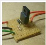
Intro The Arduino microcontroller board is able to supply a current of 40mA from its output connections. These digital outputs are fixed at 5V "ON" or 0V "OFF". This is adequate for working with LEDs but devices such as motors, solenoids, high brightness LEDs etc..... Listed under: [Motor Projects](#)
