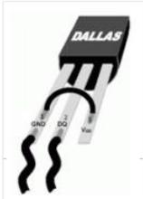
Note: When referring to Arduino below, this works in the same way on the emonTx which is arduino-based. The DS18B20 is a small thermometer with a built in 12bit ADC; it can be easily connected to Arduino digital input. The sensor communicates over a one-wire..... Listed under: [Sensor – Transducer – Detector Projects](#)
