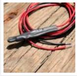
You are building a soil temperature sensor. We need a waterproof thermometer that we can burry in the soil. The sensor is made up of a small circuit enclosed in a piece of heat shrink (to waterproof it). Supplies: (see the parts page) an LM335..... Listed under: [Home Automation Projects](#), [Temperature Measurement Projects](#)
