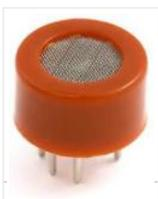
In this project, we will go over how to build an alcohol sensor with an arduino. The alcohol sensor we will use is the MQ-3 sensor. This is a sensor that is not only sensitive to alcohol, particularly ethanol, which is the type of alcohol..... Listed under: [Sensor – Transducer – Detector Projects](#)
