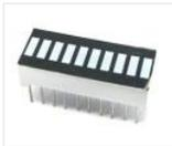
Introduction This project explores a couple of ways of simulating and using a bar graph with the Arduino. Bar graph components like the following one can be used, This type of bar graph is basically just 10 LEDs in a row with anodes on one..... Listed under: [Other Projects](#)
