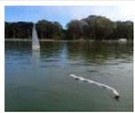
Sneel is the name of my snake / eel swimming robot. This is documentation of hardware, software and mechanical design of Sneel\_003. urethane flex tubing, microcontrollers, Zigbee wireless radio, hose clamps, wires, servo motors, titanium servo brackets, silicon, marine grease, epoxy, pond pump Sneel is..... Listed under: [Robotics – Automation Projects](#)
