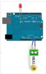
In this project, we will go over how to build a vibration detector circuit. This is a circuit which can detect and measure flex, touch, vibration, and shock. The sensor we will use to detect these movements is a piezo vibration sensor from Measurement Specialists (MEAS). The..... Listed under: [Sensor – Transducer – Detector Projects](#)
