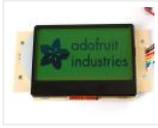
What it is... Type: Graphical (128×64) monochrome LCD with LED backlight Interface: Serial / SPI This is a good time to read the datasheet Available from: Adafruit, of course! Introduction: This mini-tutorial will go through the process of setting up a ST7565 LCD. These LCDs..... Listed under: [LCD Projects](#)
