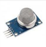
In this article, we are going to learn how to interface MQ2 Gas Sensor with Arduino. MQ2 is basically a general purpose gas sensor (similar to MQ5) which can sense a broad range of gases like LPG, Butane, Methane(CH4), Hydrogen and in addition to these..... Listed under: [Sensor – Transducer – Detector Projects](#)
