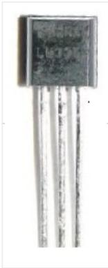
In this project, we will demonstrate how to build temperature sensor circuit using a LM335 sensor. As a temperature sensor, the circuit will read the temperature of the surrounding environment and relay this temperature to us back in degrees Kelvin. The difference between an LM335..... Listed under: [Sensor – Transducer – Detector Projects](#)
