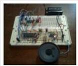
Here's the Arduino version of a project to use the General Instruments (GI) SP0256-AL2 vintage speech synthesis chip to say "hello world". I'd previously shown how to do this with a Basic Stamp 2. Here's what it sounds like saying, "hello world" 20101215\_164333.mp3 How it..... Listed under: [Development Board – Kits Projects](#)
