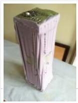
Twist Switch by ttseng Through the action of twisting, swatches of conductive fabric are folded in upon each other, completing a circuit that then turns on LEDs. On each face of stretched spandex are swatches of conductive fabric. Before choosing which swatches to designate as..... Listed under: [LED Projects](#)
