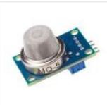
In this guide, we learn how to interface MQ5 Gas sensor (which is a generic Gas Sensor more suited to detect and determine LPG concentrations) with Arduino. In this tutorial, we are using the MQ5 Gas sensor module (which is widely available in market) ..... Listed under: [Sensor – Transducer – Detector Projects](#)
