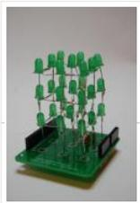
What should be in your kit: 1 – PCB 27 – LED's 2 – 6 Pins for Arduino 2 – 8 Pins for Arduino 3 – Resistors 1 – Foam Guide 1 – Small Wire 1 – Medium Wire 1 – Large Wire You will..... Listed under: [LED Projects](#)
