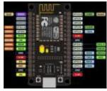
A guide to getting started with the ESP8266 with the Arduino IDE This assumes that yo have a NodeMCU type board with the Silicon Labs CP2102 USB to UART Bridge. These boards are convenient because they can be connected directly to your computer for progammng..... Listed under: [Interfacing\(USB – RS232 – I2c -ISP\) Projects](#)
