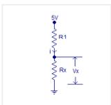
Auto ranging ohmmeter using arduino. This article is about a simple auto ranging ohmmeter using arduino. The measured resistance is displayed using a 16×2 LCD display. The circuit is sufficiently accurate and uses minimum number of external components possible. Before going into the details of..... Listed under: [Metering – Instrument Projects](#)
