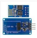
The ESP8266 is a great tool for enabling your project to access the internet. You can plug it into an Arduino easily as shown and allow your project to communicate through the internet. Or even more exciting, to control it from anywhere in the world!..... Listed under: [Other Projects](#)
