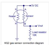
LPG sensor using arduino with alarm and cutoff. A simple LPG sensor using arduino is shown in this article. This circuit indicates the amount of LPG in the air. The circuit sounds an alarm and trips a relay when the concentration is above a predetermined..... Listed under: [Sensor – Transducer – Detector Projects](#)
