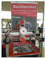
The objective of this instructable is to guide your way through the entire making process of building a BuildersBot machine. An open design Arduino Controlled CNC Router that can also perform 3D printing. The instructions will cover all areas such as design, mechanics, electronics and..... Listed under: [CNC Machines Projects](#)
