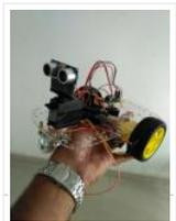
This project is designed to build a robot that automatically detects the obstacle on its path and guides itself whenever an obstacle comes ahead of it. This robotic vehicle is built, using Arduino UNO board. An ultrasonic sensor is used to detect any obstacle ahead..... Listed under: [Robotics – Automation Projects](#)
