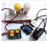
In this DIY project we make a 3-Channel Arduino Relay Shield Circuit for relay based applications. We designed an isolated PCB for 3 relays. By using this Arduino Relay Shield, we can operate 3 AC appliances at a time. We have put a two pin screw terminal blocks (Neutral, NO)..... Listed under: [Other Projects](#)
