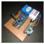
AIR Mouse is also called gesture-controlled mouse and it works based on hand gesture. In this project an accelerometer is used for measuring the tilt of hand in X and Y direction and moves the cursor according to the tilt. In the project two types of..... Listed under: [Battery Projects](#)
