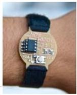
Hello! Welcome to another Other Machine project tutorial! I'm Sam DeRose, a former Other Machine Co. Summer Intern. I created the Nerd Watch last summer while working at OMC. The Nerd Watch displays the time in binary when the button is pushed. The watch shows the..... Listed under: [Clock – Timer Projects](#)
