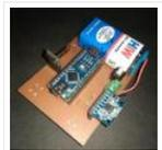
AIR Mouse is also called gesture-controlled mouse and it works based on hand gesture. In this project an accelerometer is used for measuring the tilt of hand in X and Y direction and moves the cursor according the tilt. In the project two types of..... Listed under: [Battery Projects](#)
