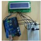
As a simple first Arduino experiment I interfaced a two line LCD (a Displaytech 162B) and an LM35DZ to make a simple Min/Max thermometer. Step 1 – Interfacing the Temperature Sensor This is really very simple. The LM35DZ has three pins, +5V, ground and a..... Listed under: [LCD Projects](#)
