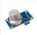
In this guide, we learn how to interface MQ5 Gas sensor (which is a generic Gas Sensor more suited to detect and determine LPG concentrations) with Arduino. In this tutorial, we are using the MQ5 Gas sensor module (which is widely available in market) ..... Listed under: [Sensor – Transducer – Detector Projects](#)
