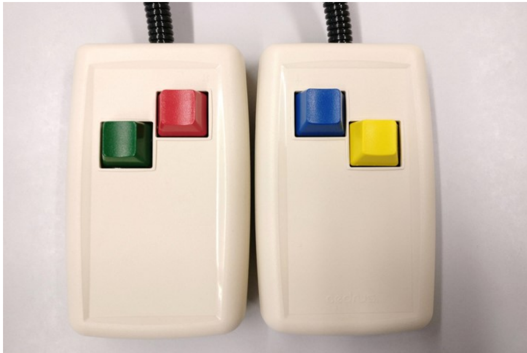
Figure 19.8.: The MRI-safe gamepads used as input device for the VR game.
