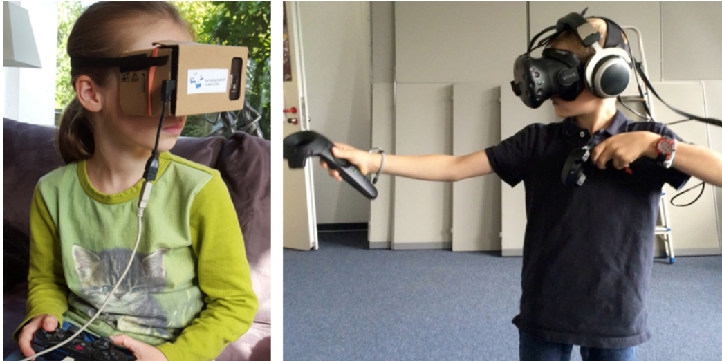
Figure 13.1.: Left: A girl using a customized cardboard mount for a smartphone and a PlayStation 3 controller. The dimensions of the mount are more suitable for small heads. However, this solution suffers from limited ergonomic quality and the high weight of the smartphone. Right: A boy using the HTC Vive HMD and controllers with additional headphones. (Photos © Jasmin Kirchhübel, Maic Masuch )
