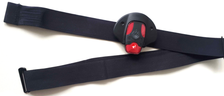
Figure 5.2.: A Bittium Faros 180 HRV sensor with stingray adapter and chest belt. (Photo reproduced by kind permission of Sykownik et al. [Syk+19])
