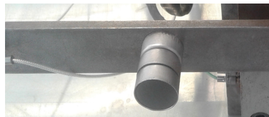
Figure 3.3: Mechanical beam modification using additive mass [ARS20]
